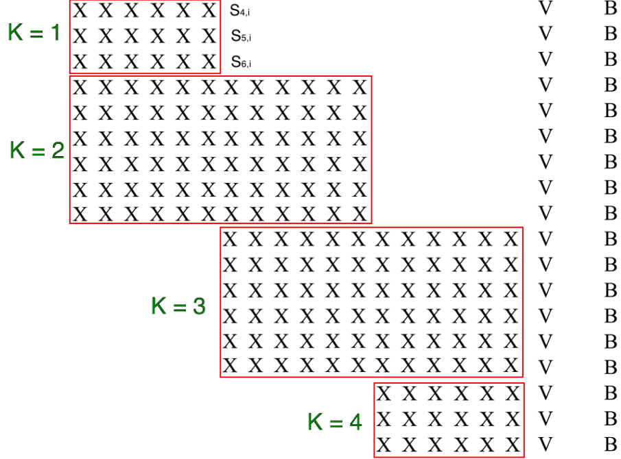
Figure 1: Matrix structure of a set of linear six FDEs with three boundary conditions imposed at both endpoints. One X represents a coefficient of the FDEs, V represents a component of the unknown solution vector, and B is a component of the known right-hand side. Empty spaces represent zeros.
