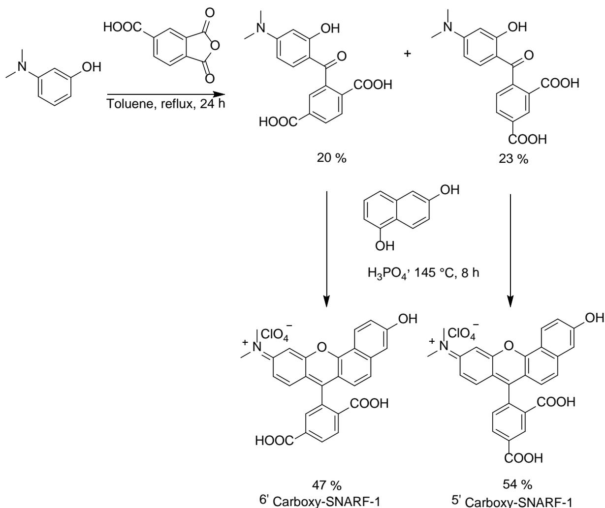
**Scheme S1** Synthesis of the 5' and 6' separated C-SNARF
