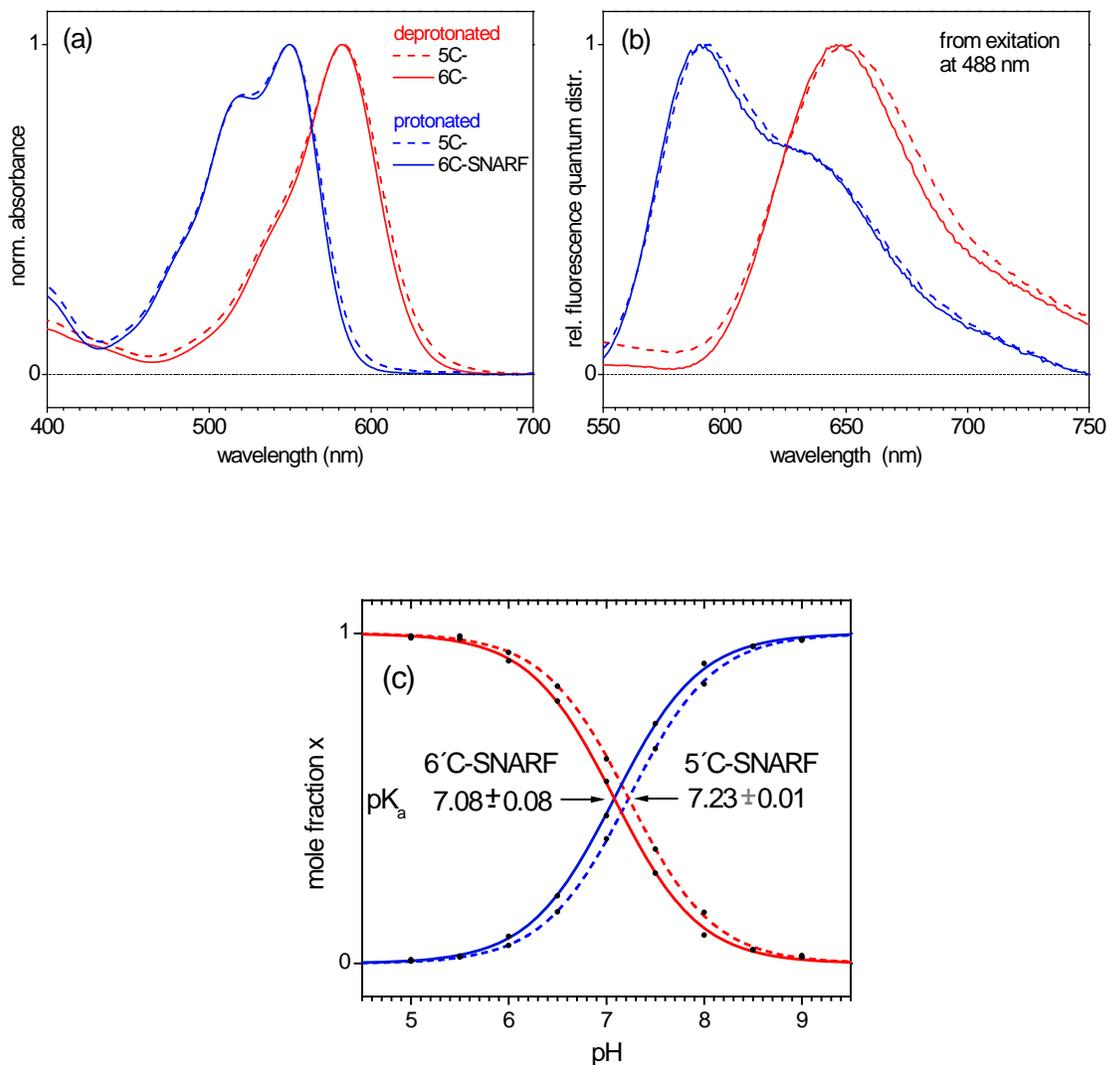
**Figure S3.** Absorption (a) and fluorescence (b) spectra of 5'-C- and 6'-C-SNARF and corresponding titration curves (c), in water:dmsolvent 5:1 (vol:vol) at 22°C. A relatively high concentration of cosolvent was used to avoid solubility problems around pH 5.
