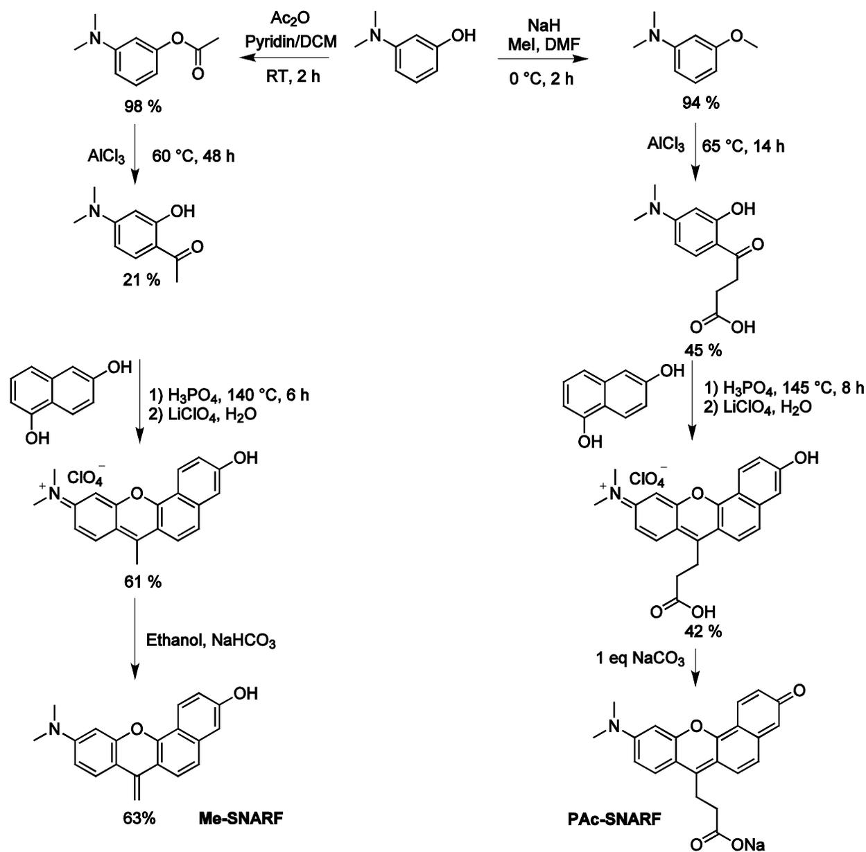
**Scheme S2** Synthesis of Me-SNARF (left branch) and of Pac-SNARF (right).
