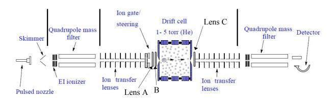
**Figure S1.** Schematic diagram of the mass-selected ion mobility tandem mass spectrometer at VCU.
