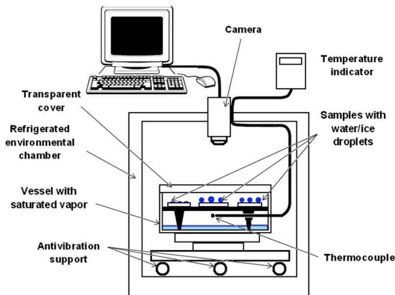
Figure S1. Schematic of the experimental setup for studying the nucleation kinetics.
