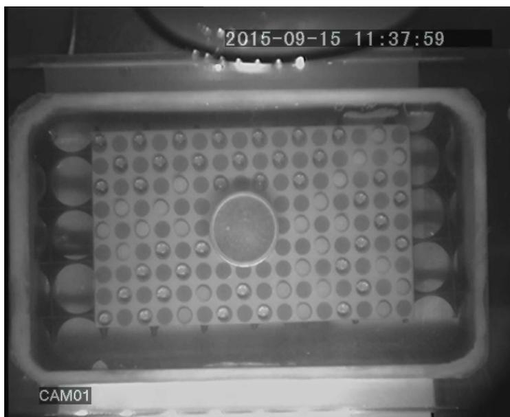
Figure S2. Still image of the experimental cell from the video recorder. A larger disk in the center of the image is the DS1921 temperature sensor. The difference in the appearance of supercooled liquid (bright) and crystallized (gray) droplets is clearly seen.
