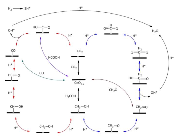
Figure 1 Reaction network for CO<sub>2</sub> hydrogenation on reduced ceria (110)
