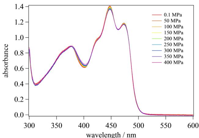
**Figure S-1.** UV-Vis absorption spectra of the phot1LOV2-linker in a buffer solution at various pressures. The pressures are shown in the legend of the figure. The intensity was corrected for the density change.
