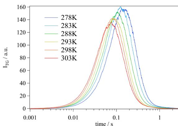
**Figure S-4.** Temperature dependence of the TG signal of the photo1LOV2-linker at ambient pressure measured at  $q^2 = 2.5 \times 10^{11} \text{ m}^{-2}$ .
