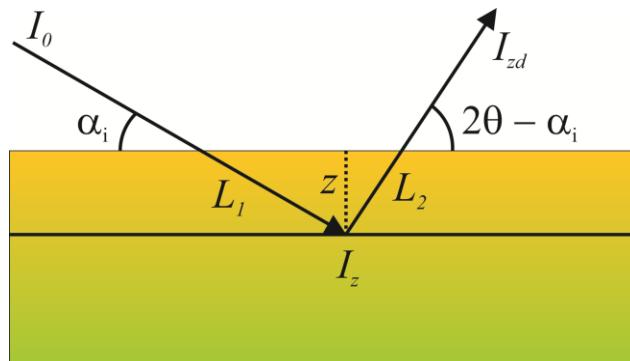
Figure S1. Schematic diagram of the X-ray diffraction through the sample in grazing incidence geometry. Based on the attenuation law, the incident beam  $I_0$  after traveling through the sample and
