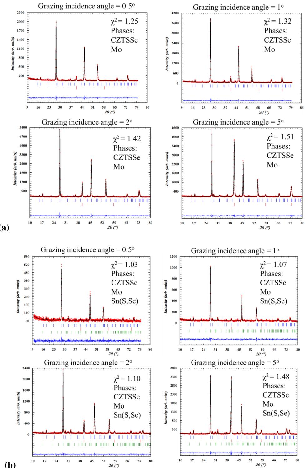
Figure S2. Le Bail fits of the XRD patterns measured with  $0.5^\circ$ ,  $1^\circ$ ,  $2^\circ$  and  $5^\circ$  incidence angles of two representative CZTSSe samples with (a)  $[S] / ([S] + [Se]) = 0.27$  and (b)  $[S] / ([S] + [Se]) = 0.65$  anion compositions.
