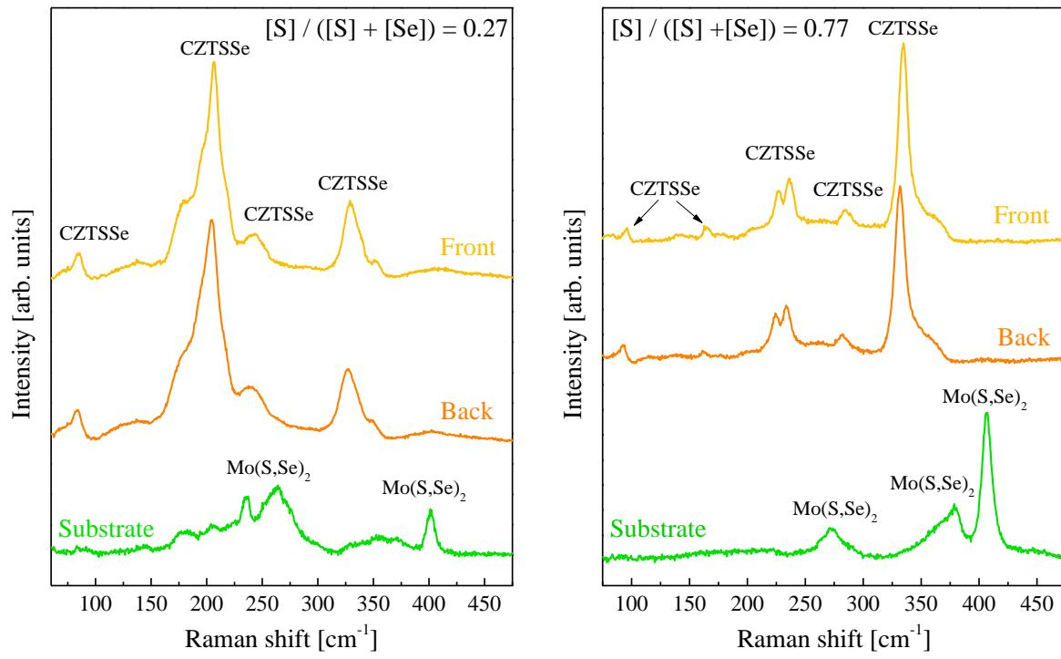
Figure S3. Raman spectra of front, back and substrate for two representative CZTSSe samples measured with 532 nm excitation wavelength.
