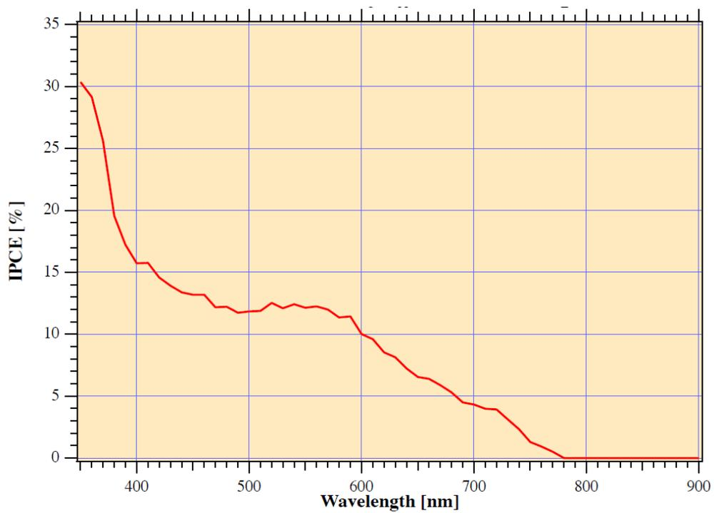
**Figure S76.** IPCE spectrum of M2S/DSSC adsorbed on [10+5]  $\mu\text{m}$  thick  $\text{TiO}_2$  film and using iodine-based electrolyte A.
