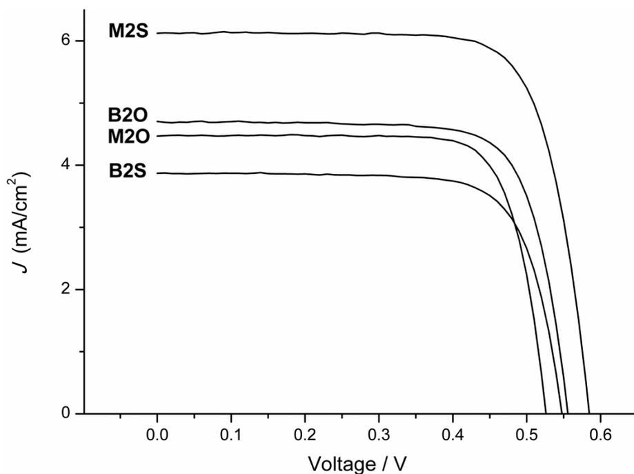
**Figure S74.** I/V curves under one sun illumination (AM1.5G) of the best DSSC devices made with **M2S**, **M2O**, **B2S** and **B2O** ([10+5]  $\mu\text{m}$  thick  $\text{TiO}_2$  films, electrolyte B).
