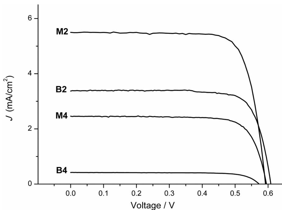
**Figure S73.** I/V curves under one sun illumination (AM1.5G) of the best DSSC devices made with **M2**, **B2**, **M4** and **B4** ([10+5]  $\mu\text{m}$  thick  $\text{TiO}_2$  films, electrolyte A).
