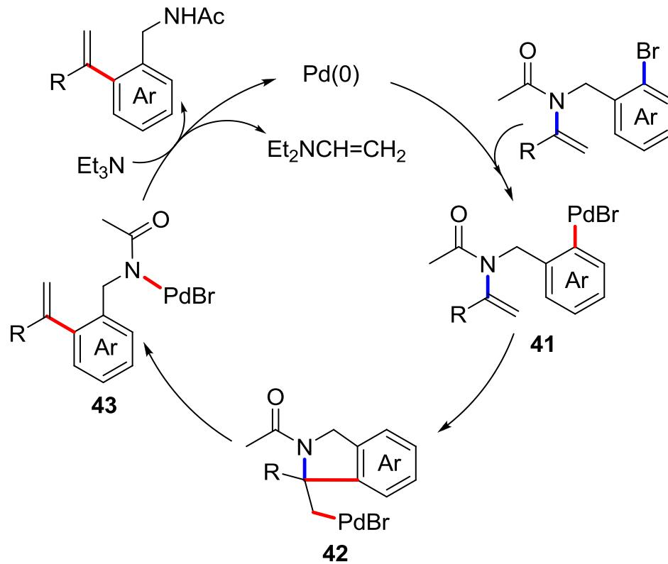
Proposed mechanism for Heck reaction of *N*-vinylacetamide derivatives
