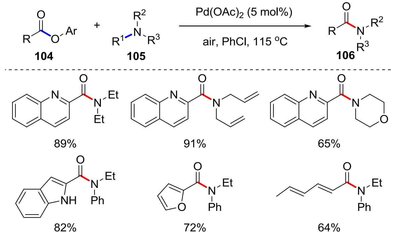
Palladium–catalysed oxidative coupling
