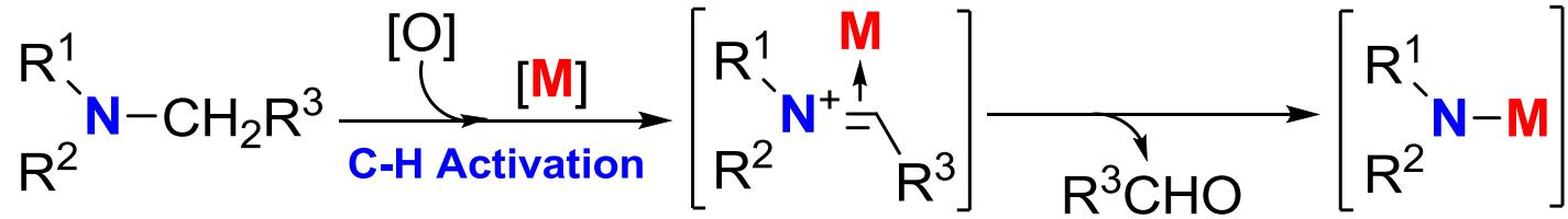
Three general mechanisms for transition-metal - mediated C–N bond metalation
