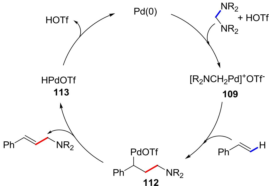
Proposed mechanism for Pd-catalysed vinylation of amines
