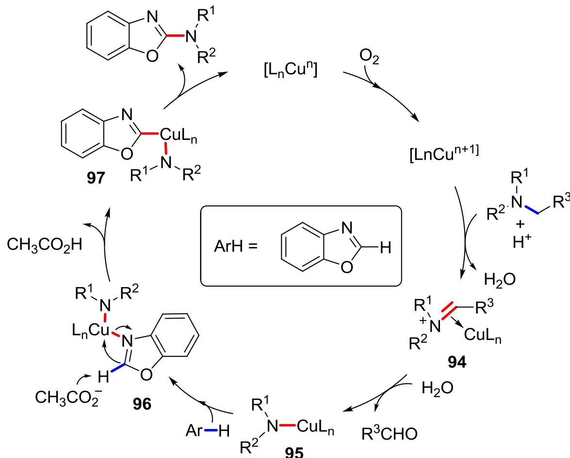
Proposed mechanism for copper-catalysed oxidative amination
