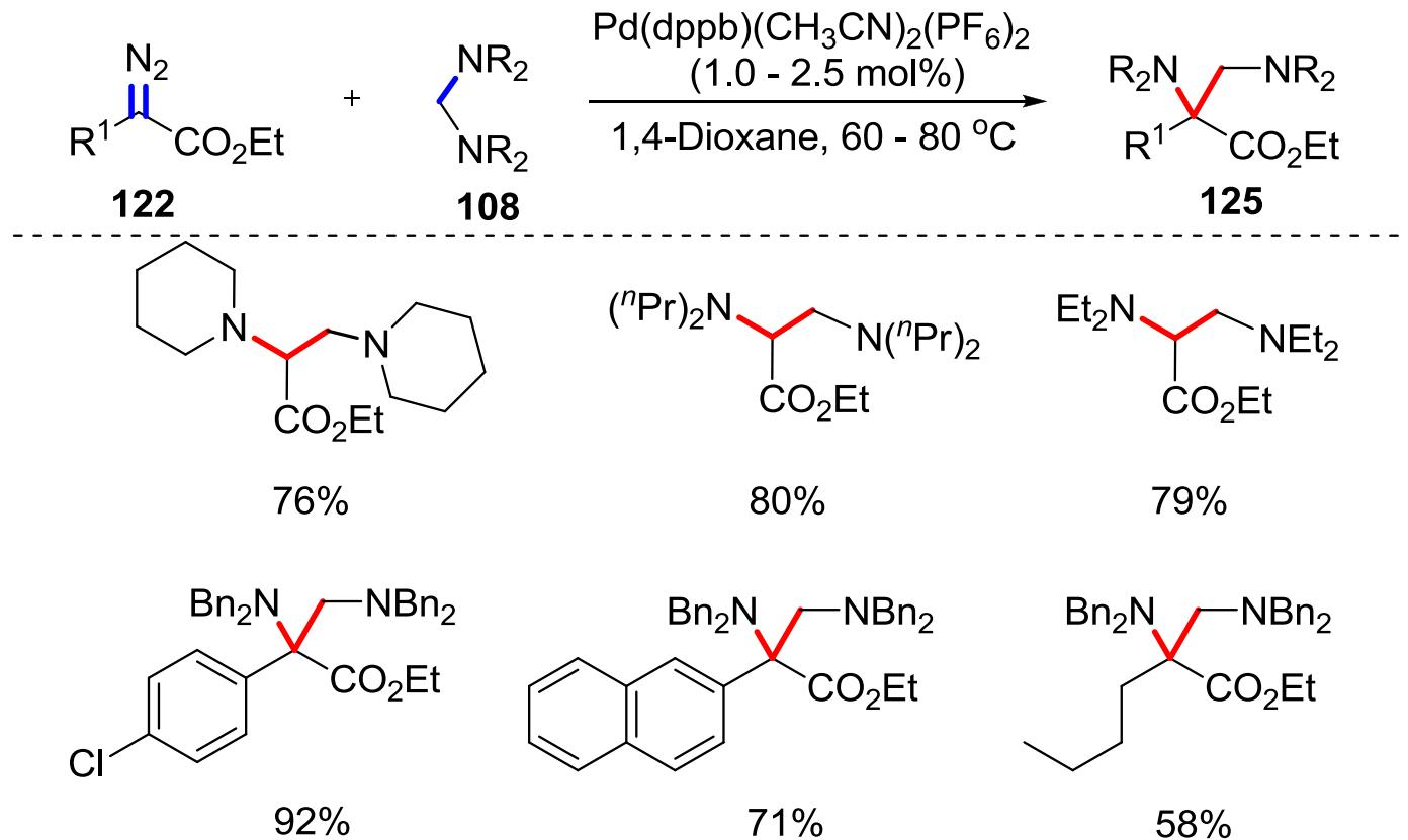
Palladium-catalysed formal insertion of carbenoids into Amines
