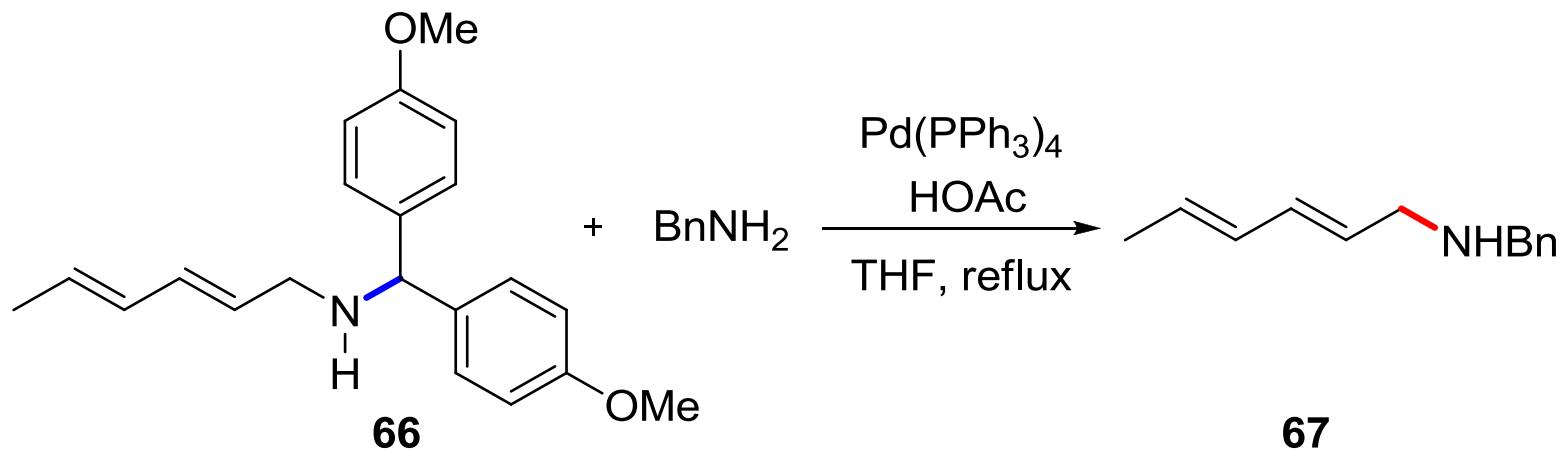
Palladium-catalysed amine exchange reaction of allylic amine
