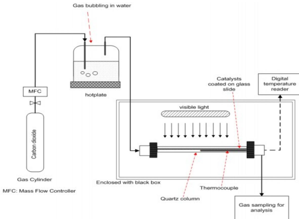
Figure S2. A schematic representation of the gas phase photocatalytic reactor setup
