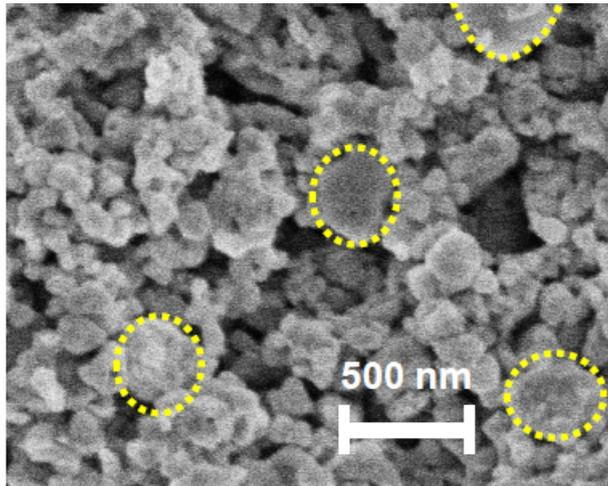
Fig. S8 SEM images of SrTiO<sub>3</sub>:Rh film (WH+20-SS) prepared with a mixture of WH- and SS-particles ( $SS/(WH+SS) = 20$  (wt%)) Yellow dashed line shows the SS-particles.
