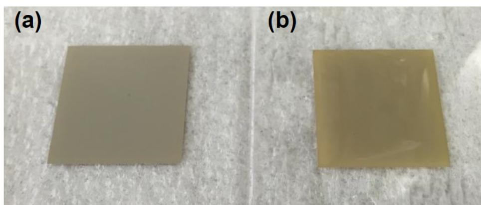
Fig. S5 Picture of WH-10' (a) before and (b) after photocatalytic reaction.
