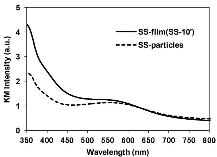
Fig. S4 UV-vis spectra of SrTiO<sub>3</sub>:Rh films (SS-10') and SrTiO<sub>3</sub>:Rh particles (SS-particles).
