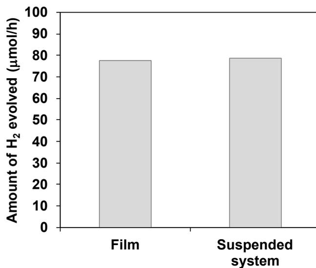
Fig.S7 Rate of H<sub>2</sub> evolution from an aqueous methanol solution under visible light irradiation on a SrTiO<sub>3</sub> film and from a SrTiO<sub>3</sub>-suspended system containing SrTiO<sub>3</sub> particles with the same amount as the film contains.
