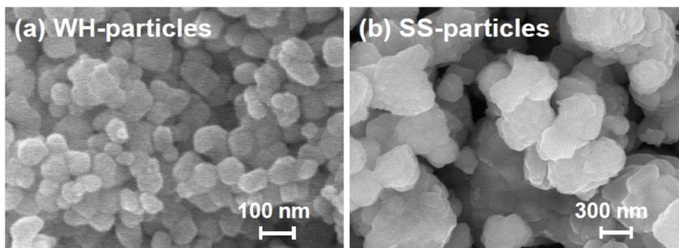
Fig. S3 SEM images of SrTiO<sub>3</sub>:Rh particles ((a) WH-particles, (b) SS-particles)).
