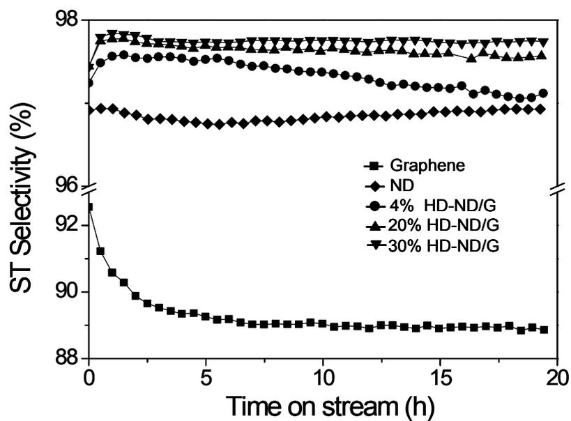
**Fig. S6** Catalytic performance over few-layer graphene, HD-ND/graphene catalysts with different ND weight loading (4 wt%, 12 wt%, 30 wt%) and commercial ND powders. Reaction conditions: T = 550 °C, Flow rate = 10 ml min<sup>-1</sup>, 2.6% ethylbenzene with He balance.
