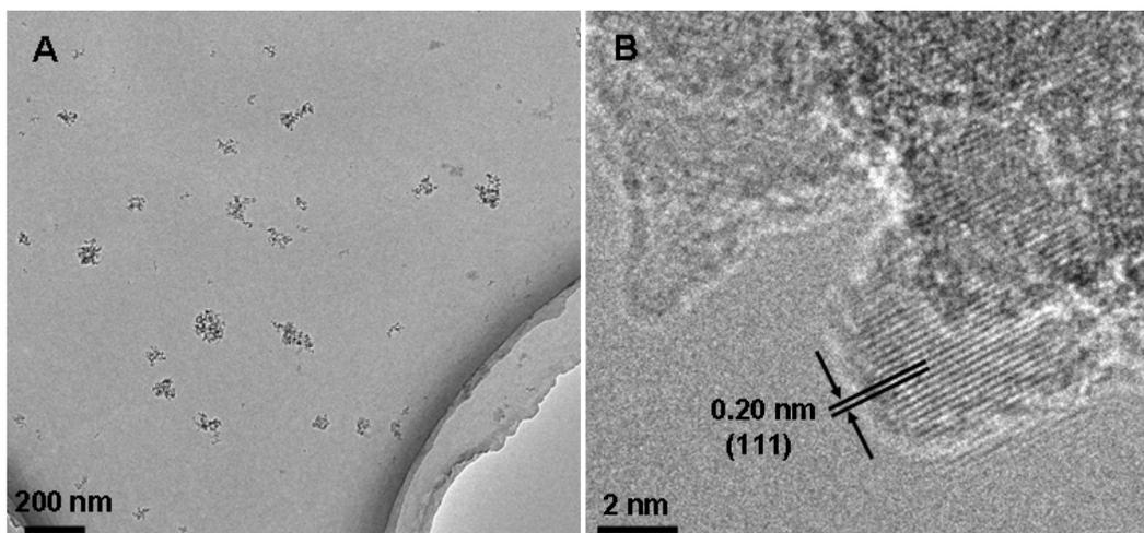
**Fig. S1** TEM images of the (A) commercial ND aggregates collected after sonicating in water and the HRTEM image of (B) one single HD-ND nanoparticle.
