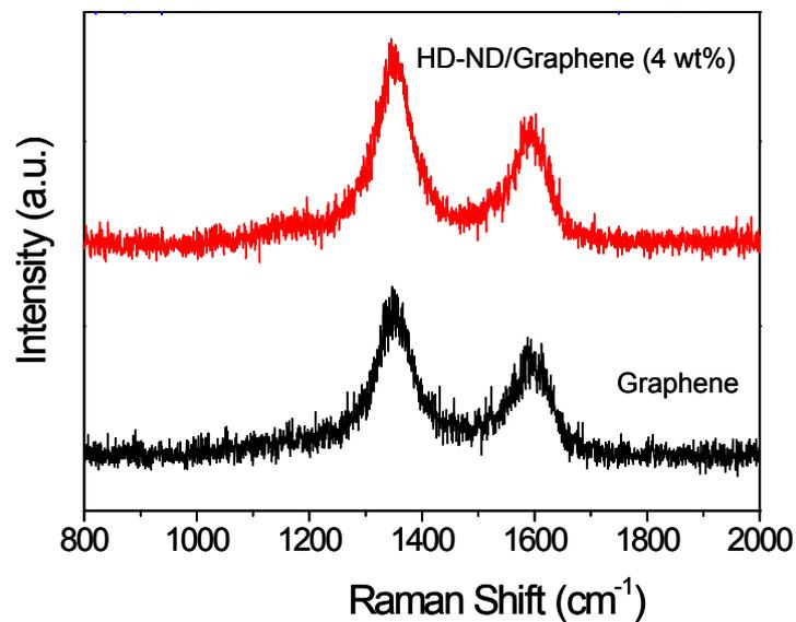
**Fig. S5** Raman spectra of the graphene support and HD-ND/graphene (4 wt%) catalyst.
