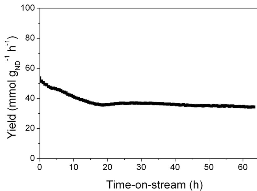
**Fig. S7** The long term test over the HD-ND/graphene catalysts with 4% ND weight loading. Reaction conditions: T = 550 °C, Flow rate = 10 ml min<sup>-1</sup>, 2.6% ethylbenzene with He balance.
