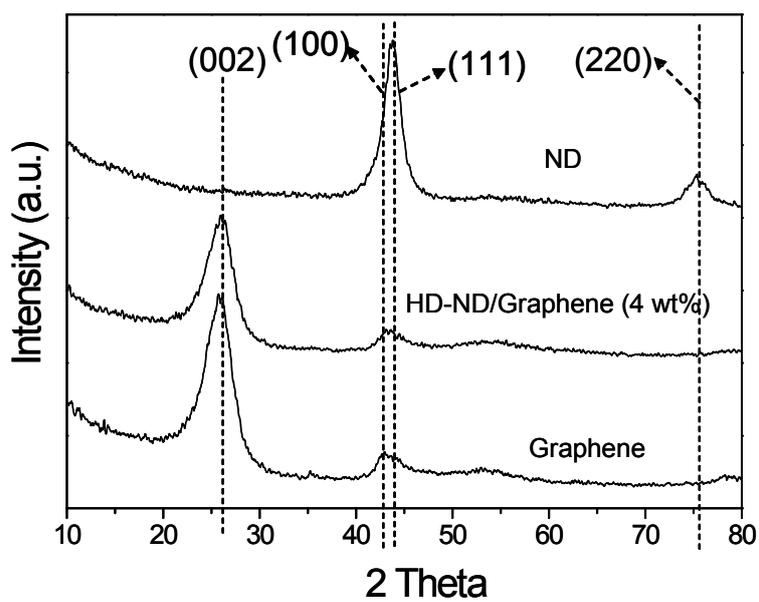
**Fig. S4** XRD patterns of the commercial ND powders, HD-ND/graphene (4 wt%) and the pure graphene support.
