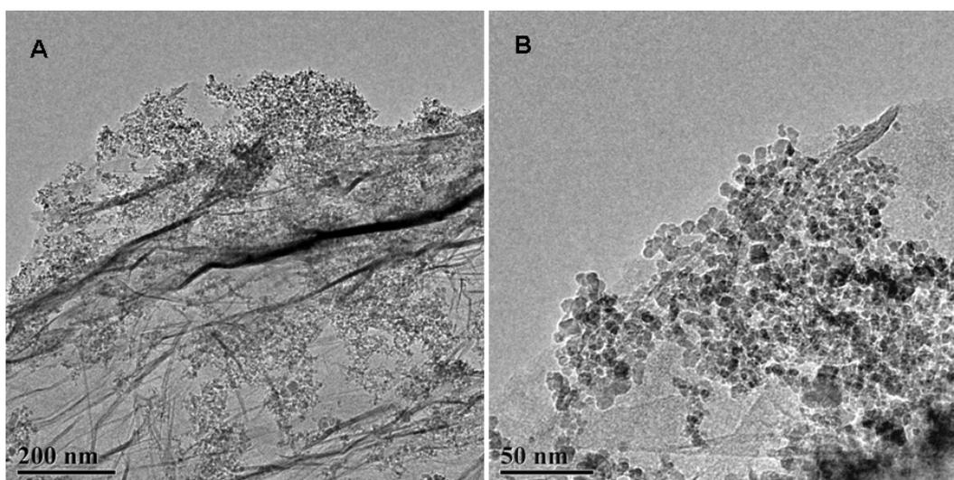
**Fig. S2** TEM images of the HD-ND/graphene catalyst. The weight loading of ND is 12 wt%.
