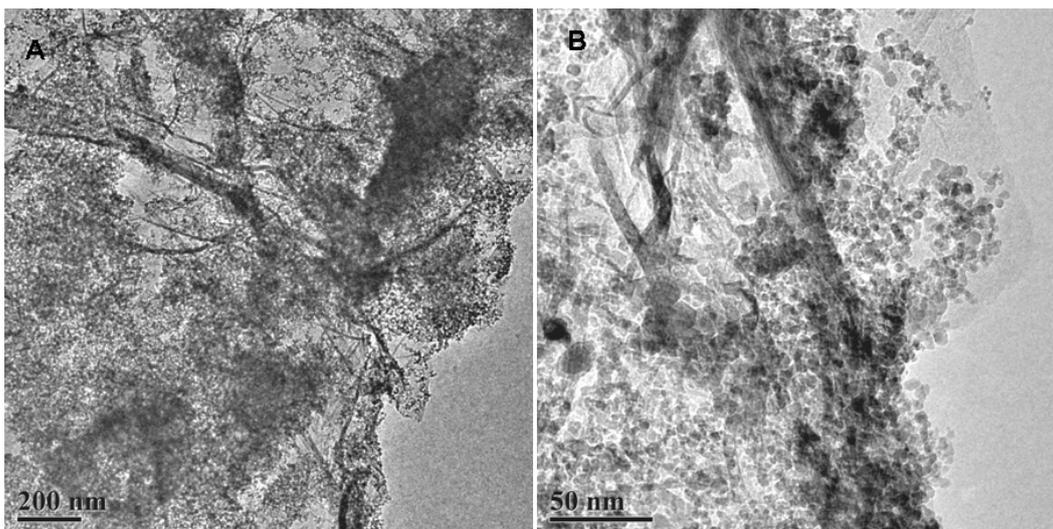
**Fig. S3** TEM images of the HD-ND/graphene catalyst. The weight loading of ND is 30 wt%.
