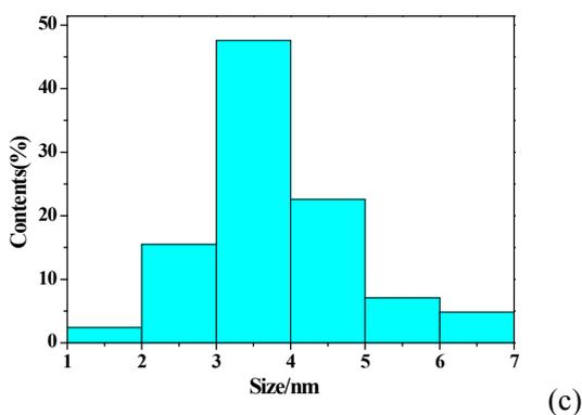
**Fig. S2** (a) TEM image of used Au/h-Co<sub>3</sub>O<sub>4</sub>, (b) Au particle size distribution of used Au/h-Co<sub>3</sub>O<sub>4</sub> ( $3.5 \pm 0.8$  nm), and (c) Au particle size distribution of used Au/c-Co<sub>3</sub>O<sub>4</sub> ( $3.9 \pm 1.2$  nm).
