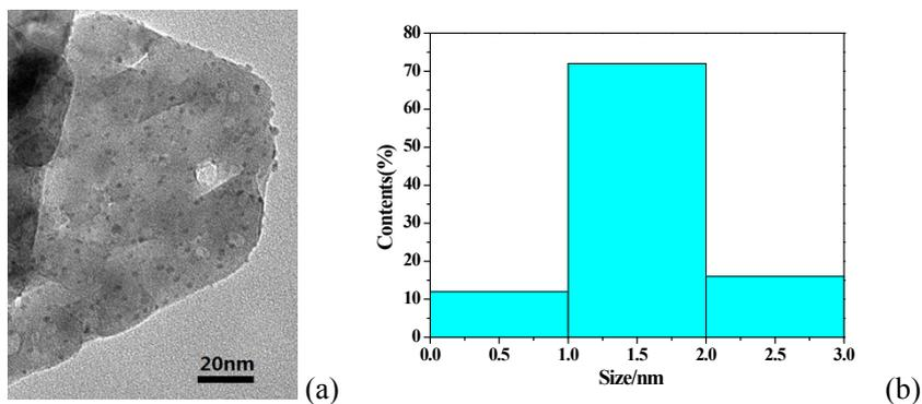
**Fig. S1** (a) TEM image and (b) Au particle size distribution of s-Au/h-Co<sub>3</sub>O<sub>4</sub> ( $1.6 \pm 0.6$  nm).
