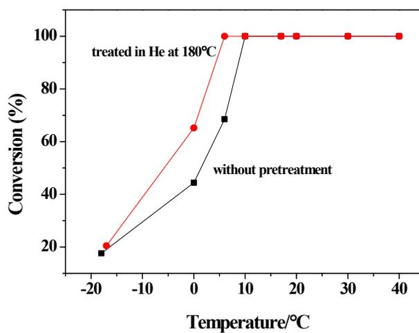
**Fig. S4** Temperature dependence of CO conversions over *s*-Au/*h*-Co<sub>3</sub>O<sub>4</sub> (1.6 ± 0.6 nm) without and with He-pretreatment.
