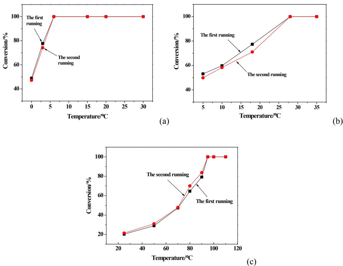
**Fig. S5** Activity repeatability tests over (a) *s*-Au/*h*-Co<sub>3</sub>O<sub>4</sub>, (b) Au/*h*-Co<sub>3</sub>O<sub>4</sub>, and (c) Au/*t*-Co<sub>3</sub>O<sub>4</sub>. The fresh samples were pretreated in the reaction atmosphere.
