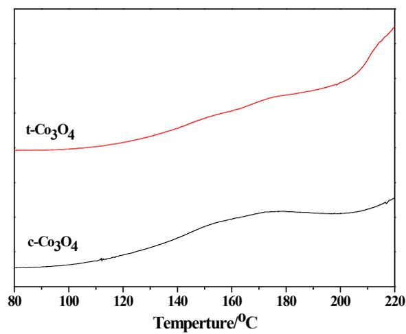
**Fig. S3** H<sub>2</sub>-TPR profiles of *c*-Co<sub>3</sub>O<sub>4</sub> and *t*-Co<sub>3</sub>O<sub>4</sub> in the 80-220°C range.
