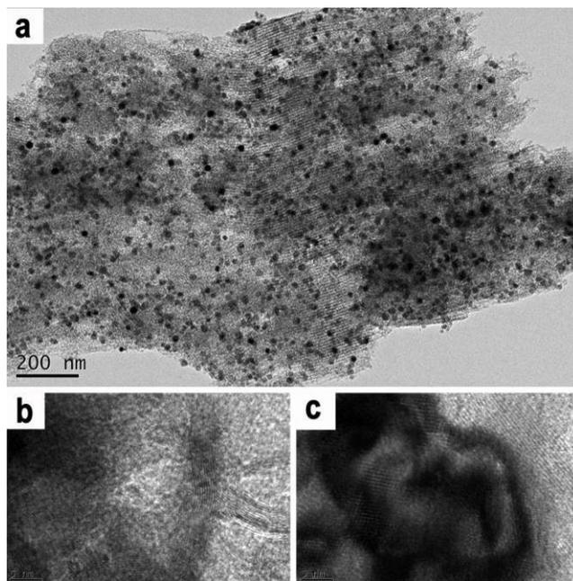
**Fig. S-1** TEM of Pd/NZVI@P (a), HR-TEM Pd/NZVI@P (b and c).
