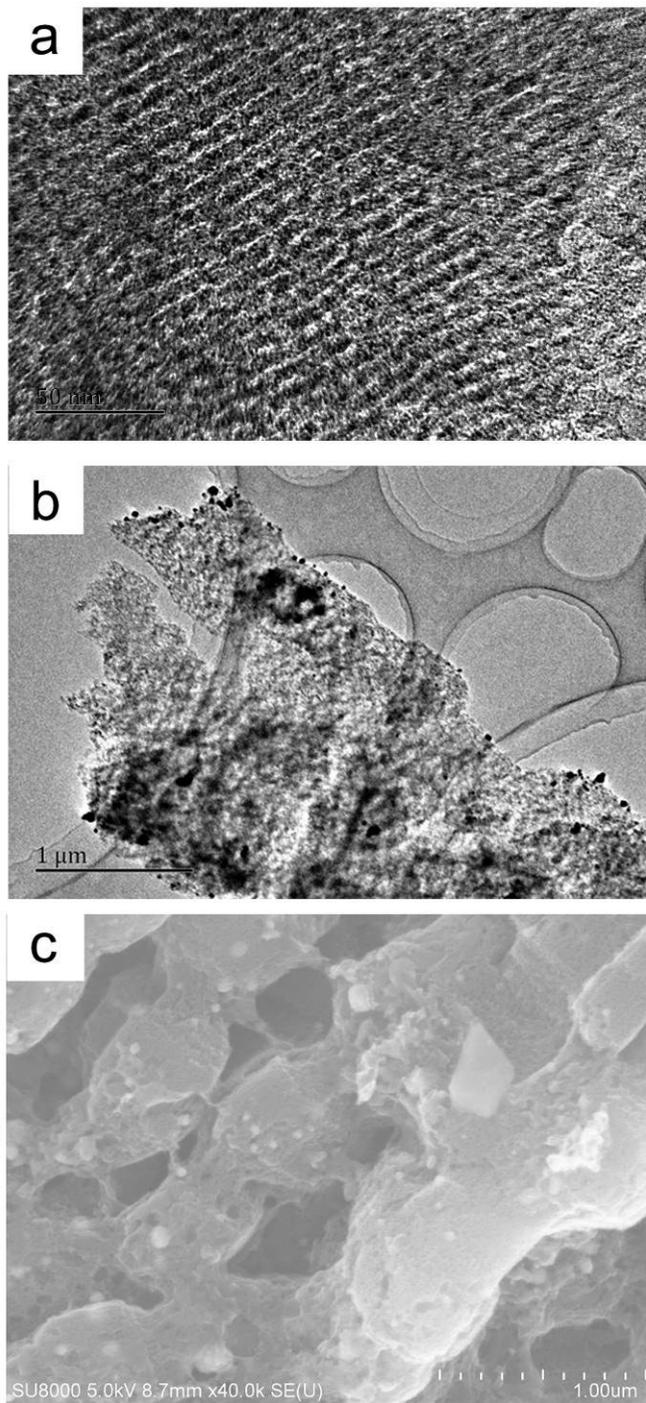
**Fig. S-2** TEM of OMC (a), Pd/NZVI/OMC (b), and SEM of Pd/NZVI/OMC (c).
