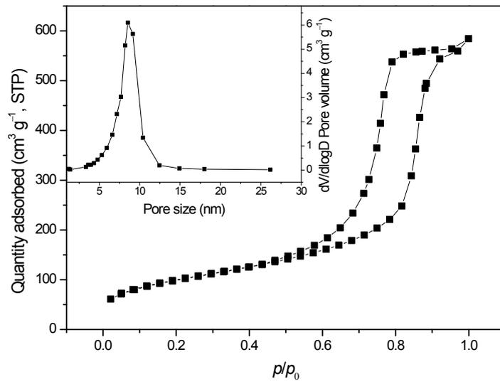
**Fig. S1** N<sub>2</sub> adsorption–desorption isotherms and the pore size distribution (the inset) of FDU-12.
