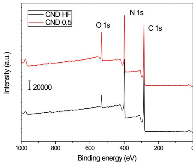
**Fig. S2** XPS surveys of CND-HF and CND-0.5M.
