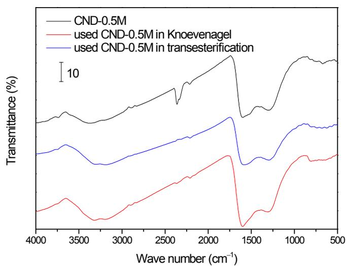
**Fig. S4** FT-IR spectra of the fresh and spent CND-0.5M catalysts subjected to four runs in Knoevenagel condensation and transesterification reactions.
