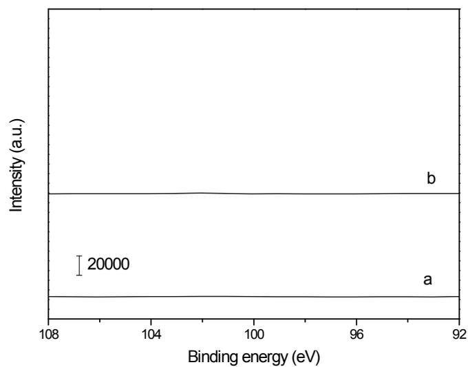
**Fig. S3** Si 2p region of XPS surveys of CND-HF (a) and CND-0.5M (b).
