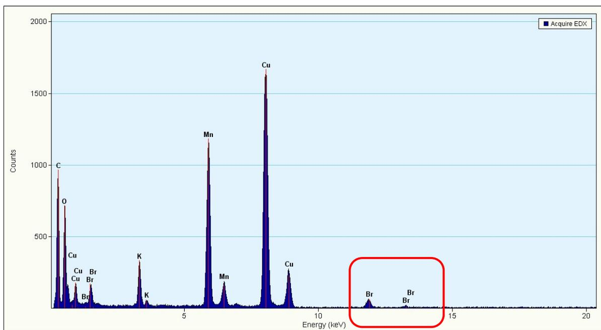
**Figure S13.** TEM-EDX (based on Figure 10c) of the sample i.e. manganese oxide, which was prepared by the addition of excess KBr solution in  $\text{KMnO}_4$  + CTAB solution (calined at  $500\text{ }^\circ\text{C}/3\text{h}$ )
