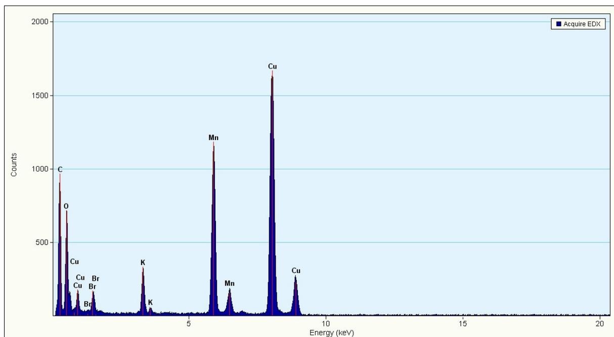
**Figure S14.** TEM-EDX (based on Figure 10c) of the sample i.e. manganese oxide, which was prepared by the addition of excess KBr solution in  $\text{KMnO}_4$  + CTAB solution (calined at  $500\text{ }^\circ\text{C}/6\text{h}$ )
