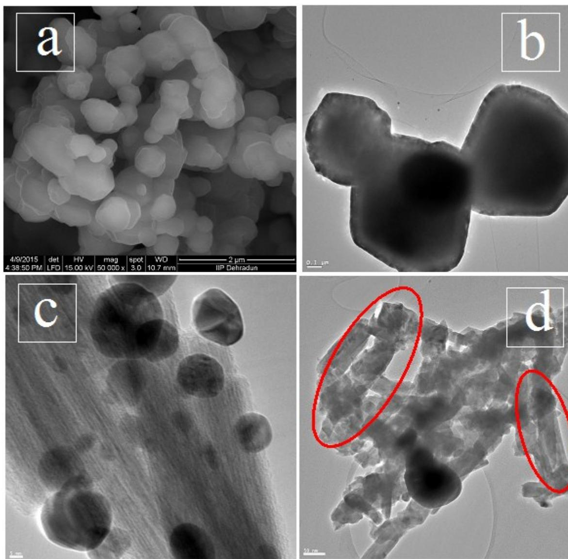
**Figure S9.** TEM images of the samples with Ag-loadings (a) 0 %, (b) 1.6 % (c) 15.5% and (d) 27%.
