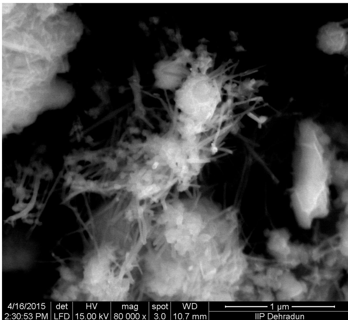
**Figure S10.** SEM images of the Ag-Mn sample when nitrate precursors of Ag and Mn and cetyl alcohol was used as surfactant.
