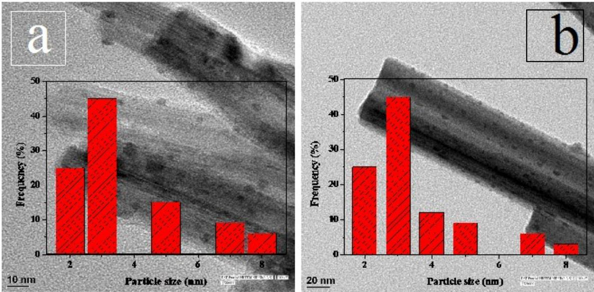
**Figure S3.** Particle size distributions (histogram) of (a) fresh catalyst (based on Fig. 6b and that of (b) spent catalyst (based on Fig. 6d).
