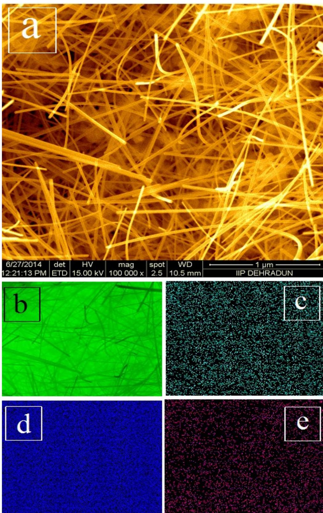
**Figure S2.** (a) SEM image (repeat of Fig. 4a, Main), (b) SEM-elemental mapping and SEM-elemental mapping of (c) Ag, (d) O and (e) Mn.
