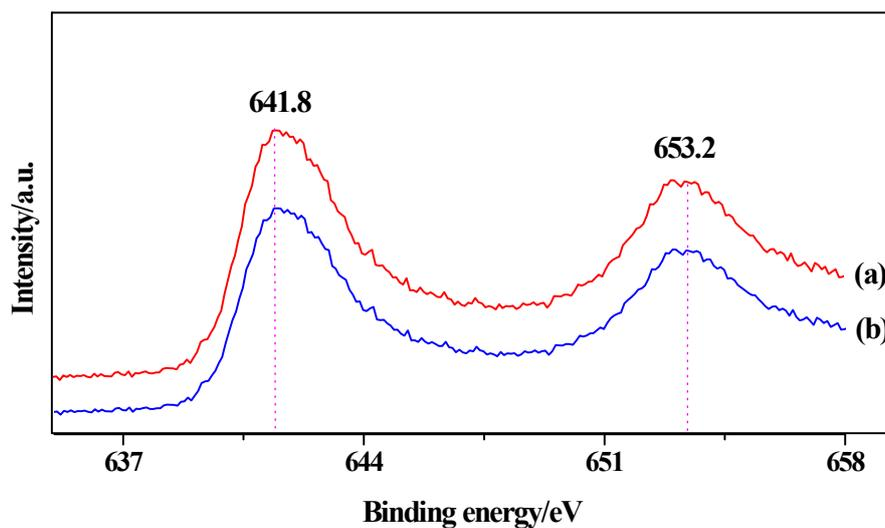
**Figure S1.** Mn 2p core-level spectra (XPS) of (a) fresh and (b) spent Ag-Mn nano-rod catalyst.
