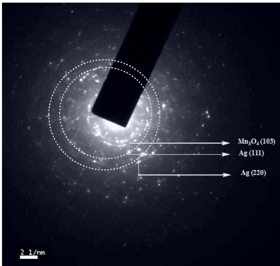
**Figure S4.** The electron diffraction pattern (based on Fig. 6b, Main).
