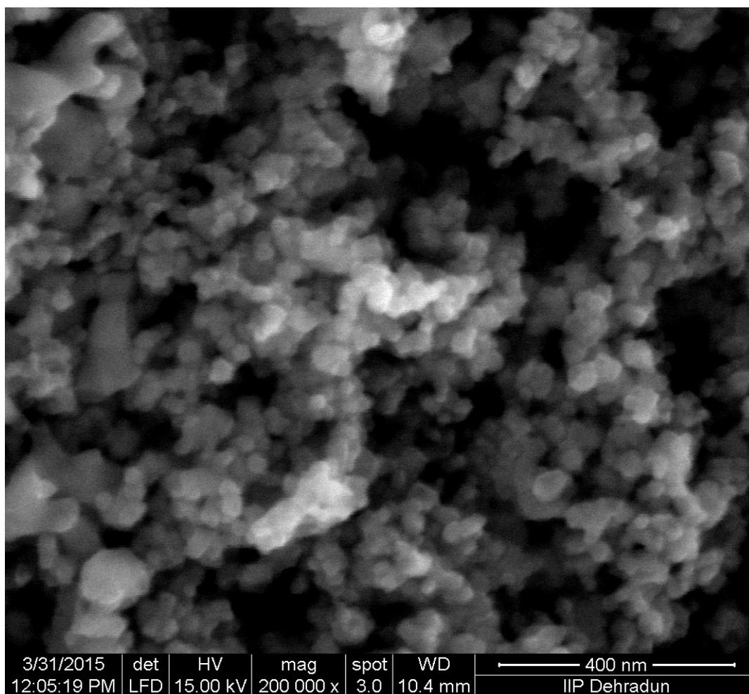
**Figure S12.** SEM image of the sample taking  $\text{KMnO}_4$  as the precursor of Mn and avoided the addition of any Ag-species and the other reagents were added as before.
