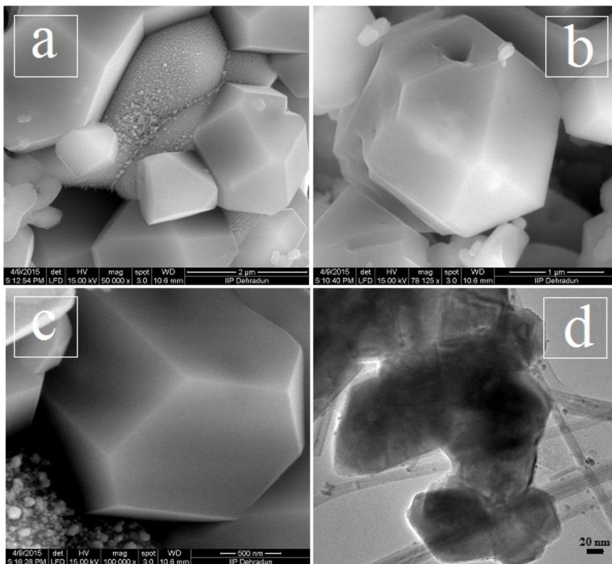
**Figure S8.** (a-c) SEM and (d) TEM images of the Ag-Mn sample when the aging time prolonged to 24h.
