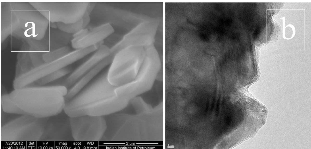
**Figure S15.** (a) SEM and (b) TEM images of the Ag-Mn sample when  $\text{KMnO}_4$  was used as the precursor of Mn.
