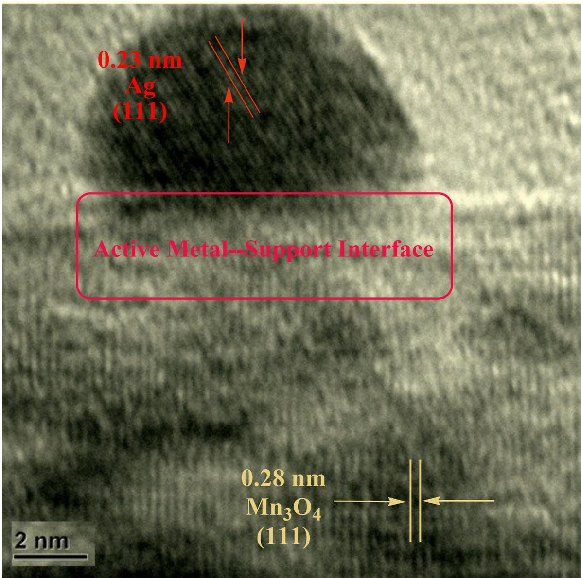
**Figure S16.** TEM image of the 1D Ag/Mn<sub>3</sub>O<sub>4</sub> catalyst (HRTEM) to show the Ag-Mn interface.
