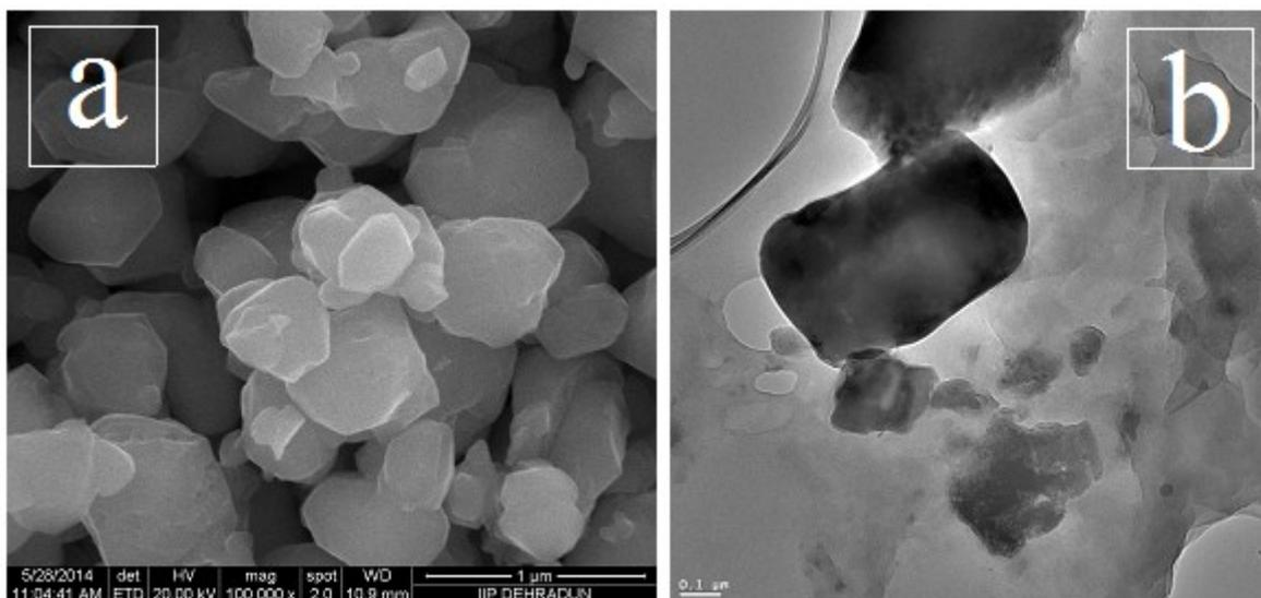
**Figure S5.** (a) SEM and (b) TEM image of the Ag-Mn catalyst without using the surfactant CTAB.
