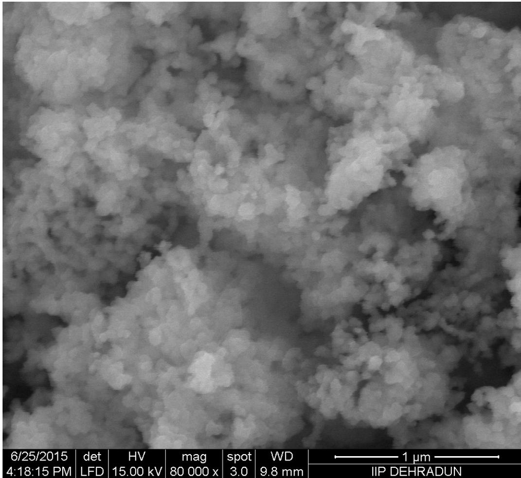
**Figure S11.** SEM images of the Ag-Mn sample when nitrate precursors of Ag and Mn and sodium dodecylsulfate (SDS) was used as surfactant.
