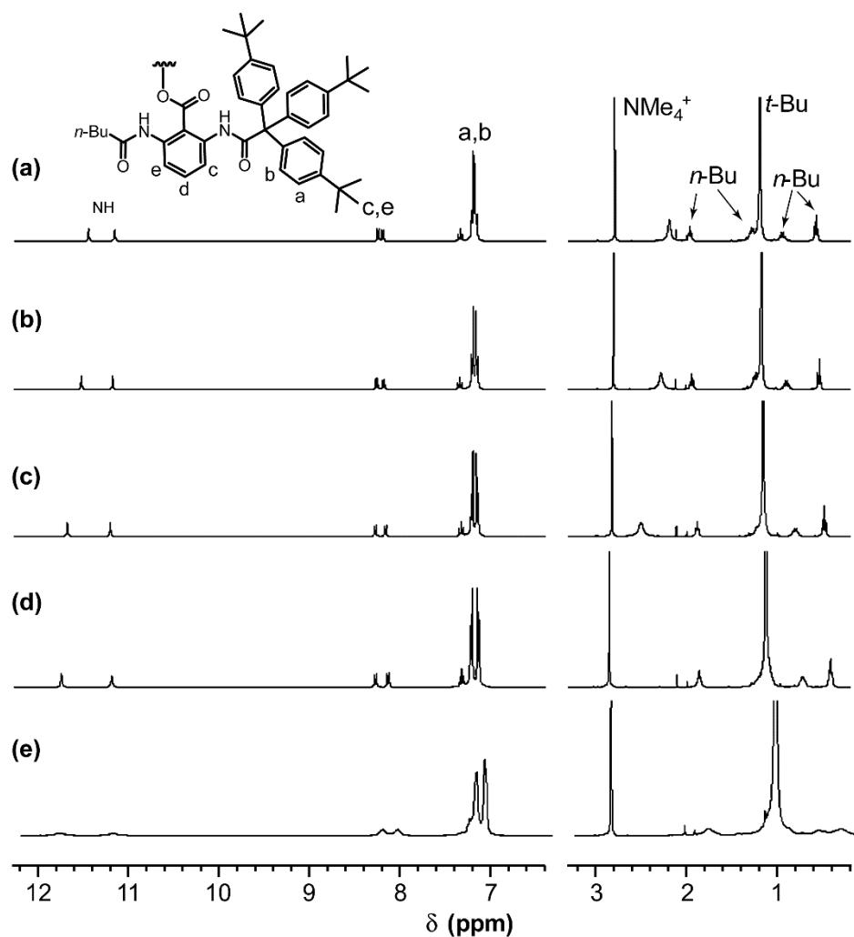
**Fig. S7**  $^1\text{H}$  NMR spectra of  $(\text{NMe}_4)[\text{ZnL13}]$  in  $\text{CD}_2\text{Cl}_2$  at (a)  $30^\circ\text{C}$ , (b)  $0^\circ\text{C}$ , (c)  $-30^\circ\text{C}$ ,  $-60^\circ\text{C}$ , and  $-90^\circ\text{C}$ .
