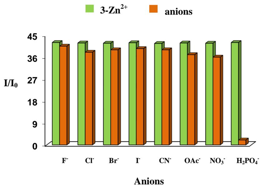
**Figure S19.** Fluorescence response of 3-Zn<sup>2+</sup> towards various anions (60 equiv) in CH<sub>3</sub>CN/H<sub>2</sub>O (8:2, v/v);  $\lambda_{\text{ex}} = 380$  nm. Bars represent the emission intensity ratio ( $I/I_0$ ) ( $I_0$  = initial fluorescence intensity at 445 nm;  $I$  = final fluorescence intensity at 445 nm after the addition of anions).
