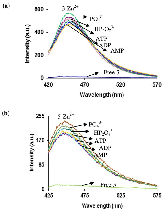
**Figure S21. (a/b):** Fluorescence emission spectra of **3/5-Zn<sup>2+</sup>** complex towards other different phosphate anions: PO<sub>4</sub><sup>3-</sup>, HP<sub>2</sub>O<sub>7</sub><sup>3-</sup>, AMP, ADP, ATP (60/40 equivalent each) in CH<sub>3</sub>CN:H<sub>2</sub>O (8:2, v/v) buffered with HEPES, pH = 7.0; λ<sub>ex</sub> = 380 nm.
