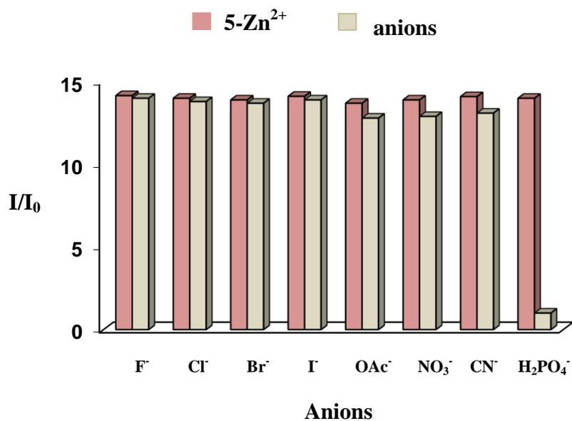
**Figure S20.** Fluorescence response of 5-Zn<sup>2+</sup> towards various anions (40 equiv) in CH<sub>3</sub>CN/H<sub>2</sub>O (8:2, v/v);  $\lambda_{\text{ex}} = 380 \text{ nm}$ . Bars represent the emission intensity ratio ( $I/I_0$ ) ( $I_0$  = initial fluorescence intensity at 445 nm;  $I$  = final fluorescence intensity at 445 nm after the addition of anions).
