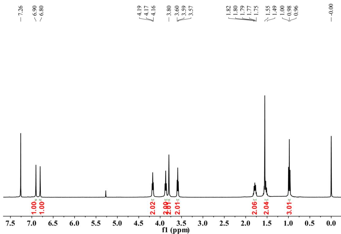
Fig. S3  $^1\text{H}$  NMR spectrum (400 MHz,  $\text{CDCl}_3$ ) of **4a** at 298 K.
