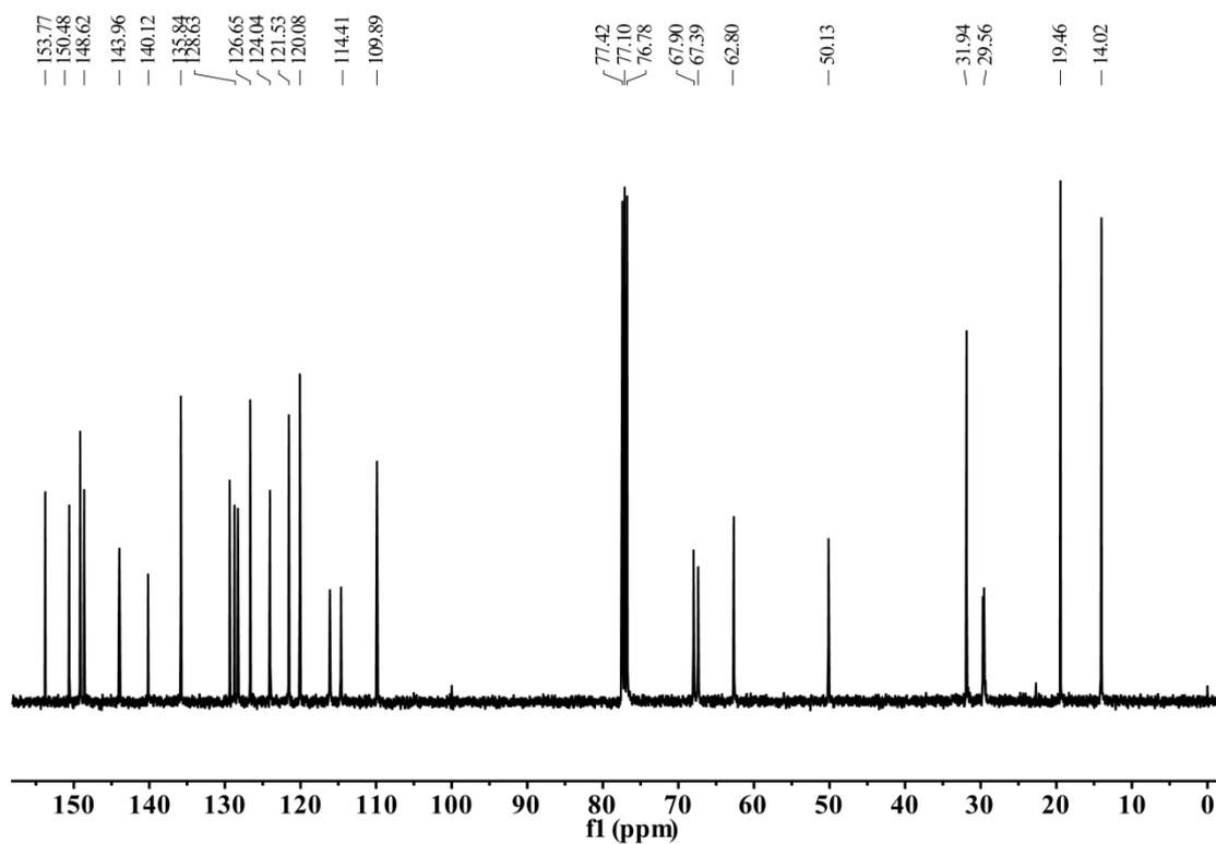
Fig. S10  $^{13}\text{C}$  NMR spectrum (100 MHz,  $\text{CDCl}_3$ ) of **1** at 298 K.
