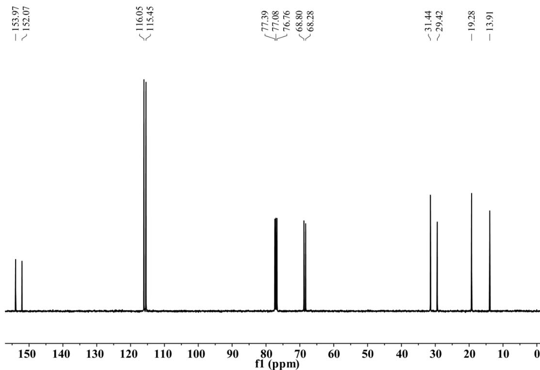
Fig. S2  $^{13}\text{C}$  NMR spectrum (100 MHz,  $\text{CDCl}_3$ ) of **3** at 298 K.
