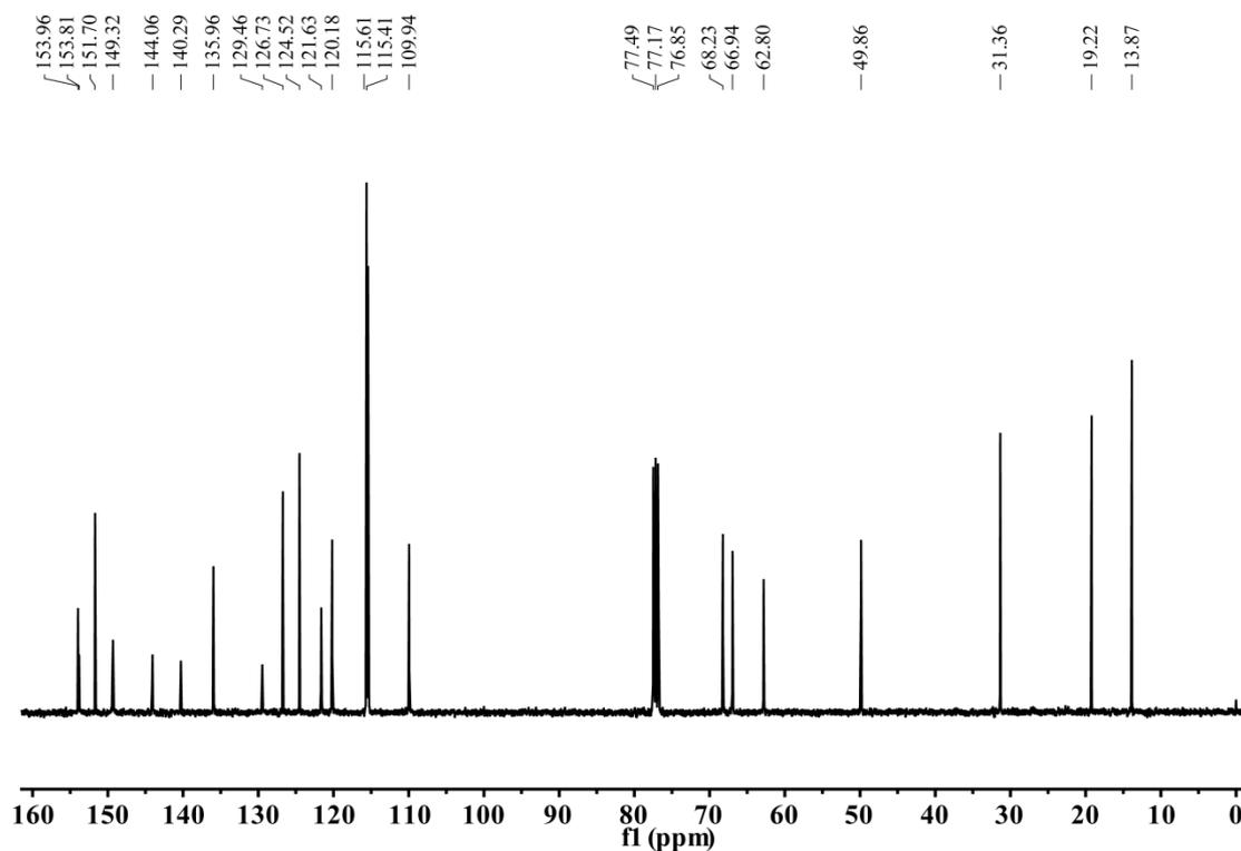
Fig. S13  $^{13}\text{C}$  NMR spectrum (100 MHz,  $\text{CDCl}_3$ ) of **2** at 298 K.
