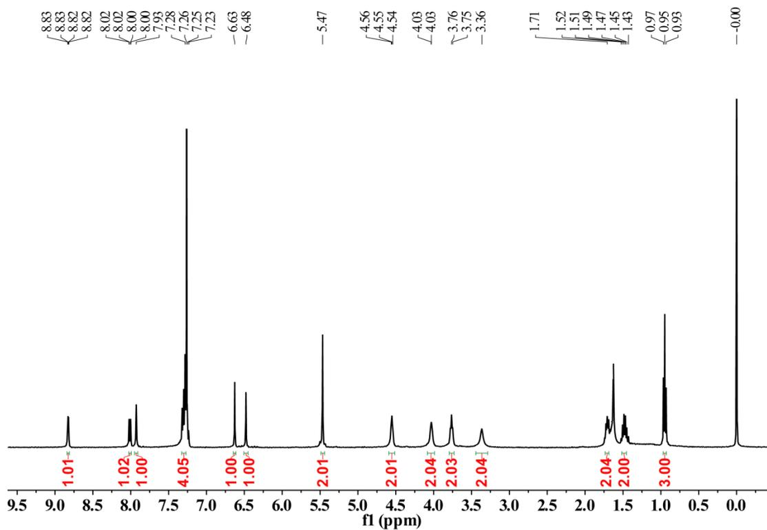
Fig. S9  $^1\text{H}$  NMR spectrum (400 MHz,  $\text{CDCl}_3$ ) of **1** at 298 K.
