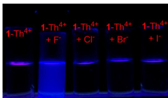
**Fig. S27** Visual changes of **1**-Th<sup>4+</sup> ensemble (50  $\mu$ M) upon addition of 6.0 equiv. of different halides upon excitation at 365 nm using a UV lamp.
