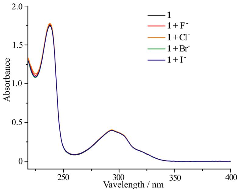
**Fig. S25** Absorption spectra of **1** ( $10 \mu\text{M}$ ) in the presence of different anion species (10 equiv.) in a mixed aqueous medium ( $\text{CH}_3\text{CN-H}_2\text{O}$ ,  $v/v = 9:1$ ).
