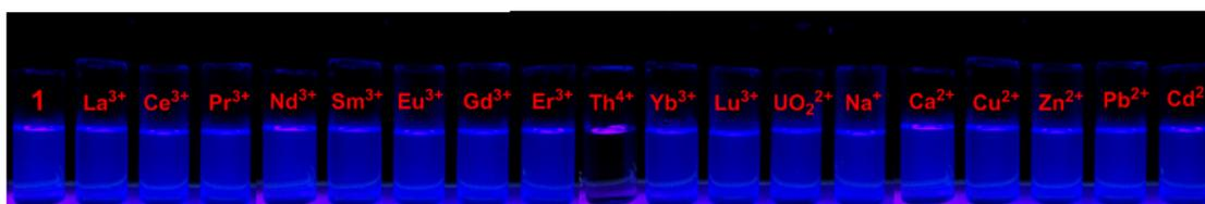
**Fig. S18** Visual changes of **1** (50  $\mu\text{M}$ ) upon addition of 1.0 equiv. of different metal ions upon excitation at 365 nm using a UV lamp.
