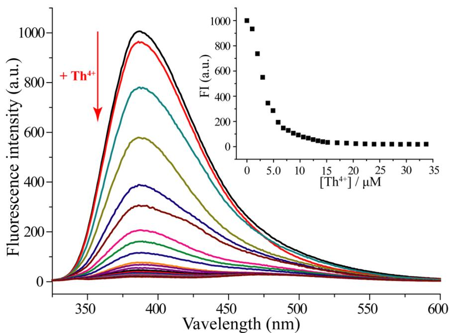
**Fig. S21** Fluorescence titration of **1** with  $\text{Th}^{4+}$  in a mixed aqueous medium ( $\text{CH}_3\text{CN-H}_2\text{O}$ , v/v = 9:1;  $\lambda_{\text{ex}} = 310 \text{ nm}$ ). Inset: fluorescence intensity at 390 nm as a function of  $\text{Th}^{4+}$  concentration.
