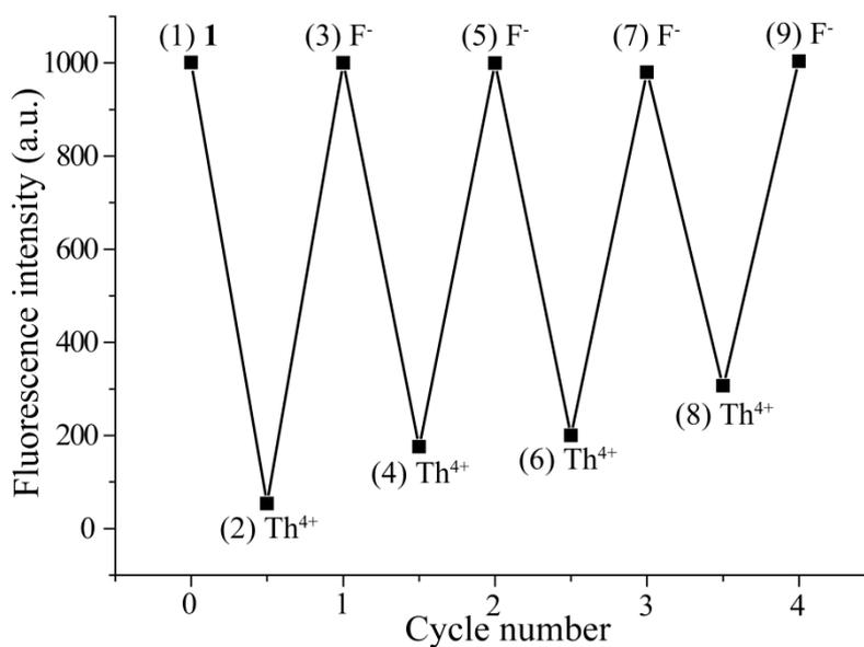
**Fig. S31** Fluorescence intensity changes of **1** (10 μM) at 390 nm in a mixed aqueous medium (CH<sub>3</sub>CN-H<sub>2</sub>O, v/v = 9:1; λ<sub>ex</sub> = 310 nm) as a function of cycles upon alternate addition of Th<sup>4+</sup> and F<sup>-</sup>, where (1) = **1**; (2) = **1** + Th<sup>4+</sup>; (3) = (2) + F<sup>-</sup>; (4) = (3) + Th<sup>4+</sup>;
