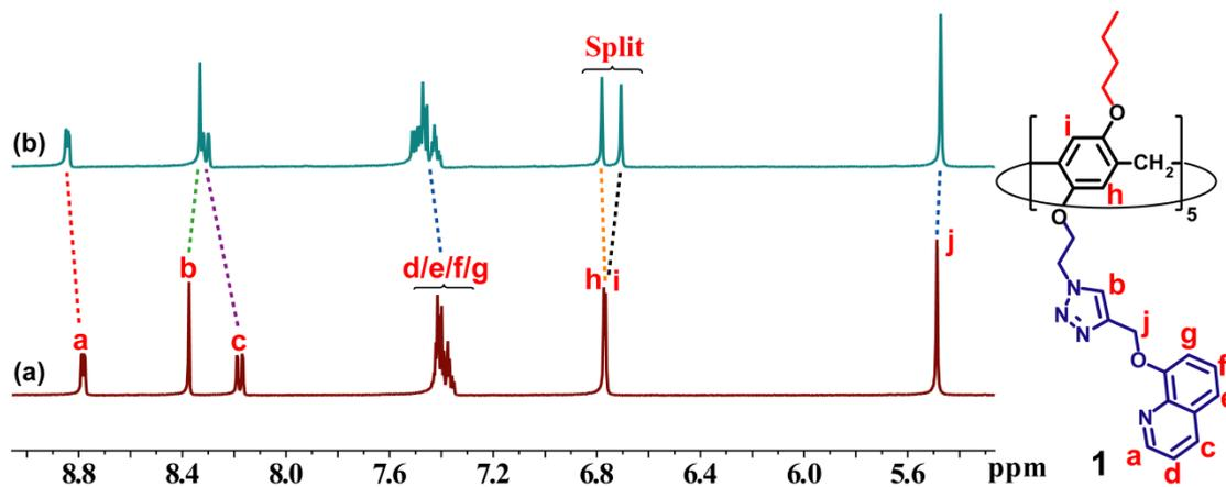
**Fig. S16** Stacked partial  $^1\text{H}$  NMR spectra in acetone- $d_6$ : (a) **1** (2 mM); (b) **1** +  $\text{Th}^{4+}$  (1:1, 2 mM).
