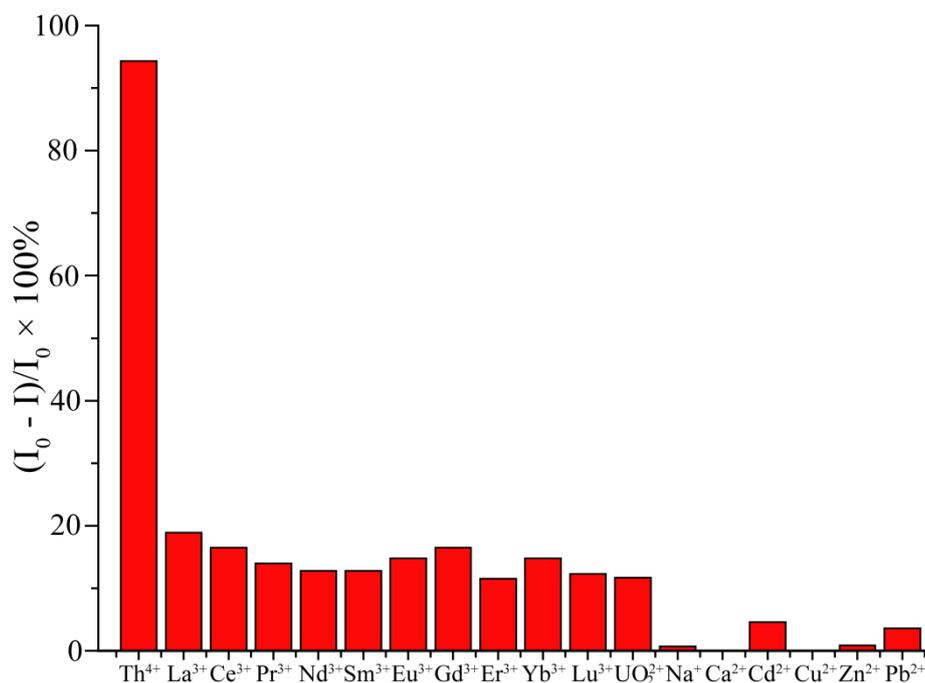
**Fig. S17** Fluorescence intensity changes ( $(I_0 - I)/I_0 \times 100\%$ ) of **1** (10 μM) in a mixed aqueous medium (CH<sub>3</sub>CN-H<sub>2</sub>O, v/v = 9:1,  $\lambda_{\text{ex}} = 310$  nm) upon addition of 1.0 equiv. of various metal ions.  $I_0$  is the fluorescent emission intensity at 390 nm of each free host and  $I$  is the fluorescent intensity after adding metal ions.
