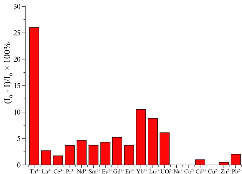
**Fig. S24** Fluorescence intensity changes  $((I_0 - I)/I_0 \times 100\%)$  of **2** ( $50 \mu\text{M}$ ) in a mixed aqueous medium ( $\text{CH}_3\text{CN-H}_2\text{O}$ ,  $v/v = 9:1$ ) upon addition of 1.0 equiv. of various metal ions.  $I_0$  is the fluorescent emission intensity at 391 nm of each free host and  $I$  is the fluorescent intensity after adding metal ions.
