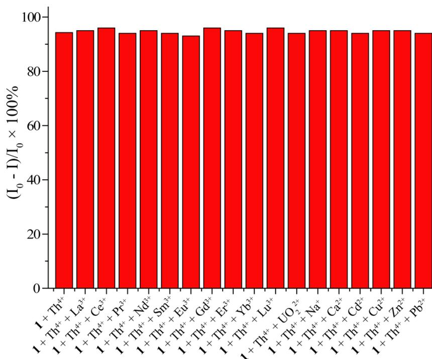
**Fig. S19** Fluorescence intensity changes ( $(I_0 - I)/I_0 \times 100\%$ ) of **1** (10  $\mu\text{M}$ ) in a mixed aqueous medium ( $\text{CH}_3\text{CN}-\text{H}_2\text{O}$ ,  $v/v = 9:1$ ) upon addition of 1.0 equiv. of various metal ions in the presence of 10 equiv. of background metal ions.  $I_0$  is the fluorescent emission intensity at 390 nm of each free host and  $I$  is the fluorescent intensity after adding metal ions.
