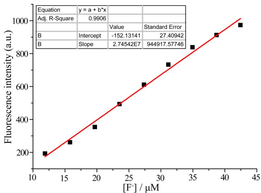
**Fig. S29** Curve of fluorescence intensity at  $390\ \text{nm}$  of  $1\text{-Th}^{4+}$  complex ( $10\ \mu\text{M}$ ) in a mixed aqueous medium ( $\text{CH}_3\text{CN-H}_2\text{O}$ ,  $v/v = 9:1$ ) versus increasing amount of  $\text{F}^-$ .
