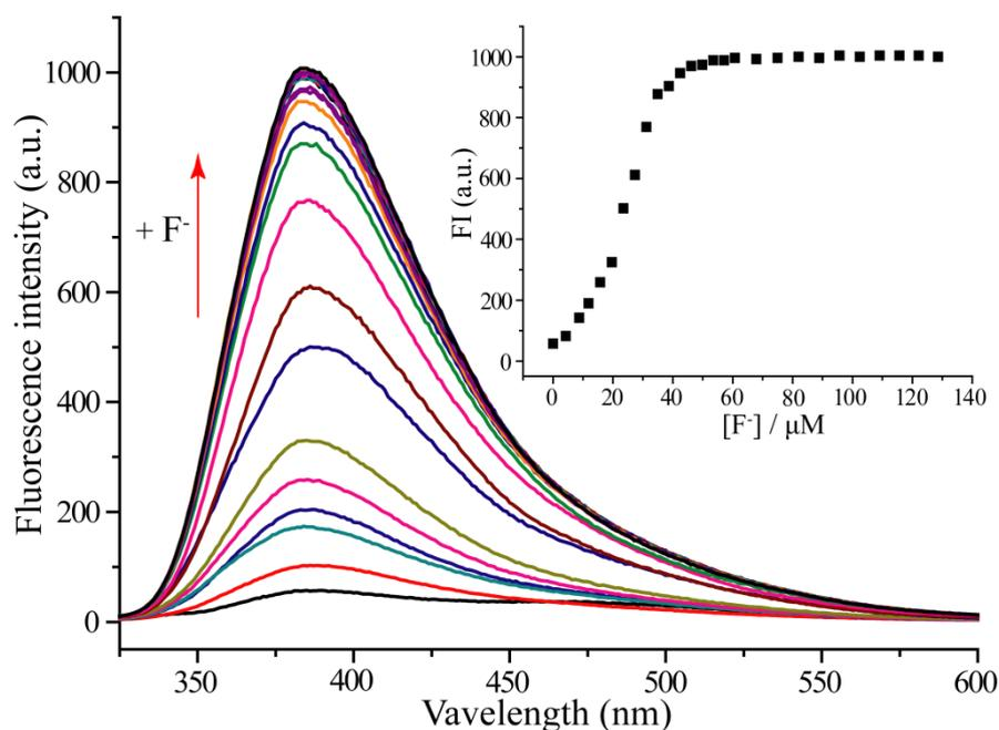
**Fig. S28** Fluorescence titration of the  $1\text{-Th}^{4+}$  complex ( $10\ \mu\text{M}$ ) with fluoride ion in a mixed aqueous medium ( $\text{CH}_3\text{CN-H}_2\text{O}$ ,  $v/v = 9:1$ ;  $\lambda_{\text{ex}} = 310\ \text{nm}$ ). Inset: fluorescence intensity as a function of  $\text{F}^-$  concentration.
