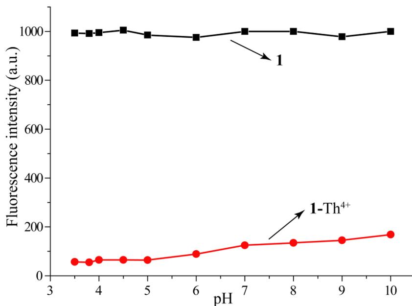
**Fig. S20** Plot of fluorescence intensities at 390 nm of **1** (10  $\mu\text{M}$ ) and **1-Th<sup>4+</sup>** ensemble (10  $\mu\text{M}$ ) in a mixed aqueous medium ( $\text{CH}_3\text{CN-H}_2\text{O}$ , v/v = 9:1;  $\lambda_{\text{ex}} = 310 \text{ nm}$ ) versus pH value (using NaOH and HCl to adjust pH to the desired value).
