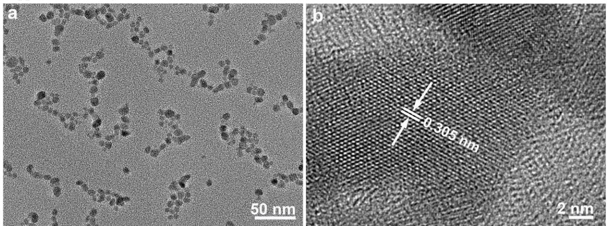
Fig. S1 (a) The TEM image and (b) HRTEM image of CuS nanocrystals
