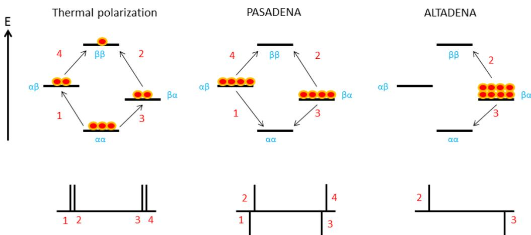
**Figure S1:** Schematic representation of the NMR characteristics of reaction products that form from natural abundant hydrogen addition (left) and *parahydrogen* addition under PASADENA (middle) and ALTADENA (right). The pictures reflect spin configurations while the lower traces correspond to the predicted NMR spectra.
