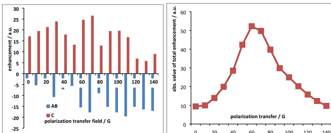
**Figure S10:** Left: Polarisation transfer field profile under SABRE of 3-hydroxypyridine  $^1\text{H}$  NMR signal enhancement in methanol- $d_4$  solution using **2c** as the catalyst with a 5 fold excess of 3-hydroxypyridine. **blue:**  $\text{H}_A$  and  $\text{H}_B$  and **red:**  $\text{H}_C$ . Right: Absolute value plot of the total proton signal enhancement of 3-hydroxypyridine versus polarization transfer field under SABRE.
