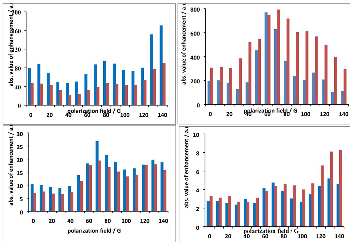
**Figure S3.** Absolute values of the total signal enhancement of pyridine in methanol- $d_4$  solution using **2c** (upper left), **4a** (upper right), **4b** (lower left), **4c** (lower right) complex with 2 (blue) and 34 (red) fold excesses of pyridine respectively as a function of polarization transfer field.
