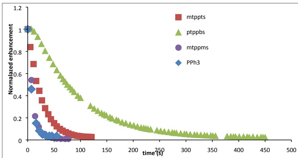
Figure S1. Plot of hydride signal enhancement versus time for **2**
