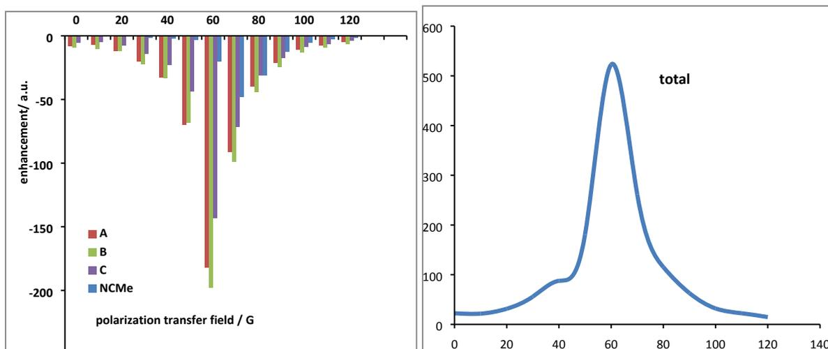
**Figure S8:** Left: Polarisation transfer field profile under SABRE of oxazole  $^1\text{H}$  NMR signal enhancement in ethanol- $d_6$  solution using **2c** as the catalyst with a 5 fold excess of oxazole and 2 fold excess of NCMe. **red:**  $\text{H}_A$ , **green:**  $\text{H}_B$  and **blue:**  $\text{H}_C$ . Right: Absolute value plot of the total proton signal enhancement of oxazole versus polarization transfer field under SABRE.
