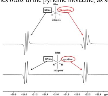
Figure S2. Hydride signals of complex **2c** in the corresponding  $^1\text{H}$  NMR spectra using normal (lower) and  $^{15}\text{N}$  labelled pyridine (upper).
