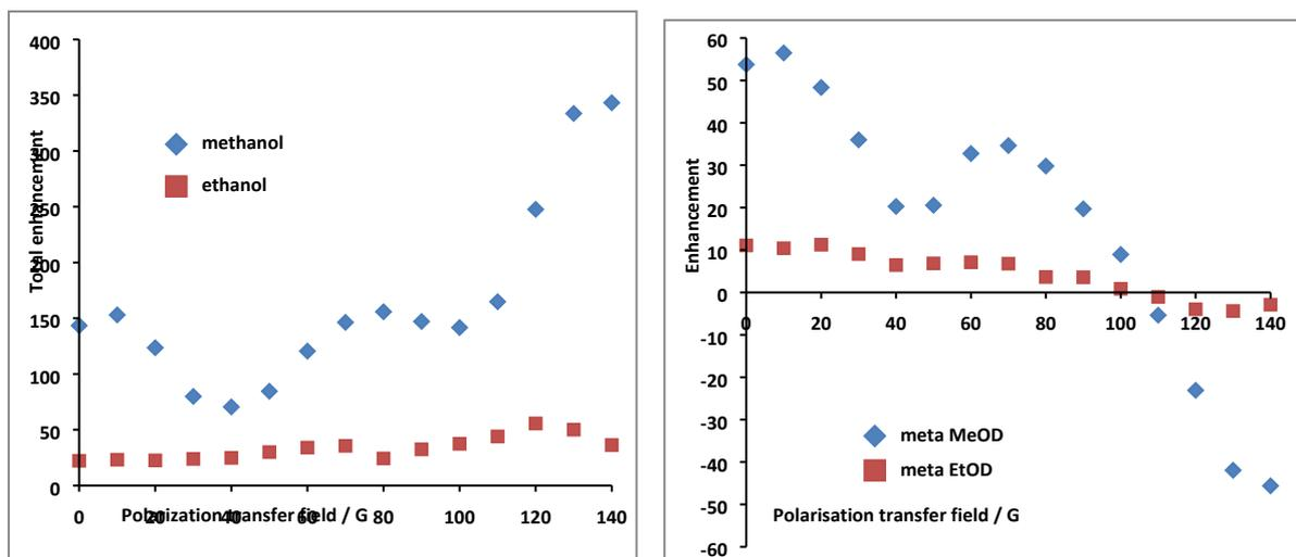
**Figure S5:** (left) Polarisation transfer field profiles for the pyridine total  $^1\text{H}$  NMR signal enhancement (fold) in the methanol- $d_4$  and ethanol- $d_6$  solution. (right) PTF profile of the *meta* proton signal enhancement in the methanol- $d_4$  and ethanol- $d_6$  solution using  $[2a] = 5.5$  mM, 20 fold pyridine, 2 fold NCMe, 3 mL solvent .
