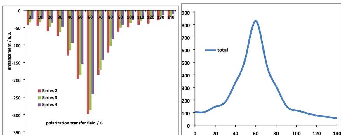
**Figure S7:** Left: Polarisation transfer field profile under SABRE of oxazole  $^1\text{H}$  NMR signal enhancement in methanol- $d_4$  solution using  $2c$  as the catalyst with a 5 fold excess of oxazole and 2 fold excess of NCMe. **red:**  $H_A$ , **green:**  $H_B$  and **blue:**  $H_C$ . Right: Absolute value plot of the total proton signal enhancement of oxazole versus polarization transfer field under SABRE.
