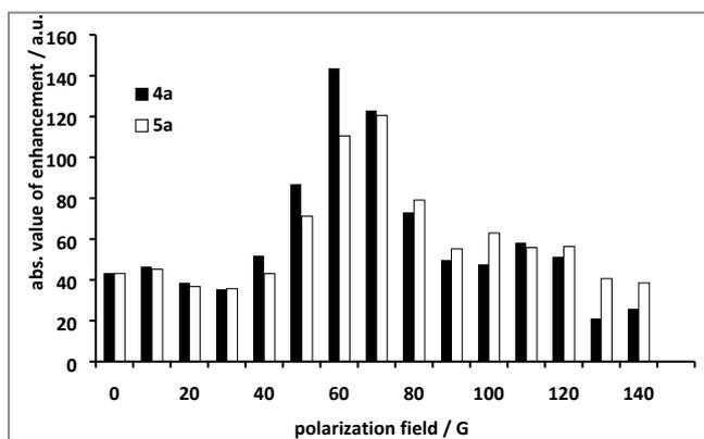
**Figure S12:** Absolute values of the total  $^1\text{H}$  NMR signal enhancement of pyridine in methanol- $d_4$  solution using **4a** (black) and **5a** (white), when a 19-fold excess of pyridine is present.
