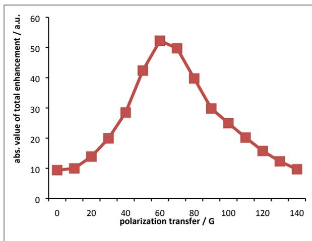
**Figure S11:** Polarisation transfer field profile of 3-hydroxypyridine proton signal enhancement in the methanol- $d_4$  solution using **4a** as the catalyst with a 5 fold excess of 3-hydroxypyridine.
