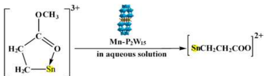
Scheme S1 Hydrolysis of estertin into open chain carboxyethyltin group during the synthetic process of SnR-Mn-P 2 W 15
