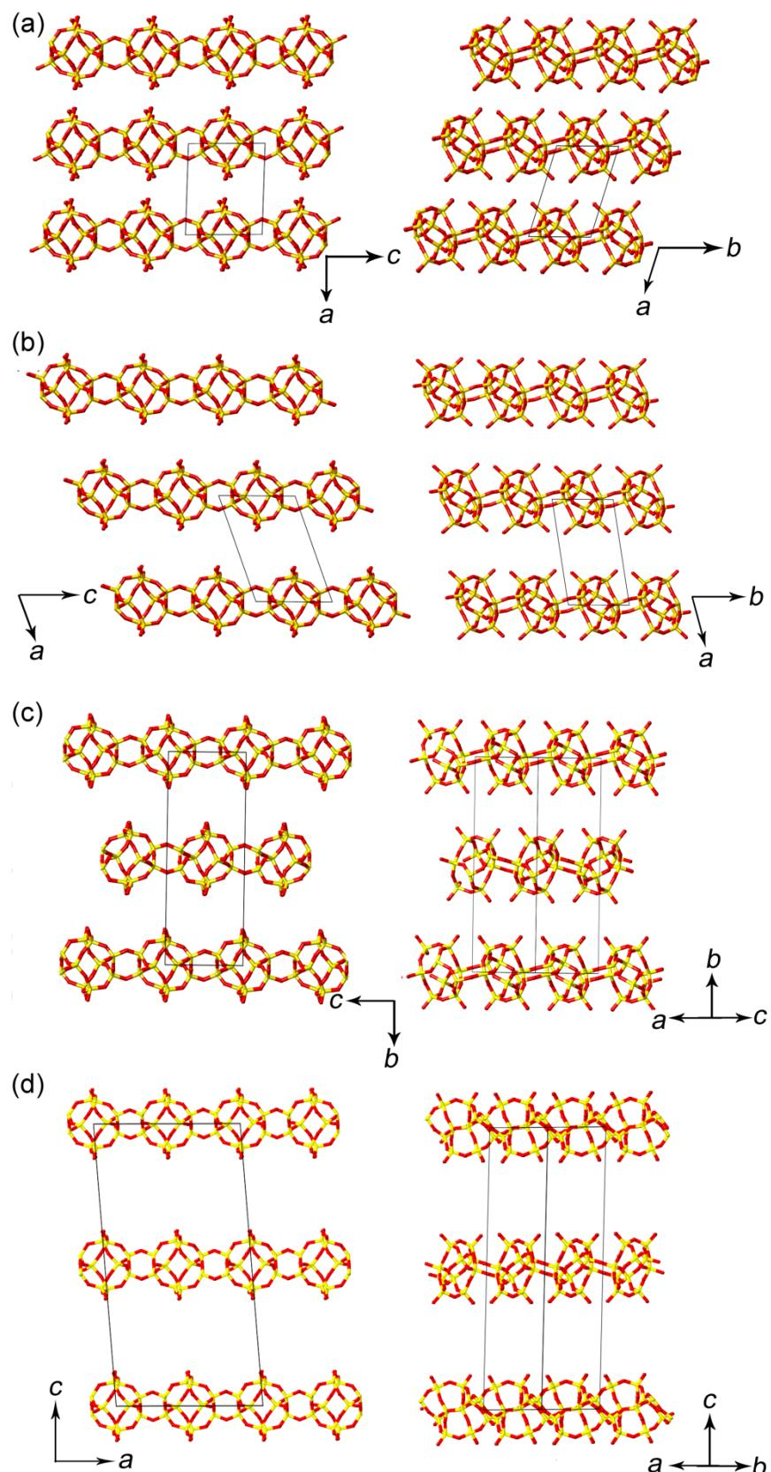
**Figure S6.** Framework comparison among (a) PKU-13, (b) PKU-13a, (c) HUS-2 and (d) HUS-7. The Si atoms are drawn in yellow and O atoms in red.
