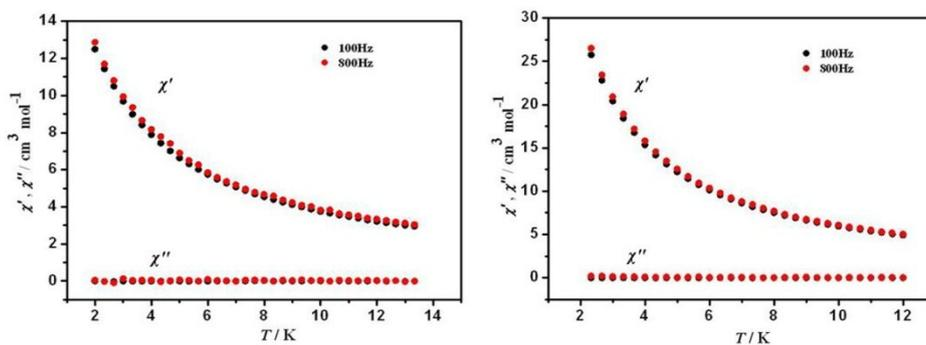
Fig. S6 Temperature dependence of ac susceptibilities under zero field for 1 (left) and 2 (right).
