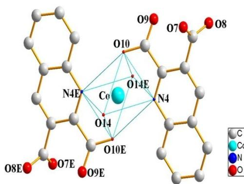
**Fig. S3** Coordination environment of Co. Atoms with E in their labels are symmetry generated. Symmetry code: E:  $-x, 1-y, -z$ .
