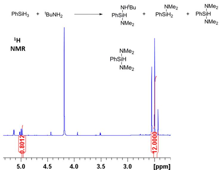
**ESI 3b**  $^1\text{H}$  NMR spectrum ( $d_8$ -toluene) showing the product  $\text{PhSiH}(\text{NMe}_2)_2$  from the reaction between  $\text{PhSiH}_3$  (1 equiv) and  ${}^t\text{BuNH}_2$  (2 equiv) catalysed by  $\text{Al}(\text{NMe}_2)_3$  (10 mol%).
