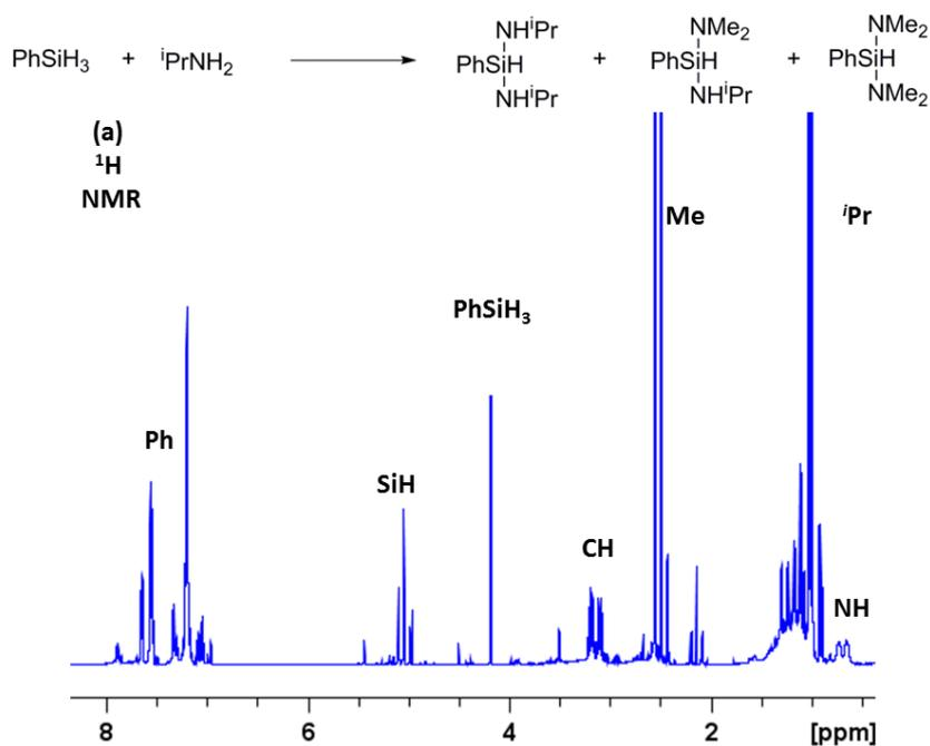
**ESI 2c** (a)  $^1\text{H}$  NMR spectrum ( $d_8$ -toluene) showing the different regions of the products formed by the reaction between  $\text{PhSiH}_3$  (1 equiv) and  $^i\text{PrNH}_2$  (1.5 equiv) catalysed by  $\text{Al}(\text{NMe}_2)_3$  (10 mol%).
