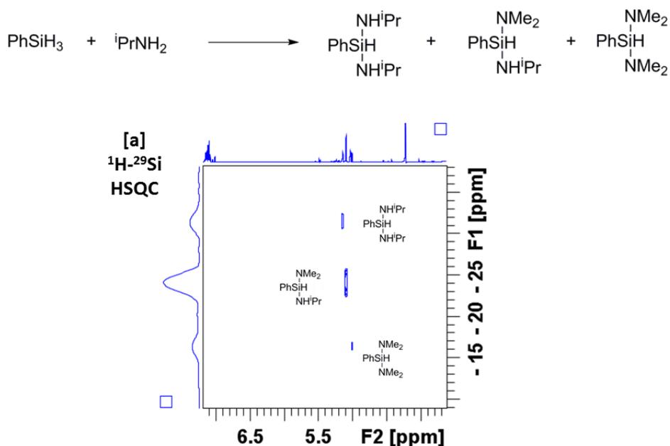
**ESI 2b** (a)  $^1\text{H}$ - $^{29}\text{Si}$  HSQC NMR spectrum (d<sub>8</sub>-toluene) showing the three silyl hydride (SiH) signals correlating with the three  $^{29}\text{Si}$  environments of the products PhSiH(HN<sup>i</sup>Pr)<sub>2</sub>, PhSiH(HN<sup>i</sup>Pr)(NMe<sub>2</sub>) and PhSiH(NMe<sub>2</sub>)<sub>2</sub> formed by the reaction between PhSiH<sub>3</sub> (1 equiv) and <sup>i</sup>PrNH<sub>2</sub> (1.5 equiv) catalysed by Al(NMe<sub>2</sub>)<sub>3</sub> (10 mol%).
