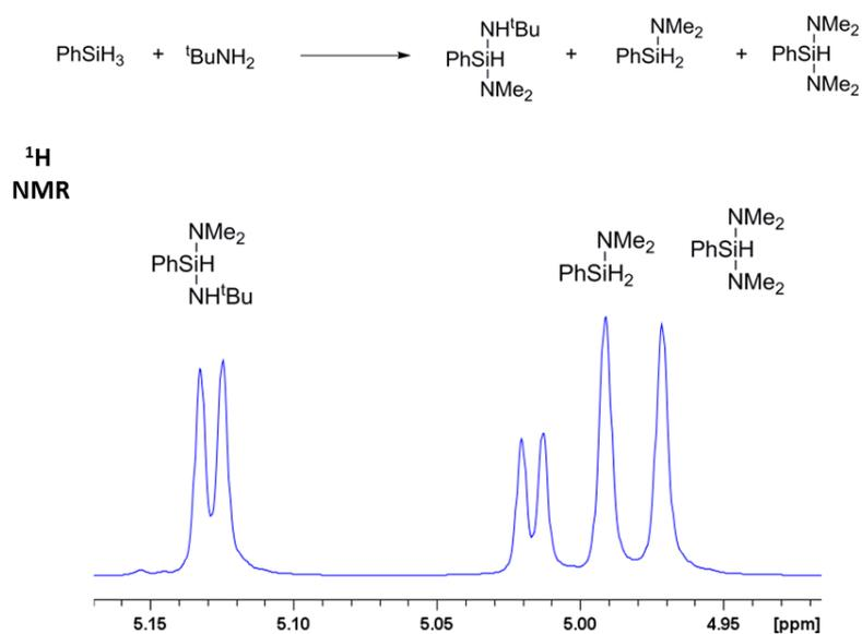
**ESI 3a**  $^1\text{H}$  NMR spectrum ( $d_8$ -toluene) showing the silyl hydride region for the products  $\text{PhSiH}(\text{HN}^t\text{Bu})(\text{NMe}_2)$ ,  $\text{PhSiH}_2(\text{NMe}_2)$  and  $\text{PhSiH}(\text{NMe}_2)_2$  formed by the reaction between  $\text{PhSiH}_3$  (1 equiv) and  $^t\text{BuNH}_2$  (2 equiv) catalysed by  $\text{Al}(\text{NMe}_2)_3$  (10 mol%).
