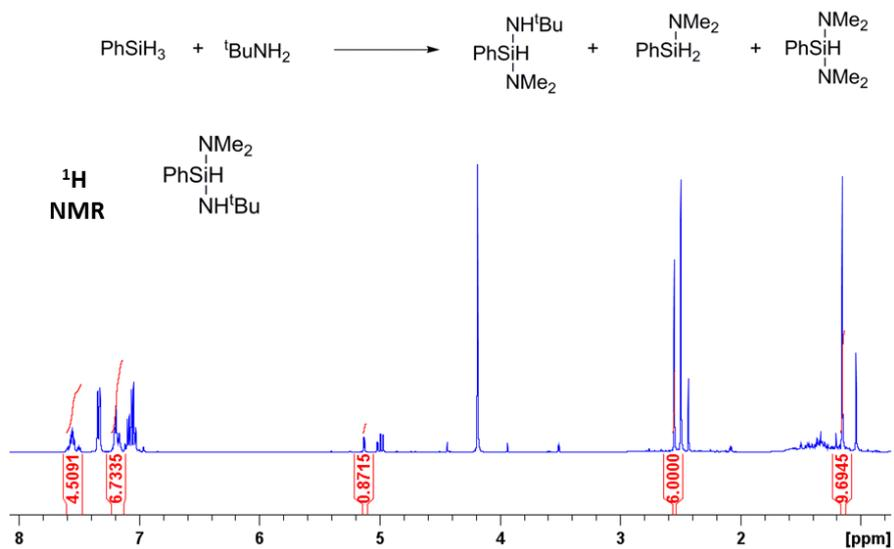
**ESI 3c**  $^1\text{H}$  NMR spectrum ( $d_8$ -toluene) showing the product  $\text{PhSiH}(\text{HN}^t\text{Bu})(\text{NMe}_2)$  from the reaction between  $\text{PhSiH}_3$  (1 equiv) and  ${}^t\text{BuNH}_2$  (2 equiv) catalysed by  $\text{Al}(\text{NMe}_2)_3$  (10 mol%).
