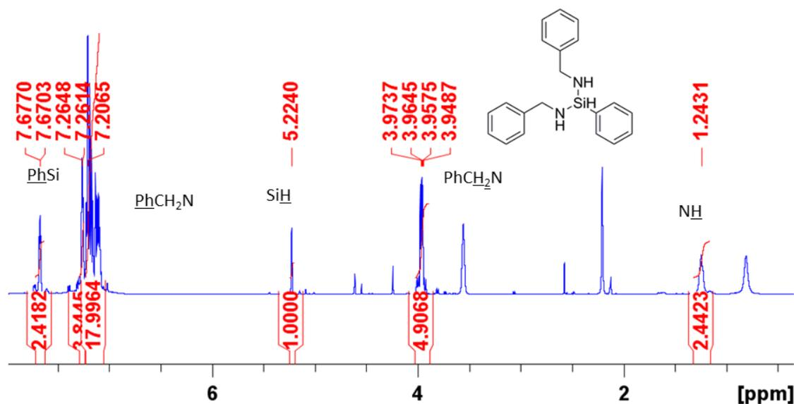
**ESI 1a**  $^1\text{H}$  NMR spectrum ( $d_8$ -toluene) of the reaction between  $\text{PhSiH}_3$  (1 equiv) and  $\text{BnNH}_2$  (3 equiv) catalysed by  $\text{Al}(\text{NMe}_2)_3$  (10 mol%) showing the formation of  $\text{PhSiH}(\text{BnNH})_2$ .
