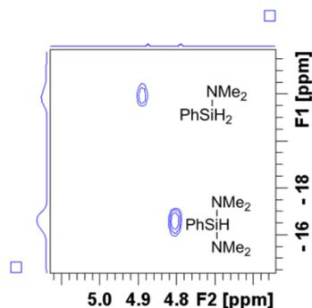
**ESI 5a**  $^1\text{H}$ - $^{29}\text{Si}$  HSQC NMR spectrum ( $d_8$ -toluene) showing the correlation of two  $^1\text{H}$  silyl hydride (Si-H) signals and the  $^{29}\text{Si}$  signals of the two products  $\text{PhSiH}(\text{NMe}_2)_2$  and  $\text{PhSiH}(\text{NMe}_2)$  ( $\delta = -22$  ppm and  $-17$  ppm respectively) formed by the stoichiometric reaction between  $\text{PhSiH}_3$  and  $\text{Al}(\text{NMe}_2)_3$ .
