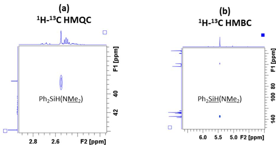
**ESI 4b** (a)  $^1\text{H}$ - $^{13}\text{C}$  HMQC correlating the  $\text{CH}_3$  ( $^1\text{H}$   $\delta = 2.55\text{ ppm}$ ) with the  $^{13}\text{C}$  signal ( $\delta = 38.4\text{ ppm}$ ) in  $\text{Ph}_2\text{SiH}(\text{NMe}_2)$ . (b)  $^1\text{H}$ - $^{13}\text{C}$  HMBC correlating the Si-H proton ( $\delta = 5.40\text{ ppm}$ ) and the  $\text{NMe}_2$   $^{13}\text{C}$  signal ( $38.4\text{ ppm}$ ) in  $\text{Ph}_2\text{SiH}(\text{NMe}_2)$ .
