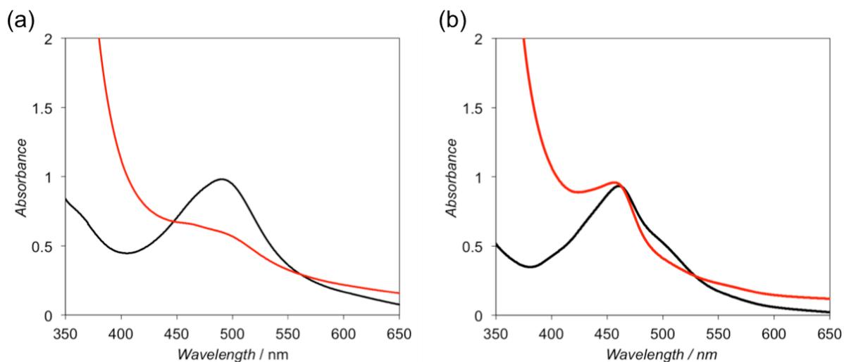
**Fig. S6** UV-visible spectra of (a) **1•PA** (Ru concentration 0.08 mM) in water (black) and the mixture of **1•PA** (Ru concentration 0.08 mM) and  $(\text{NH}_4)_2[\text{Ce}(\text{NO}_3)_6]$  (3.2 mM, 40 equiv.) (red), and (b) **1•PG** (Ru concentration 0.08 mM) in water (black) and the mixture of **1•PG** (Ru concentration 0.08 mM) and  $(\text{NH}_4)_2[\text{Ce}(\text{NO}_3)_6]$  (3.2 mM, 40 equiv.) (red).
