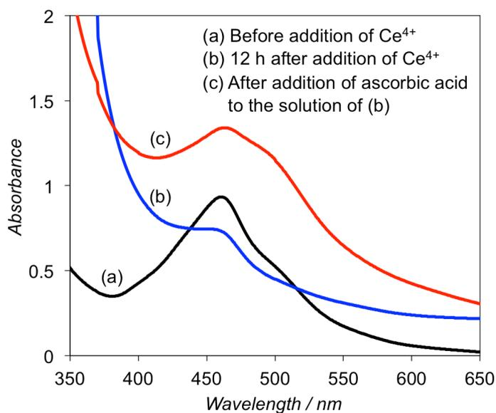
**Fig. S5** UV-visible spectra of (a) **1•PG** (Ru concentration 0.08 mM) in water, (b) the reaction mixture after 12 h from addition of  $(\text{NH}_4)_2[\text{Ce}(\text{NO}_3)_6]$  (3.2 mM, 40 equiv.) to **1•PG** (Ru concentration 0.08 mM), and (c) the solution after addition of ascorbic acid (1.9 mM) to the solution of (b).
