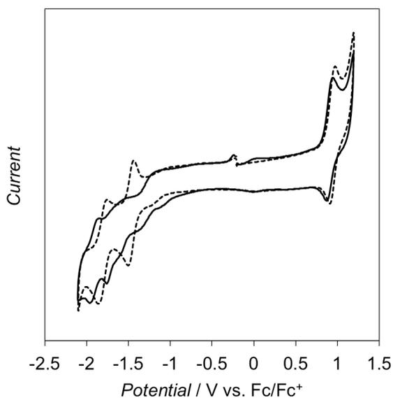
**Fig. S2** Cyclic voltammograms of **1** (solid line, 0.5 mM) and **2** (dashed line, 0.5 mM) in acetonitrile under  $N_2$  atmosphere, recorded at a scan rate of 10 mV/s using a glassy carbon working electrode, a Pt wire counter electrode, and a [Ag]/[AgCl] reference electrode. The supporting electrolyte was 0.1 M tetra(n-butyl)ammonium perchlorate. The potentials were corrected by ferrocene/ferrocinium couple as an internal standard.
