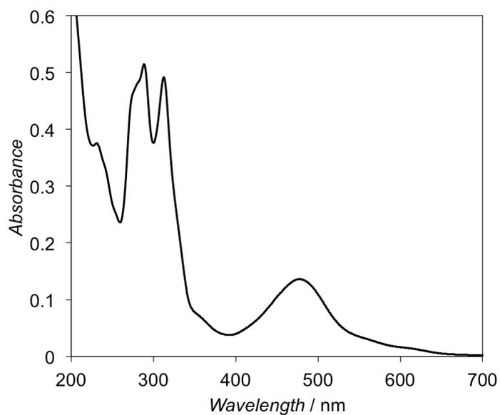
**Fig. S4** UV-visible spectrum of **cRu** in 50 mM  $\text{Na}_2\text{HPO}_4$ . The sample heated at 85 °C for 19 h before the measurement.
