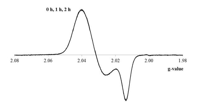
Supplementary Figure 1: The preparations of GS-DNIC made by addition of  $Fe^{2+}$  (200  $\mu$ M) to GSH (20 mM)/GSNO (400  $\mu$ M) and incubated 20 min. in pH 7 were checked for stability in 1 h and 2 h at room temperature in a quartz tube in the air in the dark. No visible deterioration of M-DNIC concentration was found. EPR: 1 scan at 77 K, microwave power 1 mW, microwave frequency 9.5 GHz and modulation amplitude 0.3 mT.
