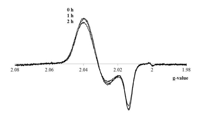
Supplementary Figure 2: The preparations of GS-DNIC made by addition of  $Fe^{2+}$  (200  $\mu$ M) to GSH (20 mM)/GSNO (400  $\mu$ M) and incubated 20 min.in pH 6 were checked for stability in 1 h and 2 h at room temperature in a quartz tube in the air in the dark. We observed ca 10% decrease of M-DNIC concentration. EPR: 1 scan at 77 K, microwave power 1 mW, microwave frequency 9.5 GHz and modulation amplitude 0.3 mT.
