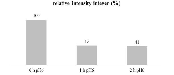
Supplementary Figure 4: The preparations of GS-DNIC made by addition of  $Fe^{2+}$  (1  $\mu$ M) to GSH (7 mM)/GSNO (700  $\mu$ M) and incubated 20 min. in pH 6 were checked for stability in 1 h and 2 h at room temperature in a quartz tube in the air in the dark (A). We observed ca 60% decrease of M-DNIC concentration after 2 h (B). EPR: 8 scans at 77 K, microwave power 1 mW, microwave frequency 9.5 GHz and modulation amplitude 0.3 mT.
