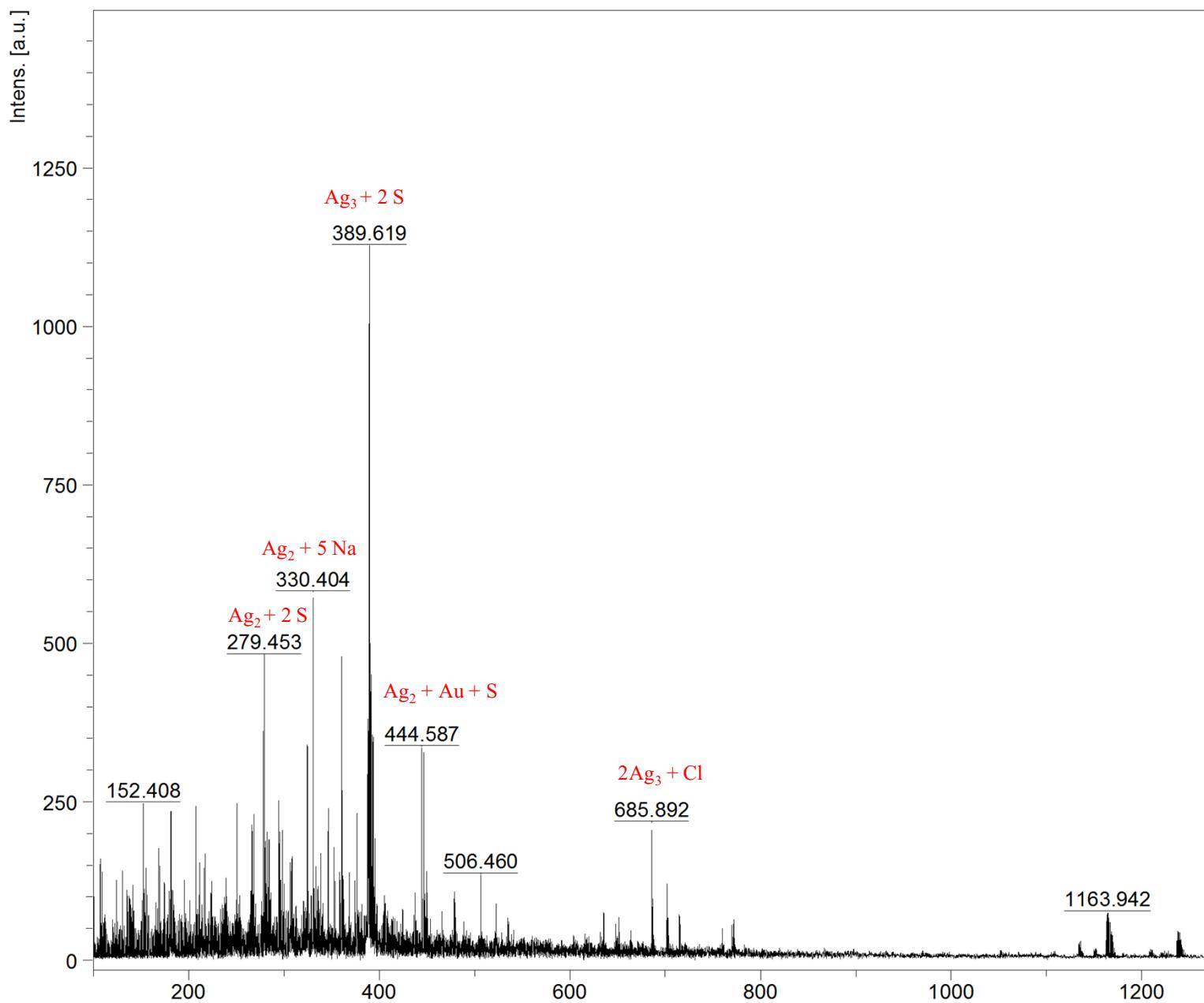
Figure S4(b): MALDI-TOF mass spectral profile of HFL solution (sinapinic acid as matrix).
