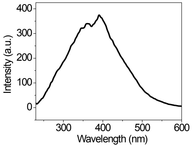
Figure S7: Excitation spectral profile of HFL when emission maximum is 635 nm.
