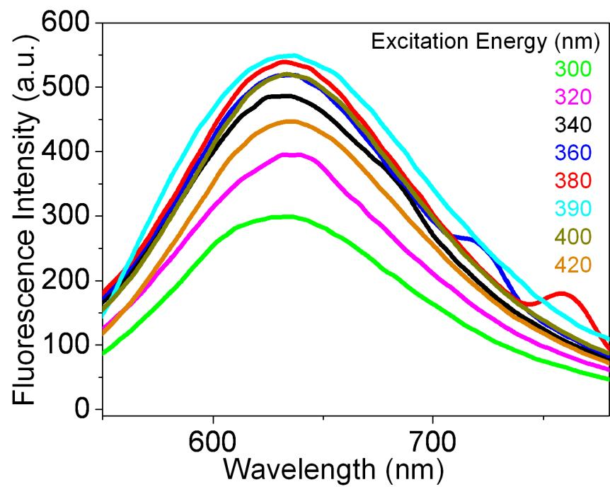
Figure S5: Fluorescence spectral profile of HFL at different excitation energy.
