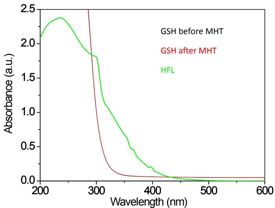
Figure S2: UV-vis spectral profile of aqueous GSH before and after MHT, and HFL.
