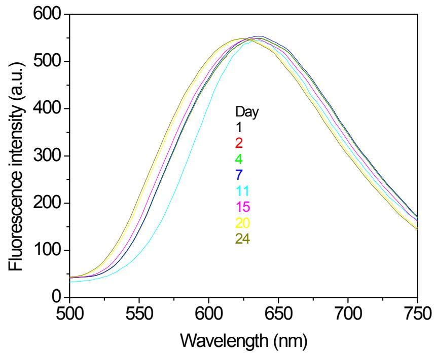
Figure S3: Fluorescent spectral profile of HFL at different time intervals.
