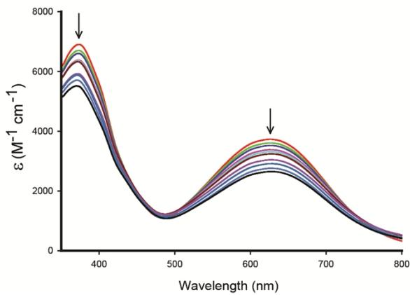
**Figure S5.** Spectral traces of **2** in  $\text{CH}_2\text{Cl}_2$  298 K with low power visible light ( $15 \text{ mW/cm}^2$ )
