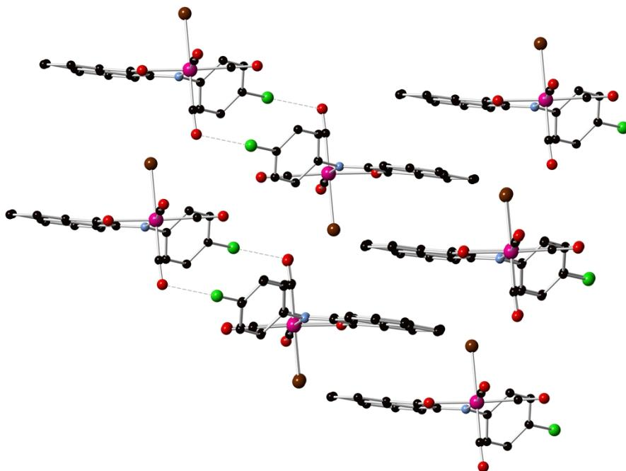
**Figure S4.** Packing diagram of **2** showing growth along the y axis. The Cl–O interactions are shown in addition to  $\pi$ -stacking.
