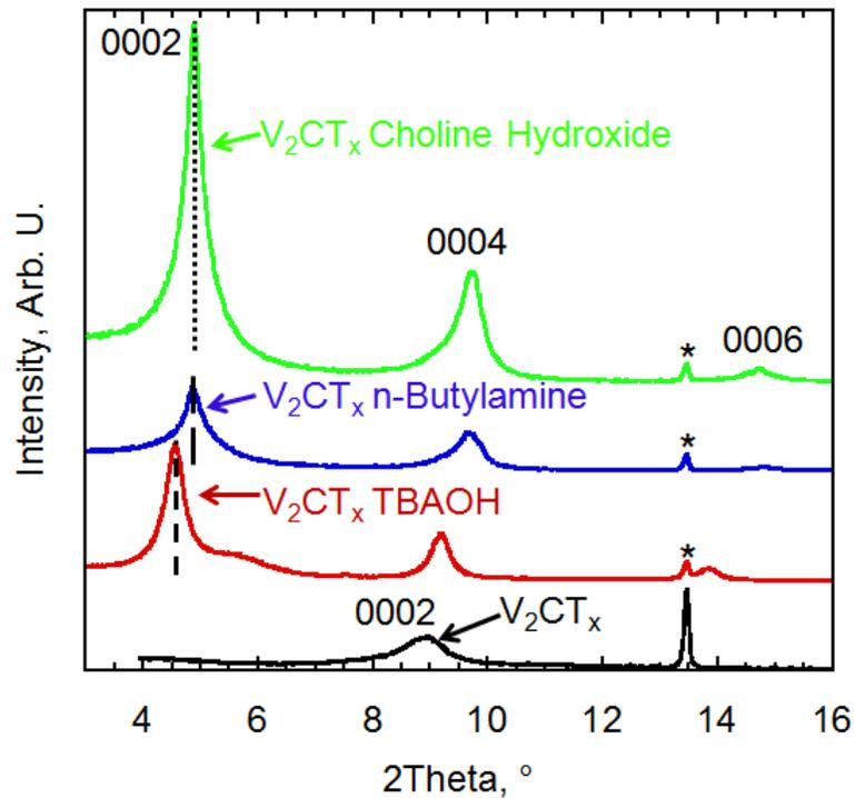
Fig. S1. XRD patterns for  $V_2CT_x$  samples before and after treatments with different organic bases; tetrabutylammonium hydroxide (TBAOH), n-butylamine, and choline hydroxide for 4 hours each at room temperature. The \* symbols indicate the 0002 peak position of unreacted  $V_2AlC$  in MXene samples.
