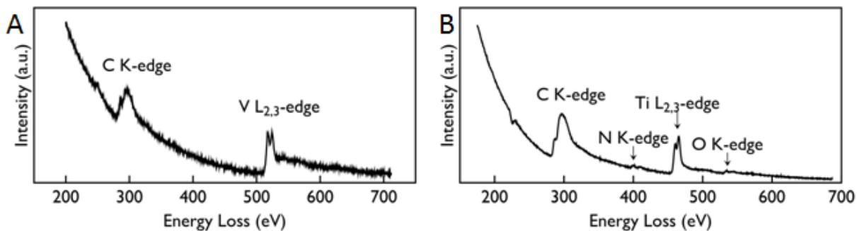
Fig. S2. Electron energy loss spectra of delaminated flakes of (A)  $V_2CT_x$ , and (B)  $Ti_3CNT_x$
