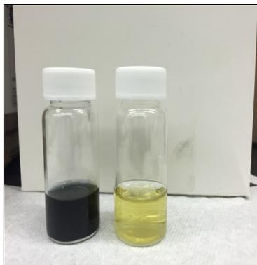
Figure S3. Photograph for two vials contain freshly delaminated  $V_2CT_x$  in water (the black liquid in the left vial) and  $V_2CT_x$  solution that was kept in air for 48 h (the yellow solution at the right).
