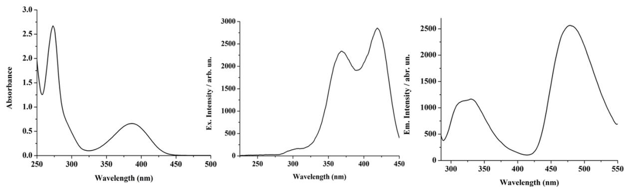
**Fig.S37** Absorbance, excitation and emission spectra (left to right) of [L1+Al<sup>3+</sup>] (in EtOH/ H<sub>2</sub>O, 1/1, v/v, 20 μM)
