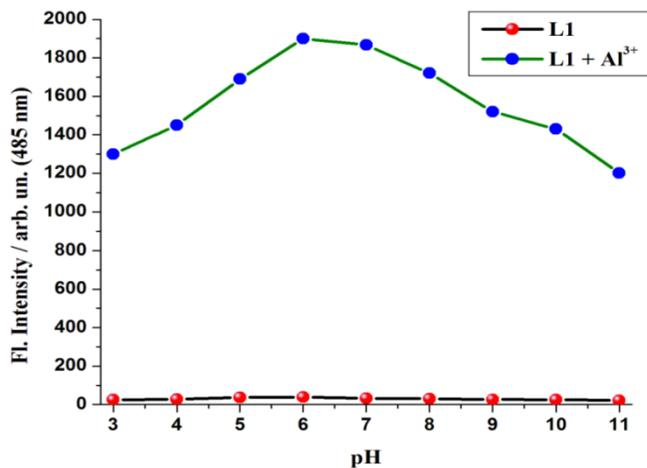
**Fig.S2** Effect of pH on the emission intensities of free L1 (20  $\mu\text{M}$ ) and [L +  $\text{Al}^{3+}$ ] system (1: 50, mole ratio,  $\lambda_{\text{ex}}$ , 276 nm)
