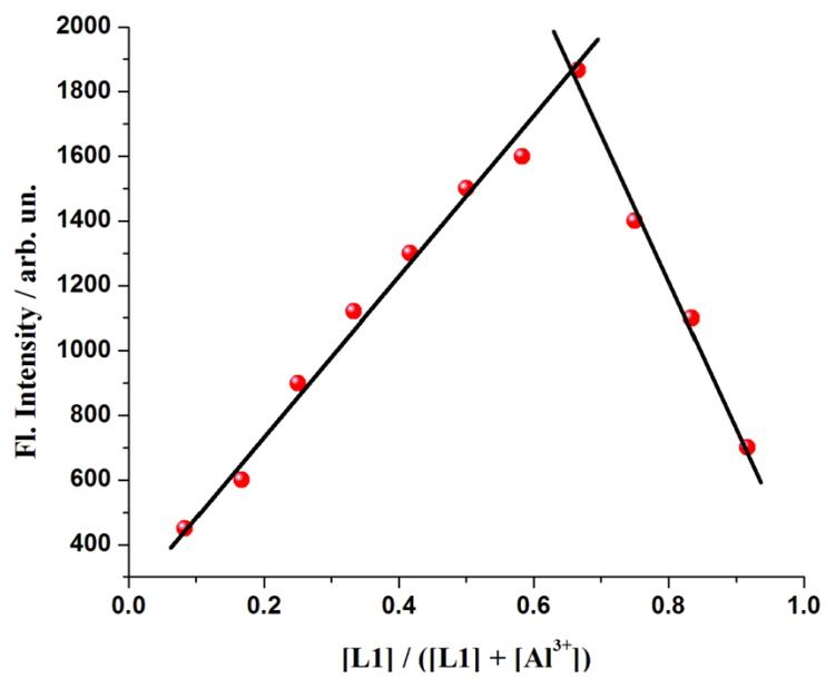
**Fig.S19** Job's plot for stoichiometry determination of the adduct between L1 and  $Al^{3+}$
