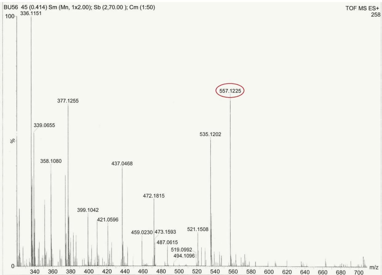
**Fig.S38** QTOF-MS spectrum of the product derived upon addition of  $\text{Al}^{3+}$  to  $[\text{L1}+\text{Zn}^{2+}]$  complex
