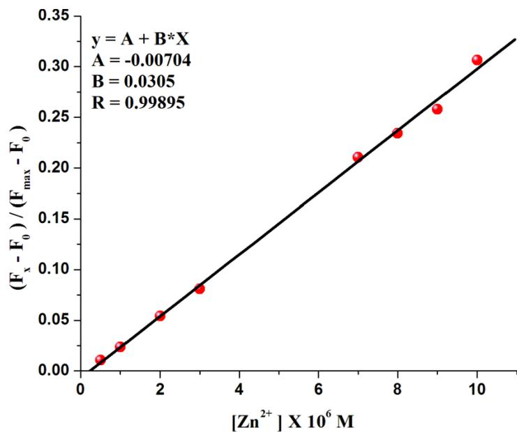
**Fig.S9** Emission intensities of **L1** (20  $\mu$ M) as a function of externally added Zn<sup>2+</sup> in EtOH/H<sub>2</sub>O 1/1, v/v,  $\lambda_{\text{ex}}$ , 276 nm,  $\lambda_{\text{em}}$ , 450 nm (used data of Fig.2)
