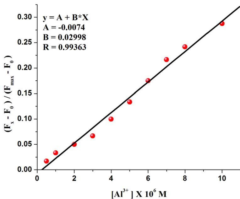
**Fig.S10** Emission intensities of **L1** (20  $\mu$ M) as a function of externally added [Al<sup>3+</sup>] in EtOH/H<sub>2</sub>O, 1/1, v/v,  $\lambda_{\text{ex}}$ = 276 nm,  $\lambda_{\text{em}}$ = 485 nm (used data of Fig.3)
