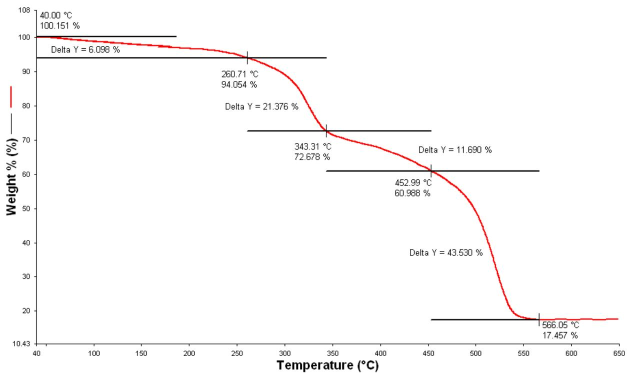
Fig.S32 Thermogram of [L1+Zn<sup>2+</sup>] complex
