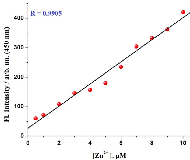
**Fig.S3a** Linear region of the plot of emission intensities of **L1** (10  $\mu\text{M}$ ,  $\lambda_{\text{ex}} = 276 \text{ nm}$ ,  $\lambda_{\text{em}} = 450 \text{ nm}$ ) as a function of externally added  $\text{Zn}^{2+}$  (0.5-10  $\mu\text{M}$ )
