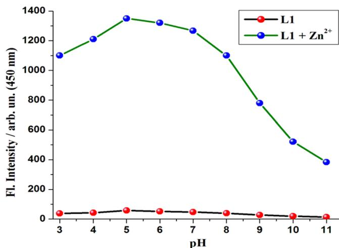
**Fig.S1** Effect of pH on the emission intensities of free L1 (20  $\mu\text{M}$ ) and  $[\text{L} + \text{Zn}^{2+}]$  system (1: 50, mole ratio,  $\lambda_{\text{ex}}$ , 276 nm)
