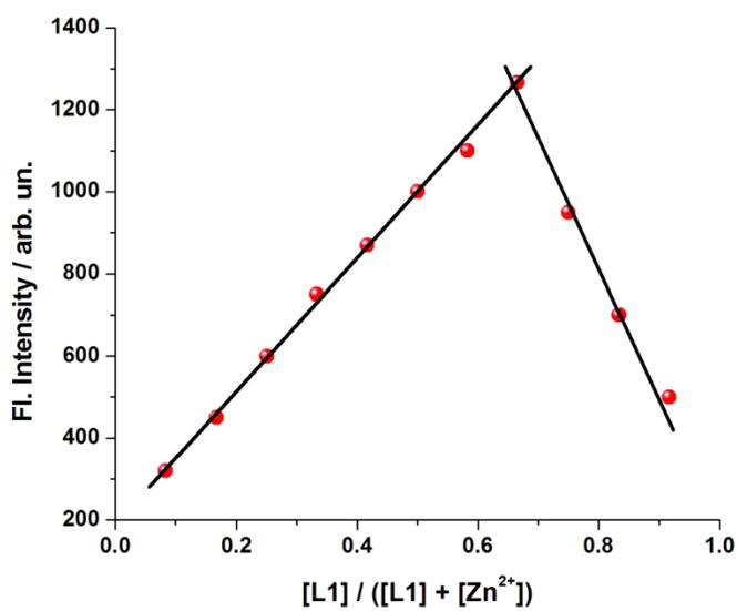
Fig.S18 Job's plot for stoichiometry determination of the adduct between L1 and Zn<sup>2+</sup>
