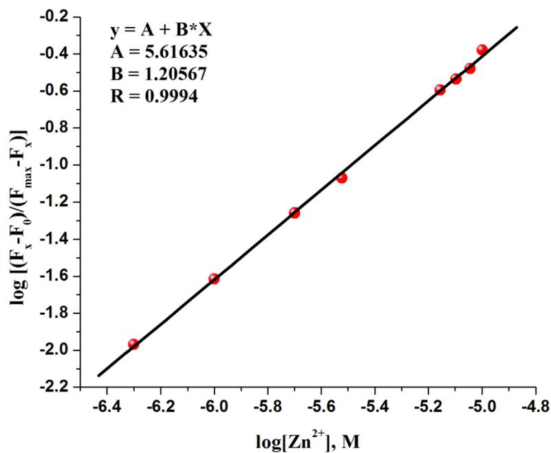
**Fig.S7** Hill plot for determination of binding constant of L1 to  $\text{Zn}^{2+}$  in 1:1 EtOH/ $\text{H}_2\text{O}$  (data from Fig.2 is used)
