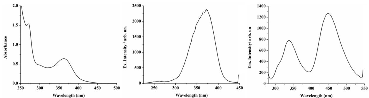
Fig.S33 Absorbance, excitation and emission spectra (left to right) of [L1+Zn<sup>2+</sup>] (in EtOH/ H<sub>2</sub>O, 1/1, v/v, 20 μM)
