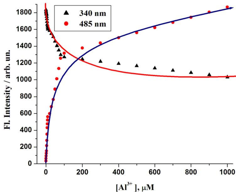
**Fig.S4** Plot of emission intensities of **L1** (20  $\mu\text{M}$ ,  $\lambda_{\text{ex}} = 276 \text{ nm}$ ,  $\lambda_{\text{em}} = 340 \text{ nm}$  and 485 nm) as a function of externally added  $\text{Al}^{3+}$  (0.5-1000  $\mu\text{M}$ )
