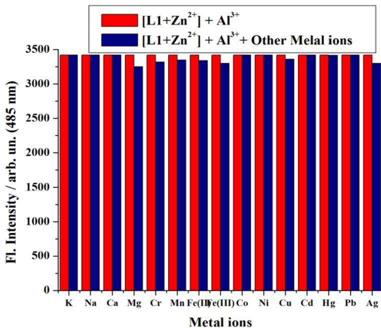
Fig.S14 Relative emission intensities of {[L1 - Zn<sup>2+</sup>] + Al<sup>3+</sup>} system in presence of various cations
