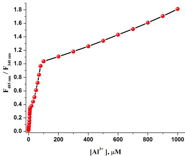
**Fig.S6** Changes in the emission intensity ratio ( $F_{485}/F_{340}$ ) of L1 upon gradual addition of  $\text{Al}^{3+}$
