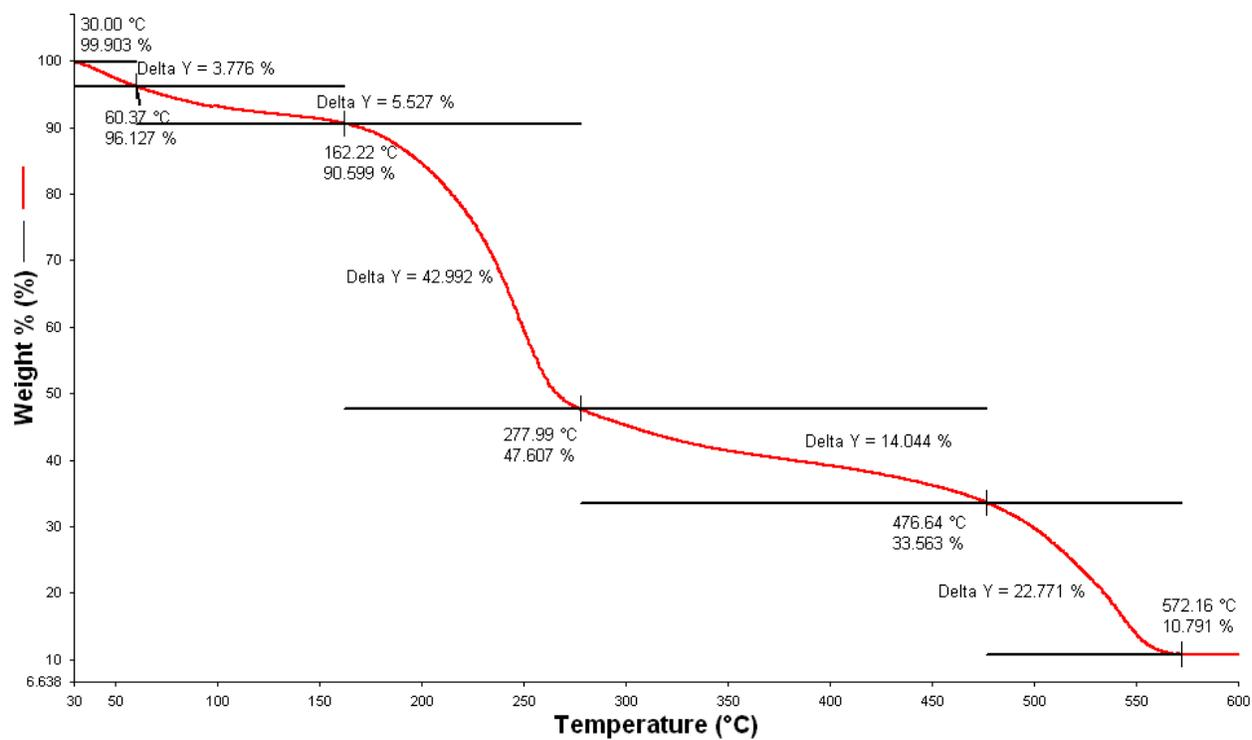
**Fig.S36** Thermogram of [L1+Al<sup>3+</sup>] complex
