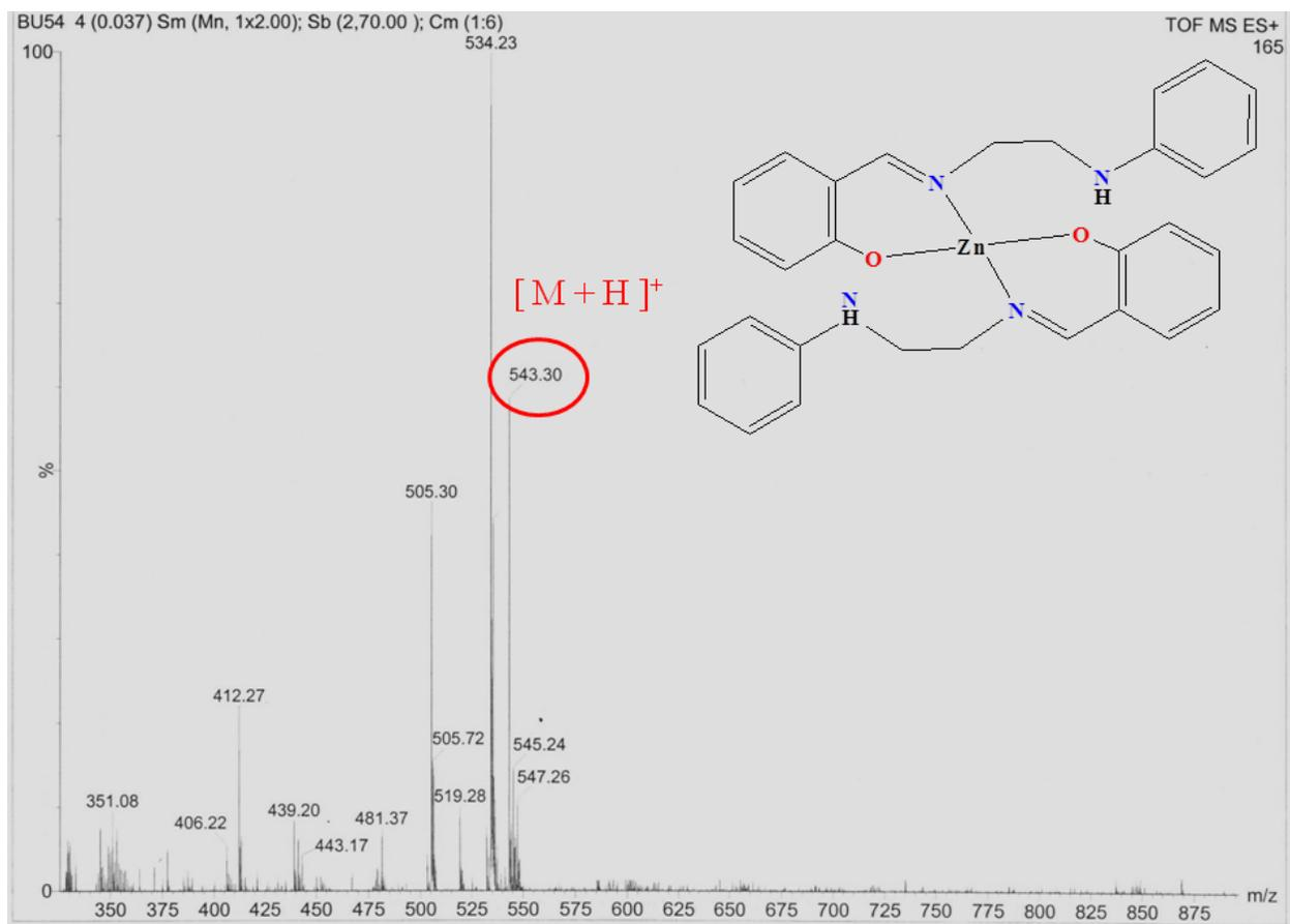
**Fig.S30** QTOF-MS spectrum of [L1+Zn<sup>2+</sup>] complex
