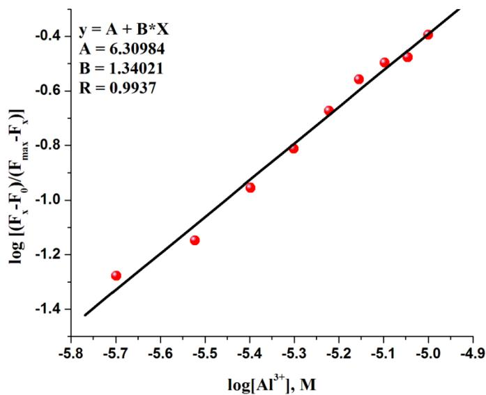
**Fig.S8** Hill plot for determination of binding constant of L1 to  $\text{Al}^{3+}$  in 1:1 EtOH/ $\text{H}_2\text{O}$  (data used from Fig.3)
