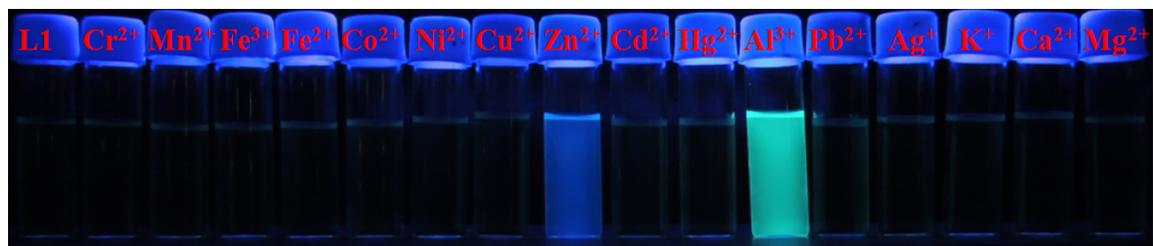
**Fig.S15** Changes of colour of L1 (30  $\mu\text{M}$ ) upon addition of equimolar various cations (500  $\mu\text{M}$ ) under UV light
