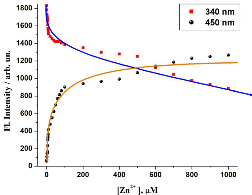
**Fig.S3** Plot of emission intensities of L1 (20  $\mu\text{M}$ ,  $\lambda_{\text{ex}}$  = 276 nm,  $\lambda_{\text{em}}$  = 340 nm and 450 nm) as a function of externally added  $\text{Zn}^{2+}$  (0.5-1000  $\mu\text{M}$ )
