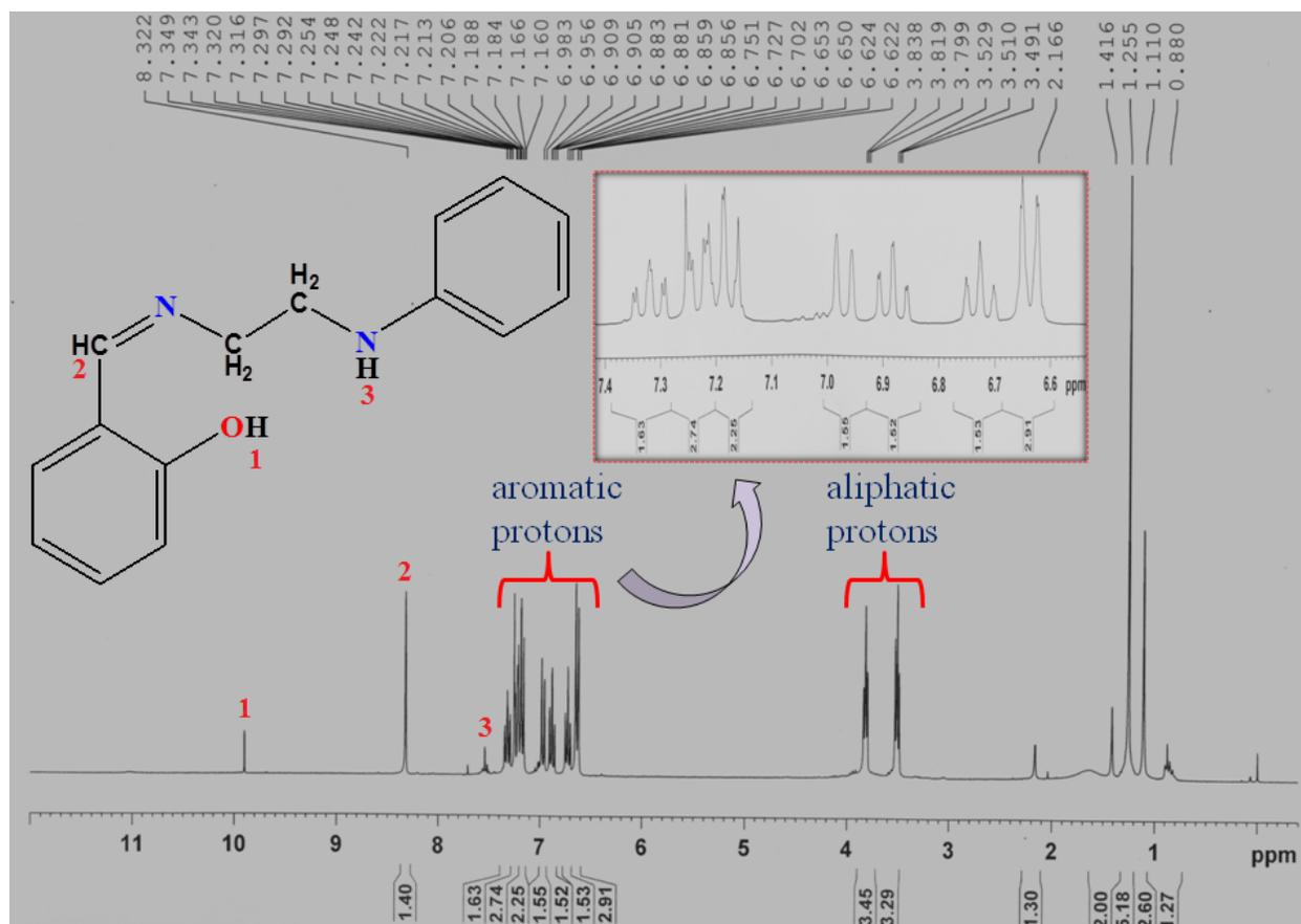
**Fig.S24**  $^1\text{H}$  NMR spectrum of L1 in  $\text{CDCl}_3$
