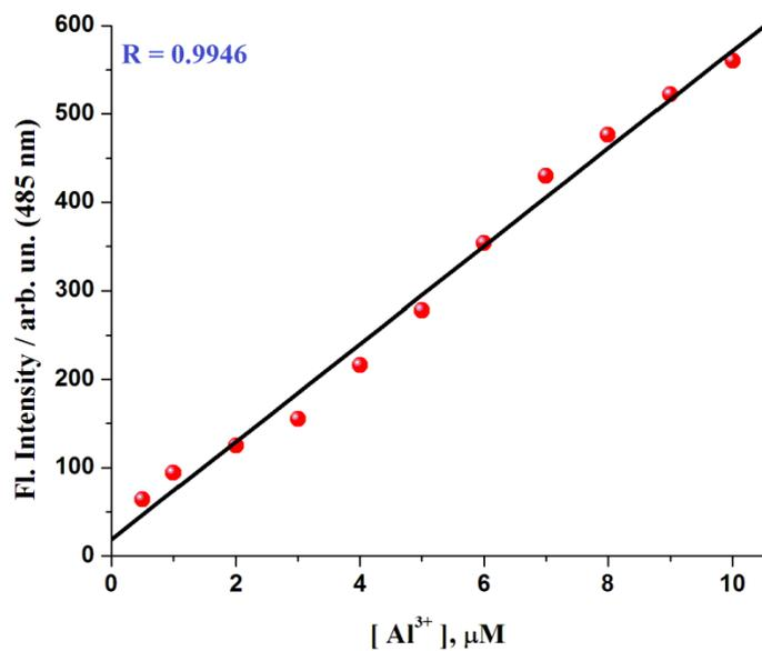
**Fig.S4a** Linear region of the plot of emission intensities of **L1** (20  $\mu\text{M}$ ,  $\lambda_{\text{ex}} = 276 \text{ nm}$ ,  $\lambda_{\text{em}} = 485 \text{ nm}$ ) as a function of externally added  $\text{Al}^{3+}$  (0.5-10  $\mu\text{M}$ )
