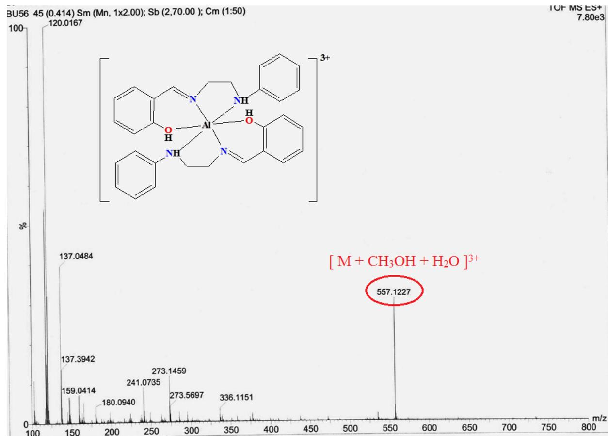
**Fig.S34** QTOF-MS spectrum of [L1+Al<sup>3+</sup>] complex
