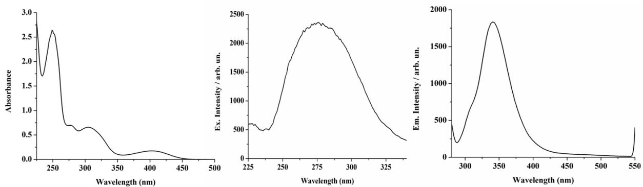
**Fig.S29** Absorbance, excitation and emission spectra (left to right) of L1 in EtOH (20 μM)
