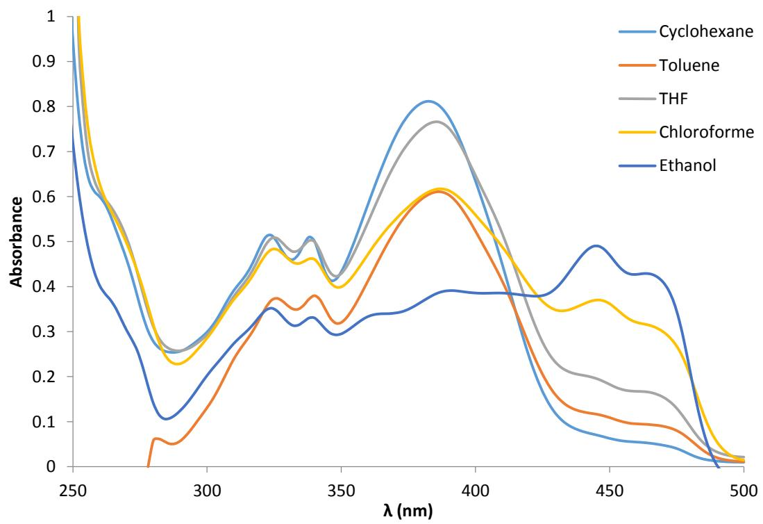
*Fig. S5* UV-VIS Spectra of *3e* in different solvents
