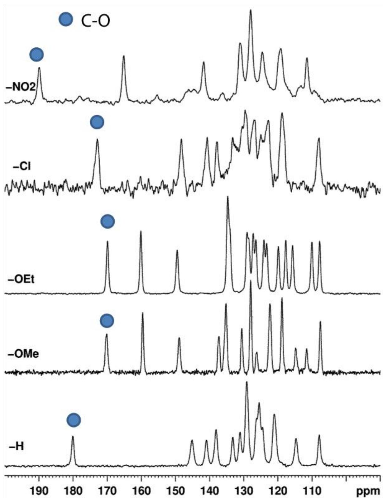
S4.3.  $^{13}\text{C}\{\text{H}\}$ CPMAS NMR spectrum of 3a
