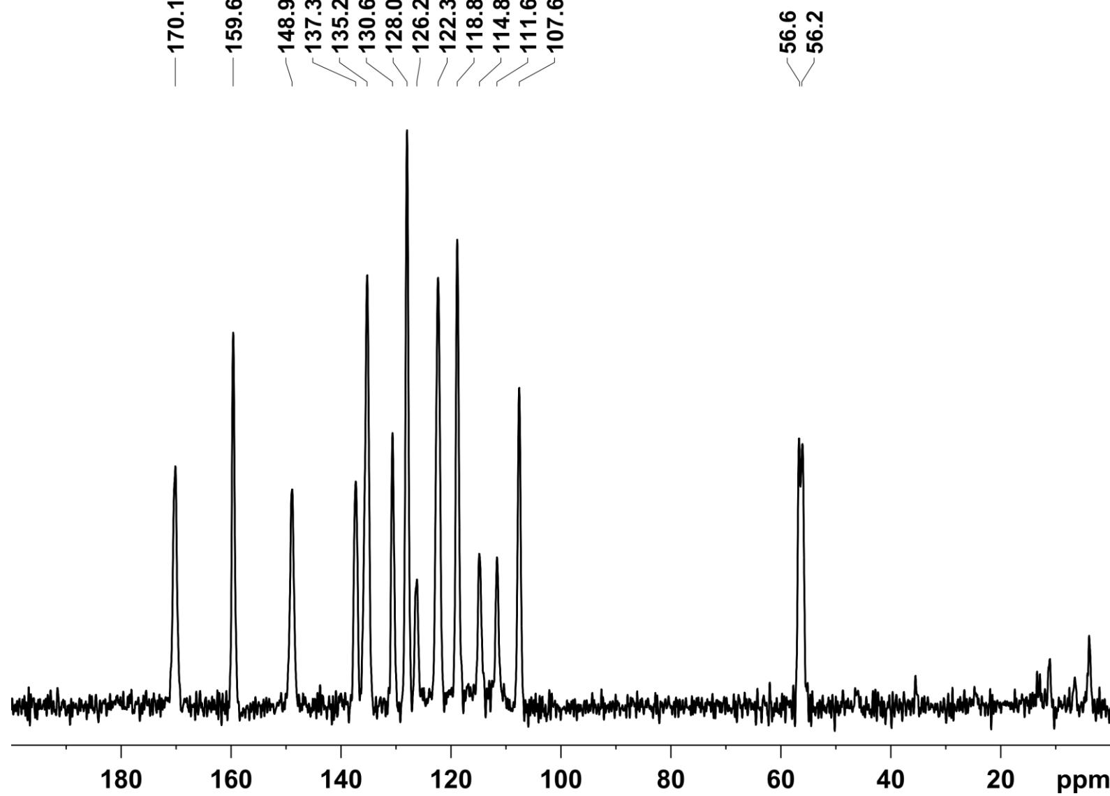
**S4.11. Extension of  $^{13}\text{C}\{^1\text{H}\}$ CPMAS NMR spectrum of 3e**
