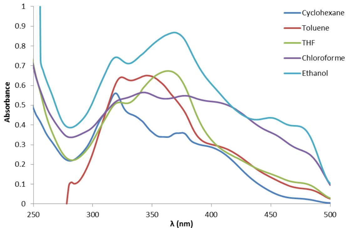
**Fig. S1** UV-VIS Spectra of **3a** in different solvents
