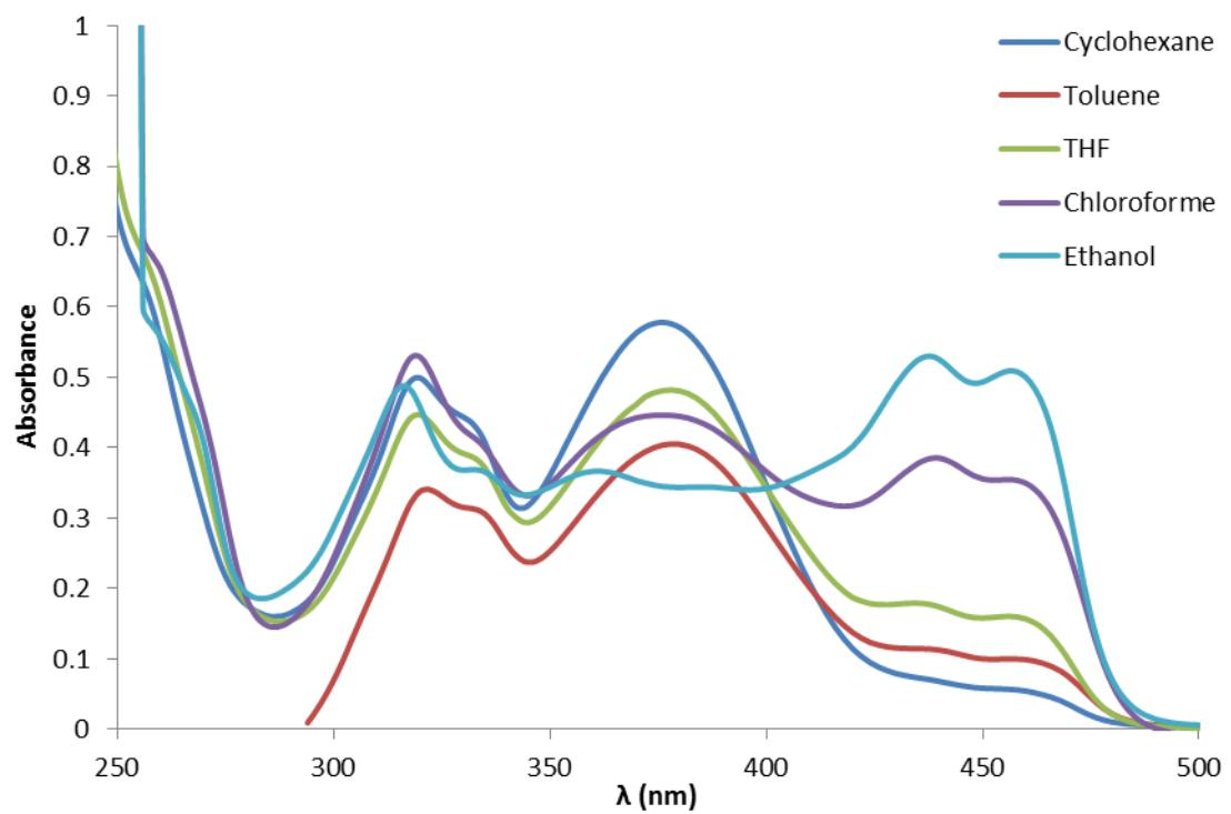
**Fig. S3** UV-VIS Spectra of **3c** in different solvents
