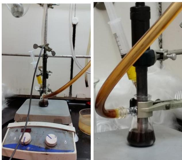
**Figure S1.** A dissolved oxygen probe monitors a stirred suspension of birnessite before and after injection of N<sub>2</sub>-sparged ceric ammonium nitrate via syringe. The apparatus is protected from air-O<sub>2</sub> by flowing nitrogen into the side-arm of the flask, which exits through the top.
