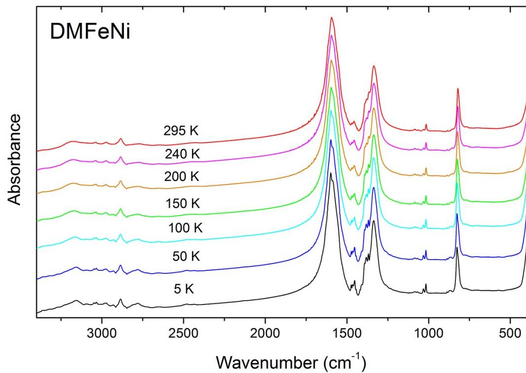
Figure S4. IR spectra of DMFeNi recorded at various temperatures.
