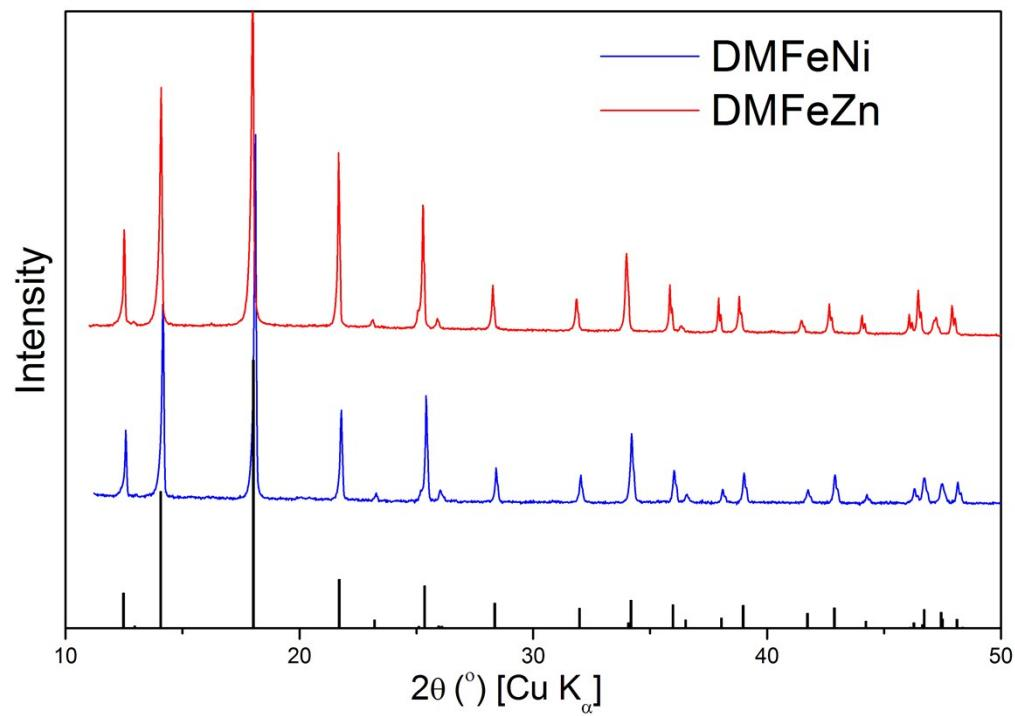
Figure S1. XRD patterns for DMFeNi and DMFeZn. Black bars at the bottom show position and relative intensity of DMFeNi diffraction patterns.
