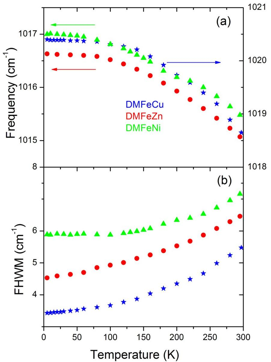
Figure S8. (a) Temperature dependence of the  $v_{\text{as}}(\text{CNC})$  IR frequencies and (b) the corresponding FWHM values for DMFeZn, DMFeNi and DMFeCu.
