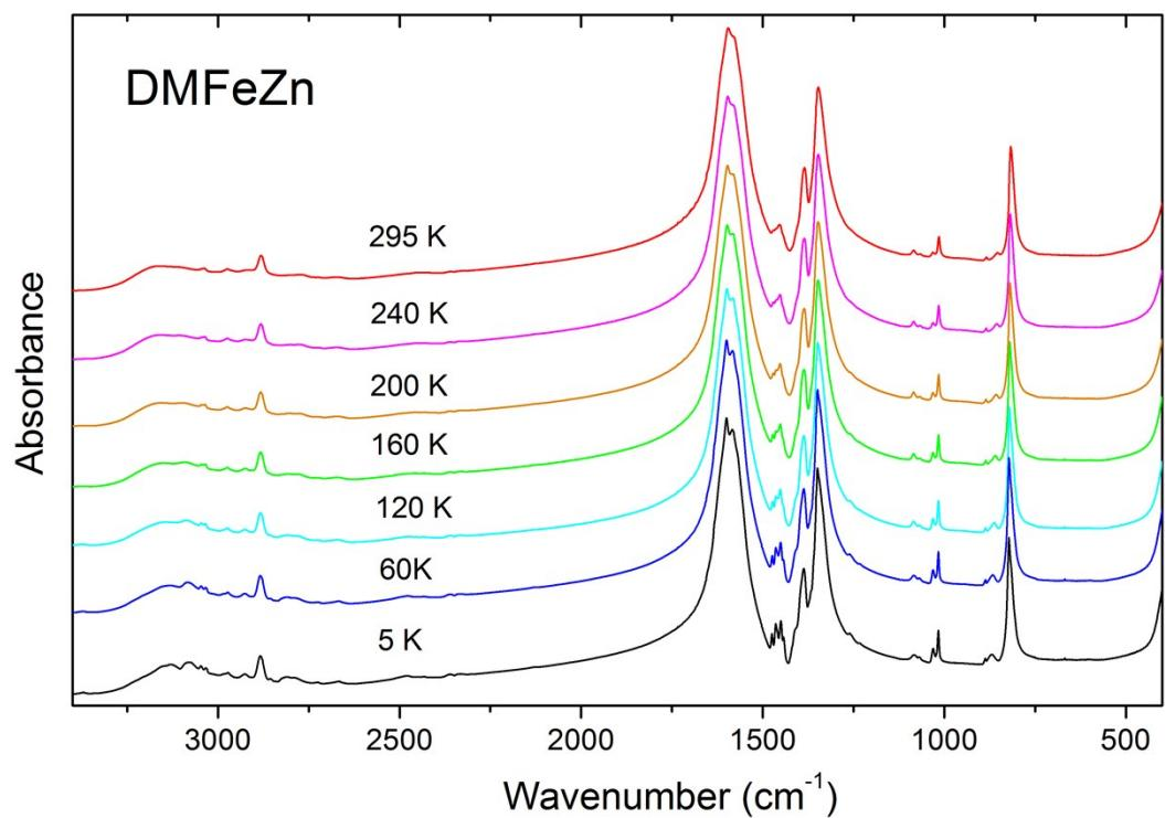
Figure S5. IR spectra of DMFeZn recorded at various temperatures.
