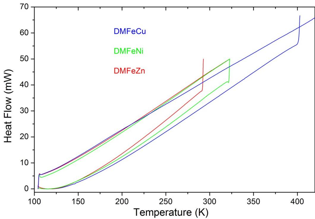
Figure S3. DSC traces for DMFeZn, DMFeNi and DMFeCu.
