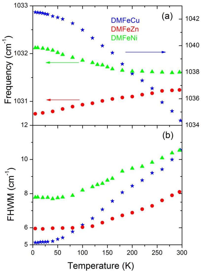
Figure S7. (a) Temperature dependence of the  $\rho(\text{CH}_3)$  IR frequencies and (b) the corresponding FWHM values for DMFeZn, DMFeNi and DMFeCu. The change of frequency is about 8 times larger for DMFeCu than DMFeZn and DMFeNi. DMFeCu also exhibit more pronounced change in FWHM.
