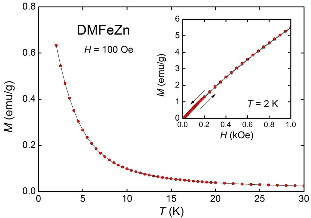
Figure S2. Magnetization of DMFeZn vs. temperature. Inset:  $M(H)$  measured upon increasing and decreasing field (open and closed symbols, respectively). Solid lines and arrows serve as guides for the eye.
