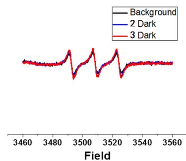
**Figure S3.** EPR signals of air-saturated  $\text{CH}_3\text{CN}$  solutions of TEMP (1 mM) alone (background) and in the presence of **2** or **3** (10  $\mu\text{M}$ ) in the dark.
