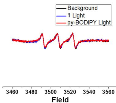
**Figure S2.** EPR signals obtained upon irradiation of air-saturated  $\text{CH}_3\text{CN}$  solutions of TEMP (1 mM) alone (background) and in the presence of **1** or py-BODIPY (10  $\mu\text{M}$ ) with 532 nm pulsed laser.
