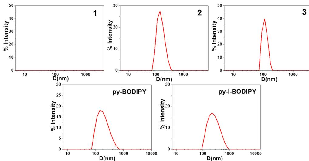
**Figure S1.** Hydrodynamic diameter distributions of **1**, **2**, **3**, py-BODIPY and py-I-BODIPY (5  $\mu\text{M}$ ) in PBS (pH = 7.4, 5 mM)/DMSO (8:1) solutions at room temperature.
