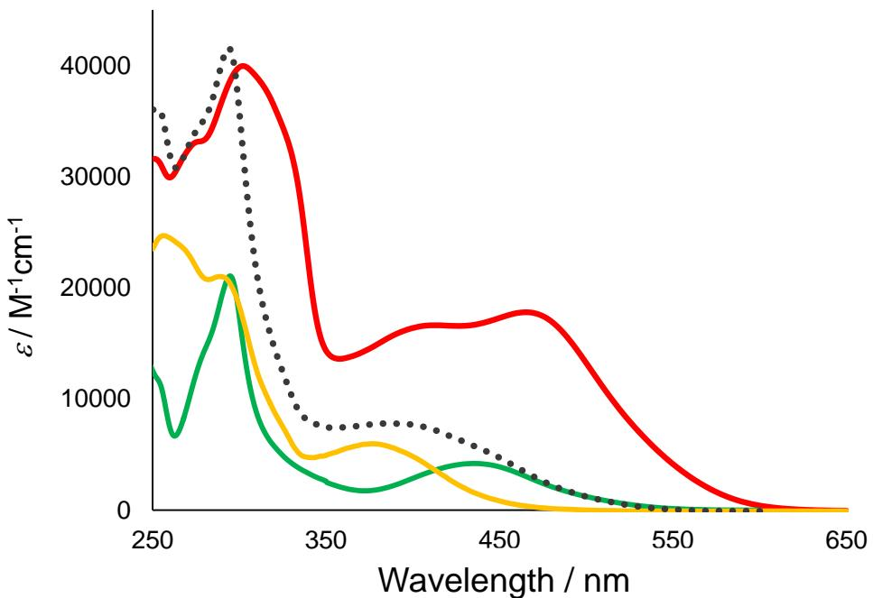
**Fig. S2** UV-Vis absorption spectra of  $[\text{Re(OEt)Re(Et)}]^{2+}$  (red),  $[\text{Re(C=C,OEt)}]^+$  (yellow),  $[\text{Re(bpy)(CO)}_2(\text{PET}_3)_2]^+$  (green) measured in MeCN and 1:1 summation spectrum of  $[\text{Re(C=C,OEt)}]^+$  and  $[\text{Re(bpy)(CO)}_2(\text{PET}_3)_2]^+$  (dotted line).
