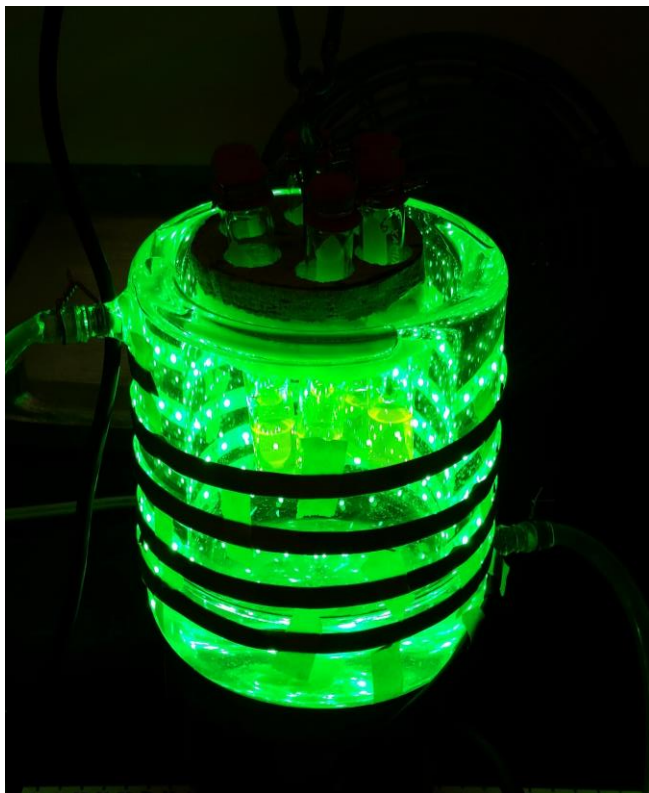
Figure S10. Image of the photocatalytic reaction vessel. An LED ribbon is attached to the outside of a jacketed beaker that is cooled to 20°C. The samples are in test tubes that are rotated inside of the beaker.
