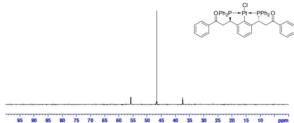
**Figure 2.**  $^{31}\text{P}\{^1\text{H}\}$  NMR spectrum of complex 6a.
