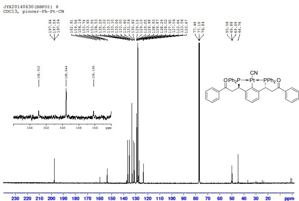
**Figure 21.** <sup>13</sup>C NMR spectrum of complex 6c.
