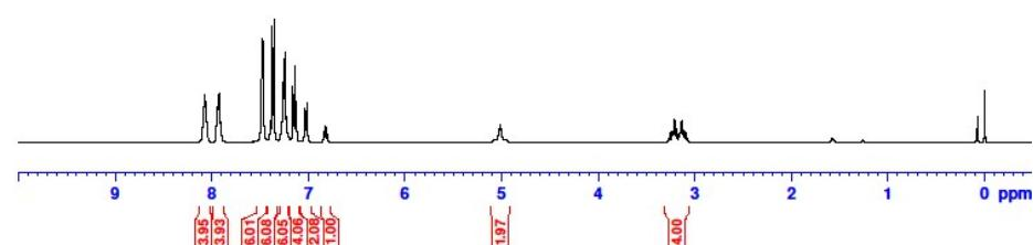
**Figure 1.**  $^1\text{H}$  NMR spectrum of complex 6a.
