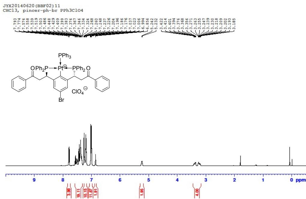
**Figure 16.**  $^1\text{H}$  NMR spectrum of complex **8b**.
