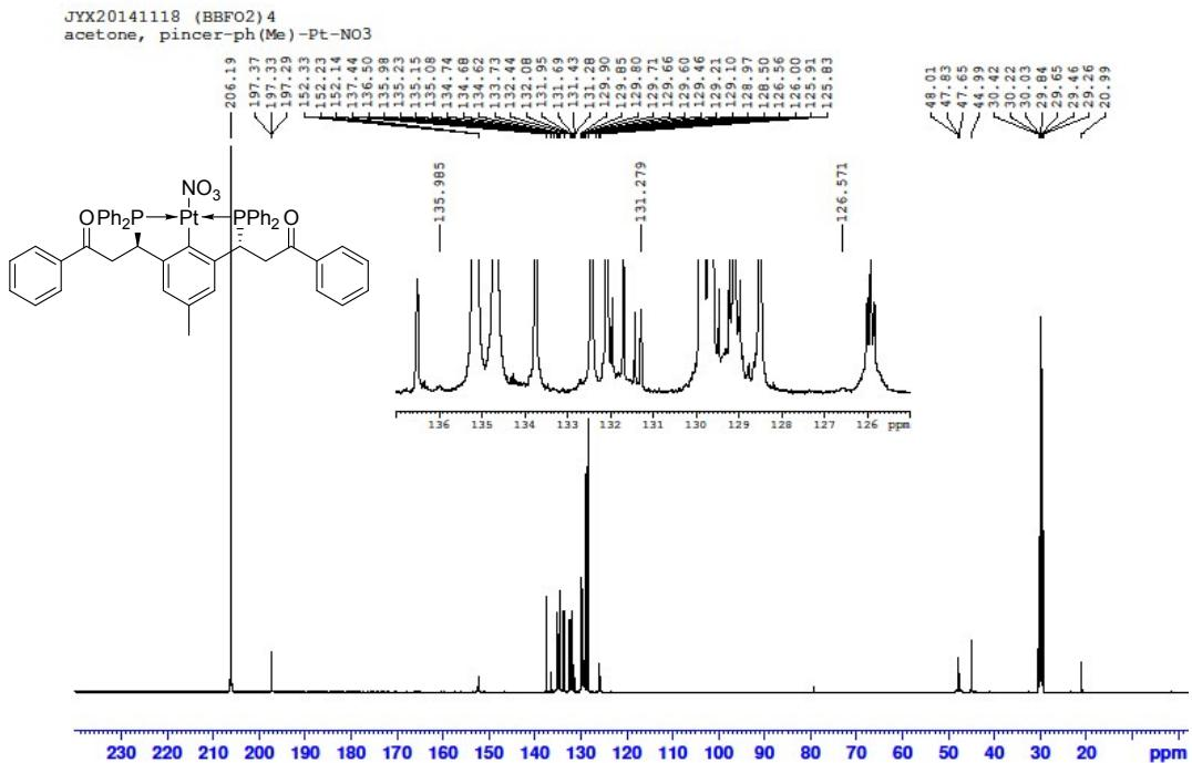
**Figure 33.**  $^{13}\text{C}$  NMR spectrum of complex **7d**.
