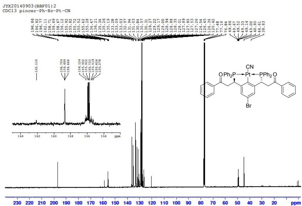
**Figure 27.**  $^{13}\text{C}$  NMR spectrum of complex **8c**.
