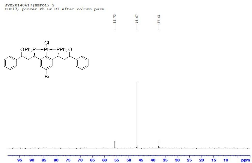
**Figure 8.**  $^{31}\text{P}\{^1\text{H}\}$  NMR spectrum of complex **8a**.
