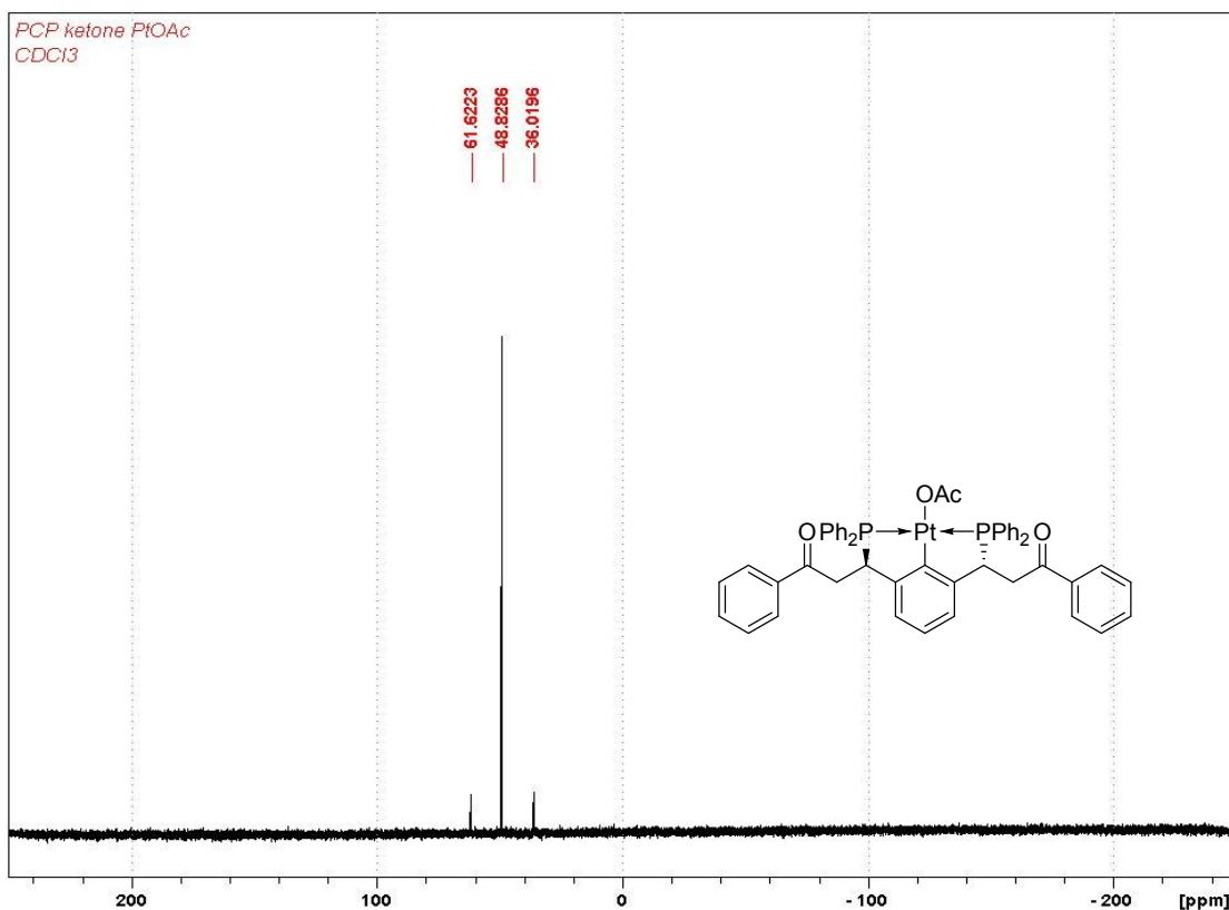
**Figure 40.**  $^{31}\text{P}\{\text{H}\}$  NMR spectrum of complex 6e.
