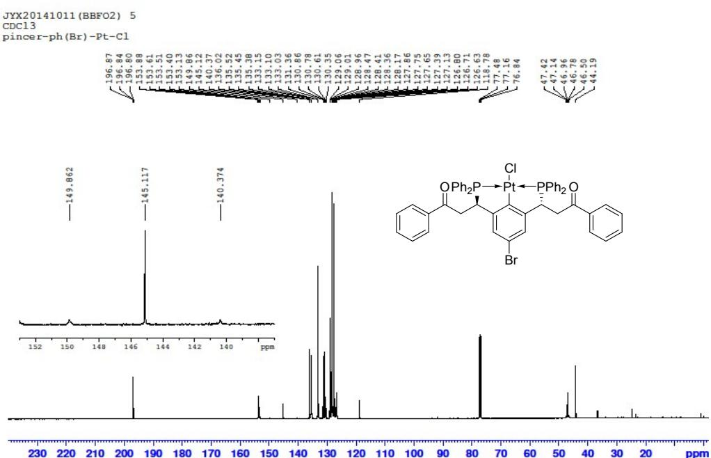
Figure 9. <sup>13</sup>C NMR spectrum of complex 8a.
