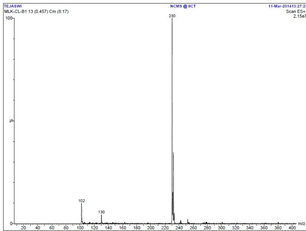
**Figure S10.** ESI-MS spectrum of 2-(4-chloropyridin-2-yl)-1H-benzimidazole.
