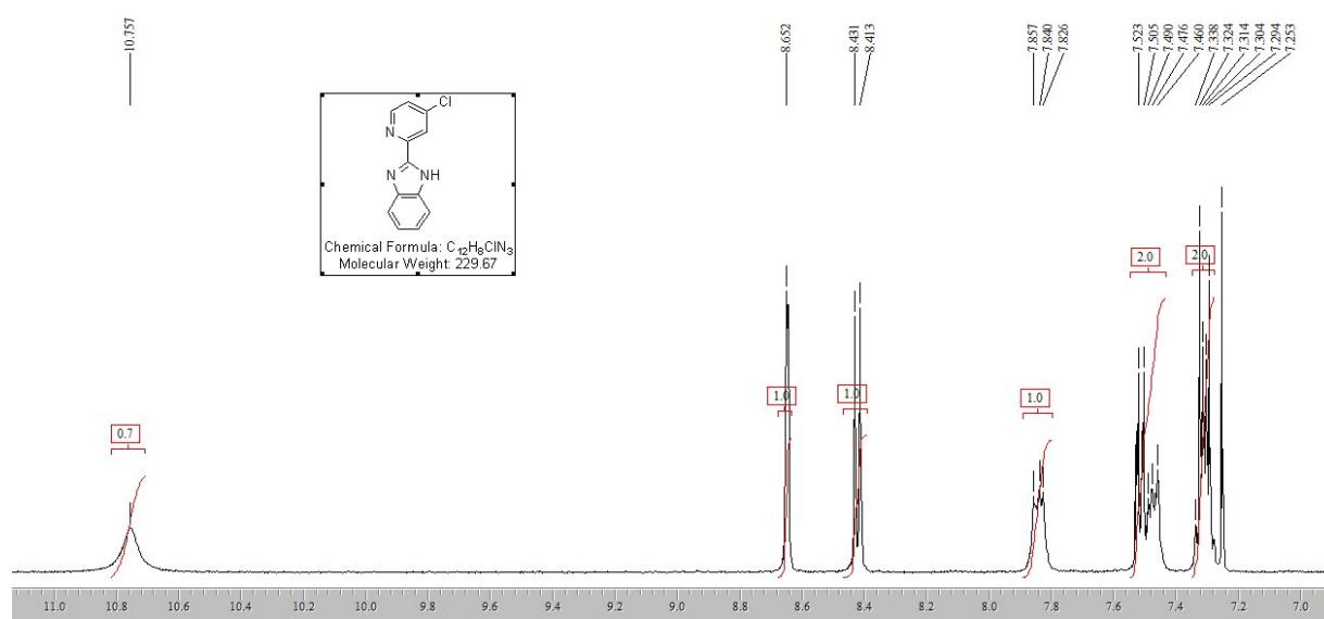
**Figure S9.**  $^1\text{H}$ NMR spectrum of 2-(4-chloropyridin-2-yl)-1H-benzimidazole.
