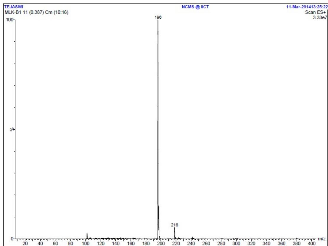
**Figure S2.** ESI-MS spectrum of 2-(pyridin-2-yl)-1H-benzimidazole.
