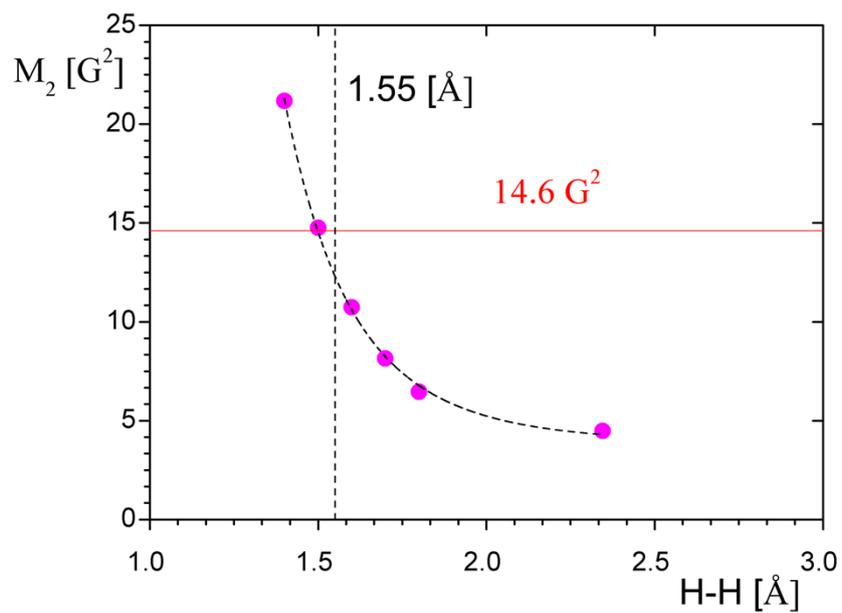
**Figure S7.** Relationship between H-H distance and calculated value of  $M_2$ .
