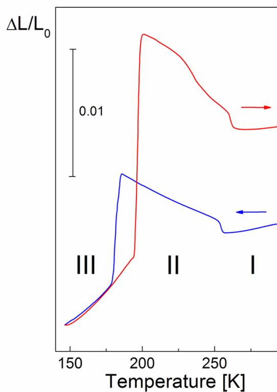
**Figure S1.** The linear thermal expansion along the *b*-axis of PI upon heating and cooling scans.
