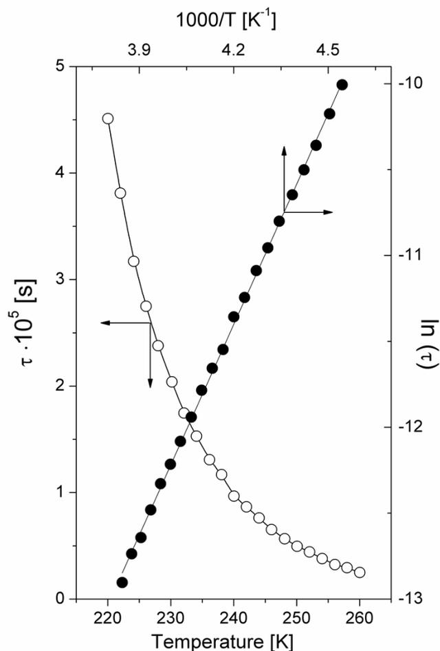
**Figure S6.** Temperature dependence of  $\tau$  versus temperature and  $\ln(\tau)$  versus reciprocal temperature for PI.
