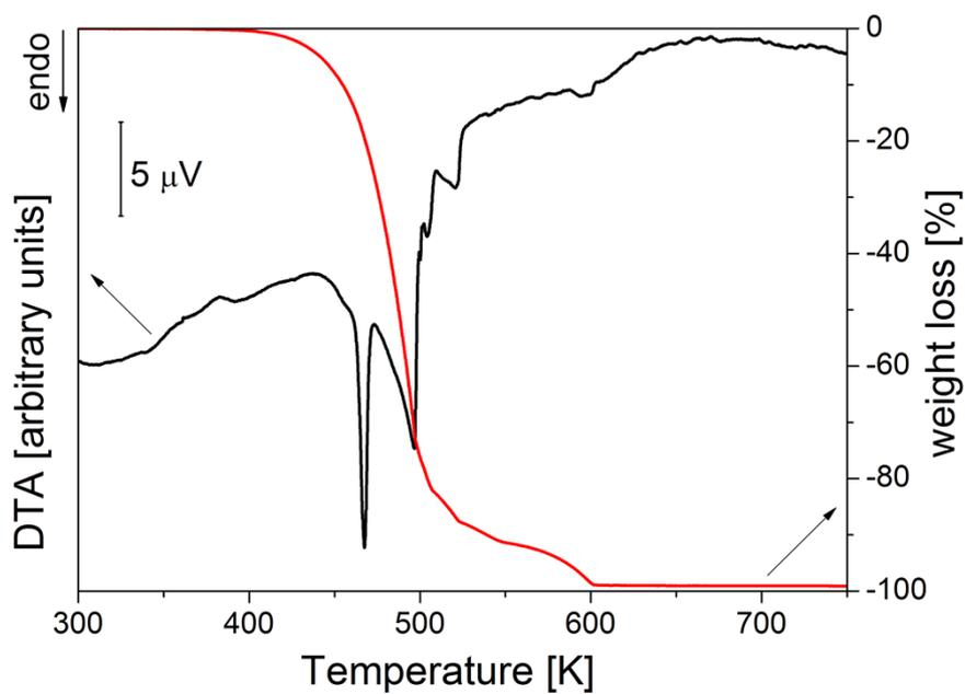
**Figure S2.** Simultaneous thermogravimetric analysis and thermal analysis scan (with temperature rate of  $2 \text{ K min}^{-1}$ , sample mass  $m=12.20 \text{ mg}$ ).
