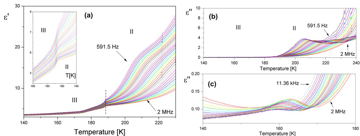
**Figure S4.** The temperature dependence of the (a) real and (b, c) imaginary part of complex electric permittivity for the polycrystalline sample of PI.
