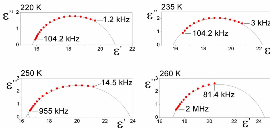
**Figure S5.** Cole-Cole plots of  $\epsilon''$  versus  $\epsilon'$  at selected temperatures showing the relaxation nature of the dielectric dispersion for PI.
