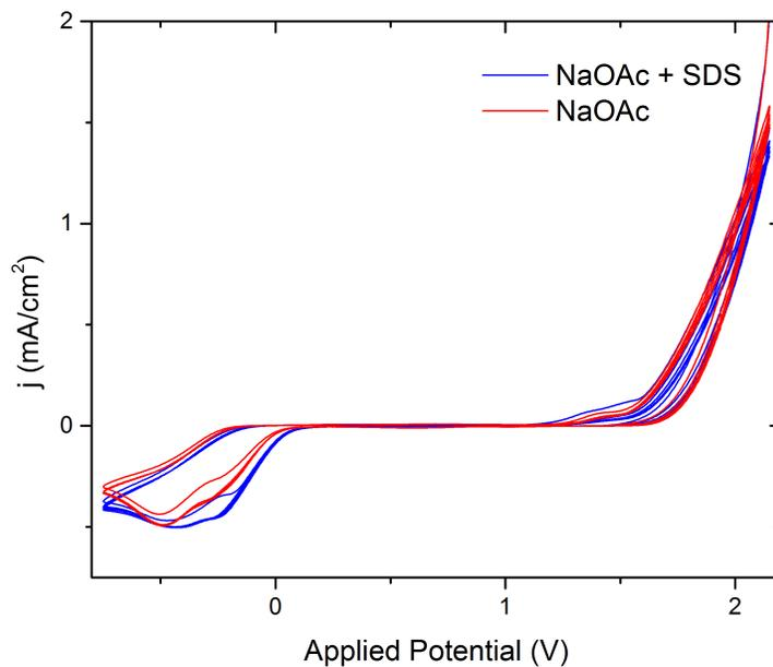
**Figure S2.** CVs of blank FTO in 25 mM sodium acetate (99.0%, Sigma Aldrich) with and without SDS. Voltage is reported vs. NHE.
