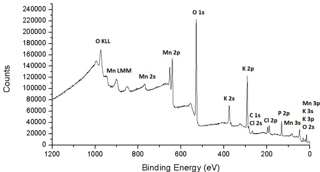
**Figure S7.** XPS spectrum of a sample with SDS after 24 hours of electrolysis. Phosphorus peak indicates the incorporation of the element from the phosphate buffer as shown in EDX (Figs. S10-S11).
