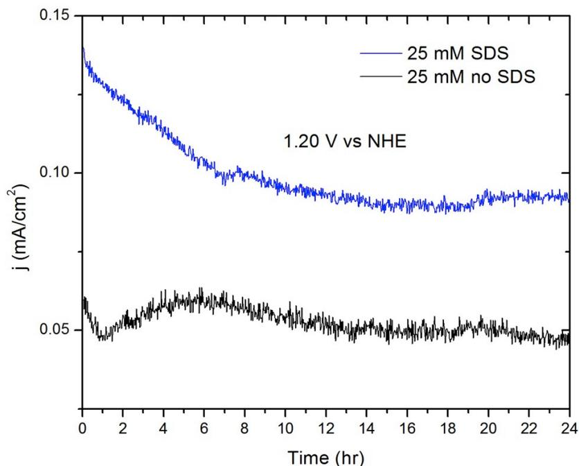
**Figure S3.** Stability of catalysts with and without SDS.
