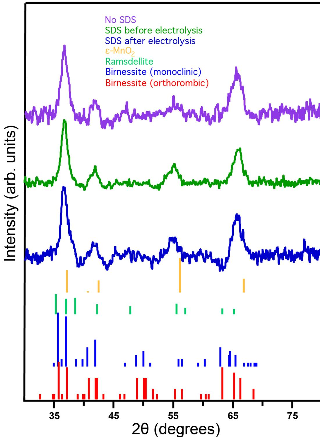
**Figure S9.** XRD data for 25 mM Mn<sup>2+</sup> with and without SDS as well as before and after the electrolysis. Vertical bars present peaks of crystal structures from JCPDS database ( $\epsilon$ -MnO<sub>2</sub>: 30-0820; ramsdellite: 43-1455; monoclinic birnessite: 43-1456; orthorombic birnessite: 23-1046).
