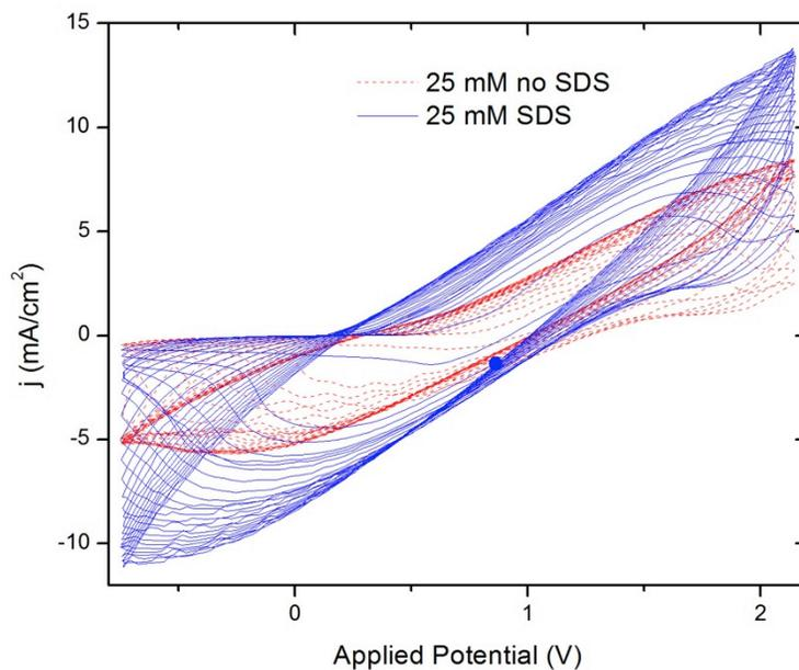
**Figure S1.** Deposition of 25 mM MnO<sub>2</sub> with and without SDS. Voltage is reported vs. NHE.
