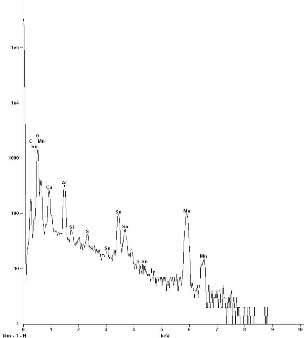
**Figure S10.** SEM-EDX spectrum of a sample of the Mn catalyst after deposition but prior to any water-oxidation catalysis. S is present due to SDS. Sn, Si, Cu, and Al signals arise from the FTO-coated glass substrate and sample holder.
