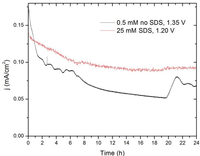
**Figure S5.** 24 h stability tests comparing the catalyst deposited using conditions from Protocol C in ref. 35 of the manuscript (0.5 mM Mn<sup>2+</sup>, no SDS, black) at 1.35 V vs. NHE to a sample of 25 mM SDS (red) at 1.20 V vs. NHE.
