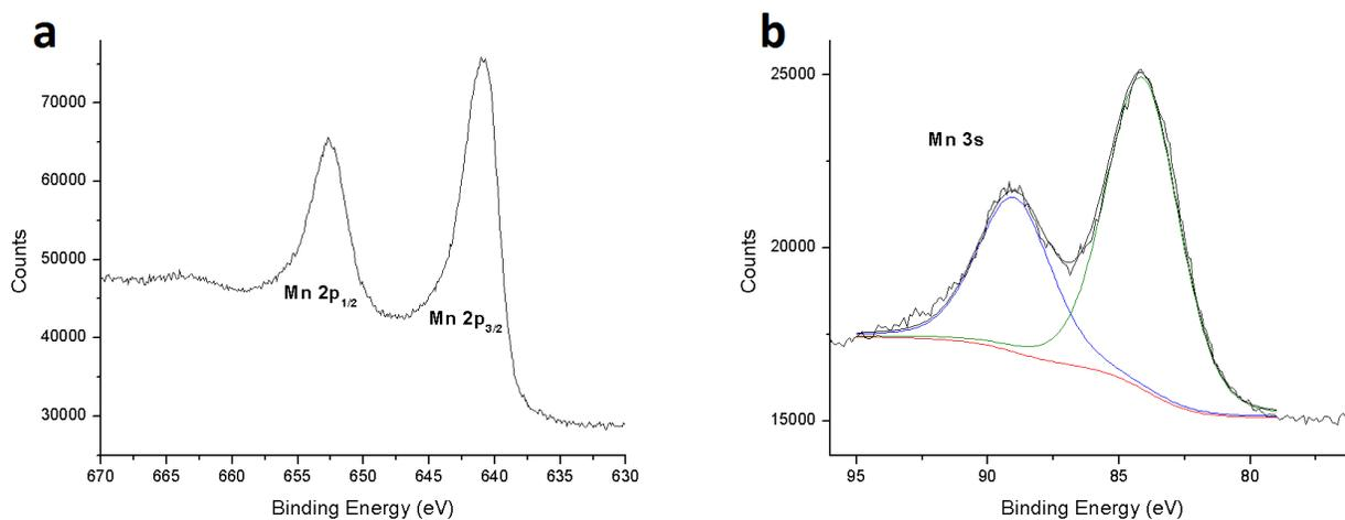
**Figure S8.** XPS spectra of a sample with SDS after 24 hours of electrolysis. (a) Mn 2p region showing the Mn  $2p_{3/2,1/2}$  spin-orbit pair, with the Mn  $2p_{3/2}$  multiplet centered near 641 eV. (b) Mn 3s region; the magnitude of peak splitting is a reliable indicator of Mn oxidation state. The energy difference between the multiplets (shown in green and blue, with Shirley background in red) is approximately 4.8 eV, diagnostic of an oxide containing predominantly Mn<sup>IV</sup>.
