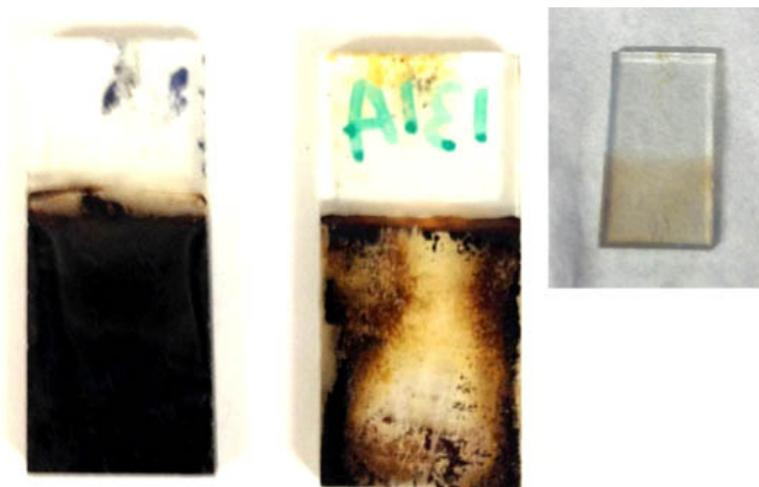
**Figure S4.** After 24 h of electrolysis, the slide with SDS (left) was visually not affected, while the slide with no SDS (middle) lost a significant amount of material. Right: for comparison, a slide containing a much more transparent film of a manganese oxide water-oxidation catalyst, that was prepared using protocol C from ref. 35 in the manuscript (deposited from 0.5 mM Mn acetate in deionized water), after 24 h of electrolysis.
