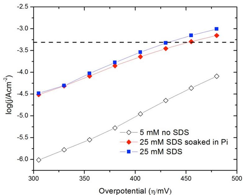
**Figure S12.** Tafel plots of catalyst deposited with and without SDS, at different concentrations, and with/without 36-hour-long pre-soaking in phosphate. Dashed line marks  $0.5 \text{ mA/cm}^2$ .
