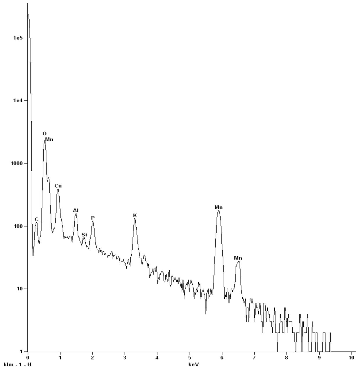
**Figure S11.** SEM-EDX spectrum of a sample after 24 h of electrolysis. S is no longer present, but K and P have been incorporated into the film. Si, Al, and Cu signals arise from the sample holder.
