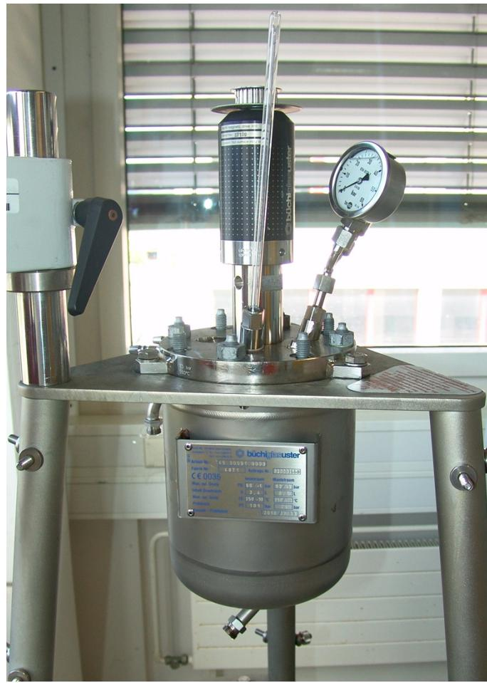
**Fig. S4.** The picture of the 3 L of autoclave used in large-scale MIL-101(Cr) syntheses.
