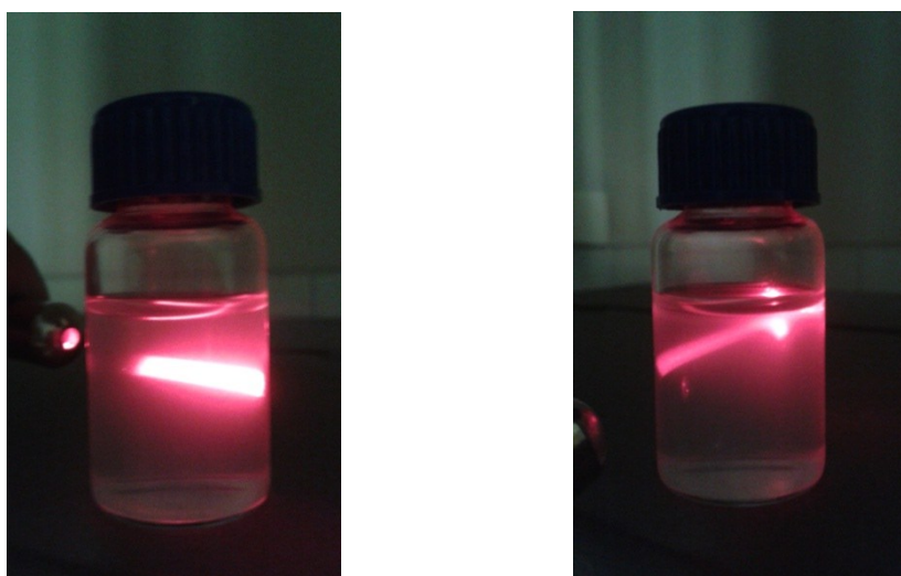
Figure 9S. The Tyndall effect of aqueous dispersion of sample 1 . Stable and homogeneous dispersions of these compounds were obtained by stirring the sample in a deionized water solution, that contained a small amount (4/5 drops) of propilamine 0.2 M, and then ultrasonicated for 10 minutes; Tyndall Effect was established on compound 1 ; all other two compounds showed similar behavior.
