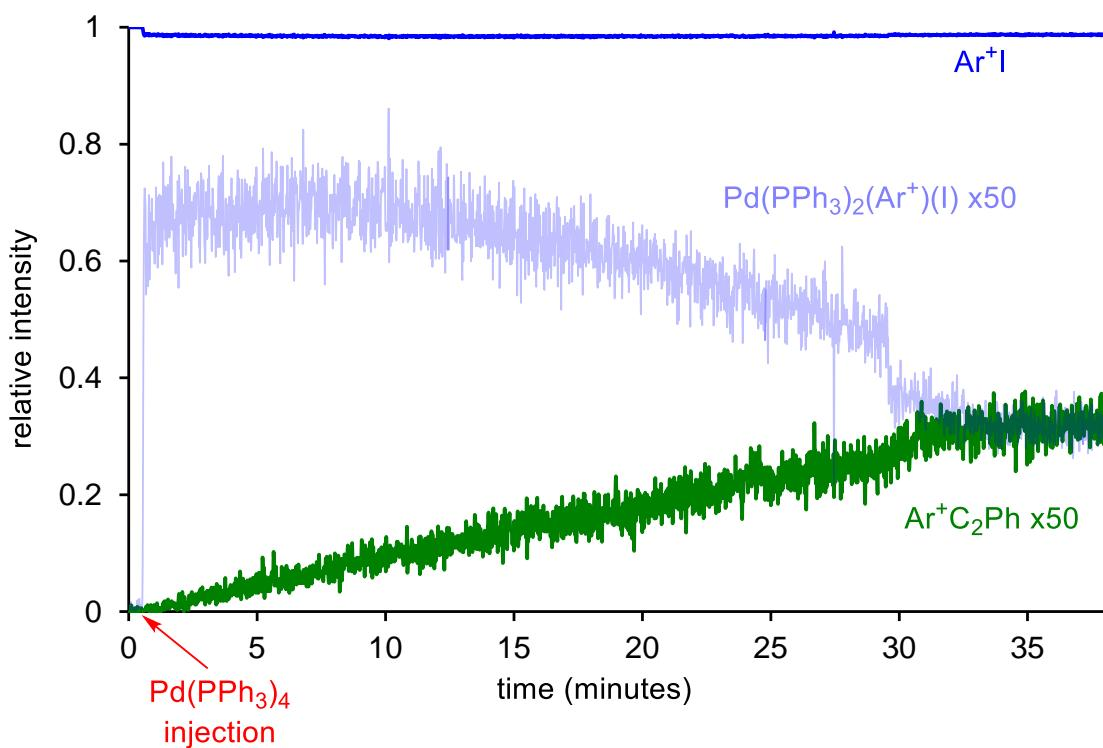
Figure SI6: ESI(+)–MS over time of a reaction performed in the absence of base. The intensities of all observed key species bearing the charged tag are shown, with the intensities of the product and  $\text{Pd}(\text{PPh}_3)_2(\text{Ar}^+)(\text{I})$  have been multiplied by 50 for illustrative purposes.
