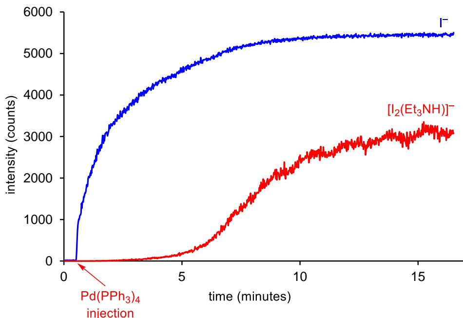
Figure SI11a. ESI(-)-MS intensity data for reaction involving neutral substrates. Release of the iodide and  $[\text{I}_2(\text{Et}_3\text{NH})]^-$  clearly indicates the reaction is proceeding.
