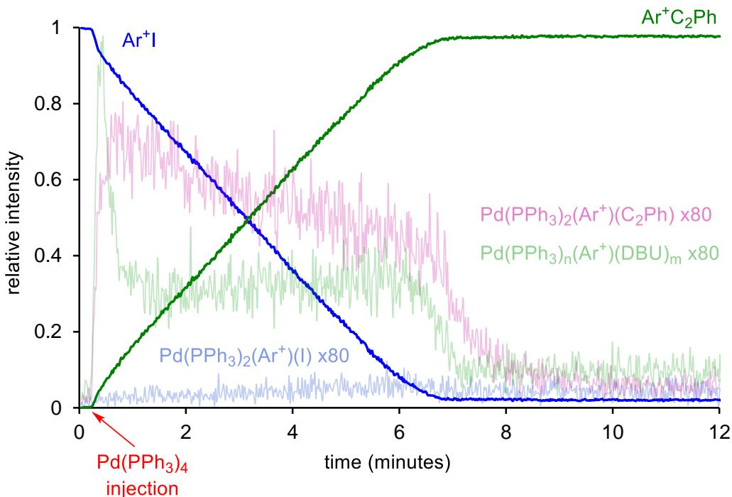
Figure SI9: ESI(+)‑MS of reaction with “standard conditions “and six equivalents of phenylacetylene ( $\text{Ar}^+ = [\text{C}_6\text{H}_4\text{CH}_2\text{PPh}_3]^+$ ). The intensities of the palladium intermediates are multiplied by 80 for illustrative purposes.
