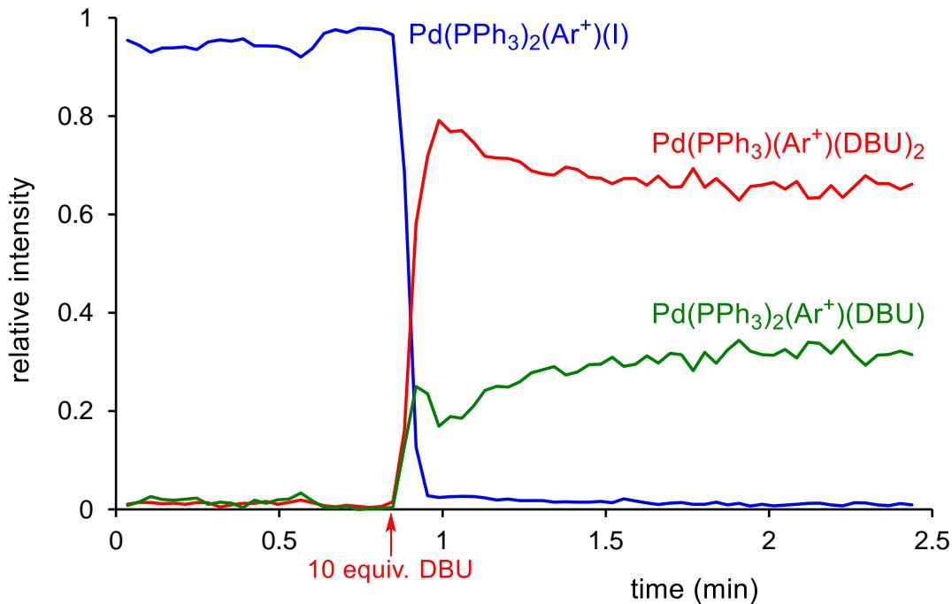
Figure SI5: Addition of ten equivalents of DBU at 0.8 minutes to the mixture of charged  $\text{Ar}^+\text{I}$  (0.5 mM) and catalyst (6 mol %) at reflux in MeOH (10 mL). Ar =  $[p\text{-C}_6\text{H}_4\text{CH}_2\text{PPh}_3]^+$ , DBU = 1,8-diazabicyclo[5.4.0]undec-7-ene. Traces are ESI(+) - MS data normalized to the total ion current.
