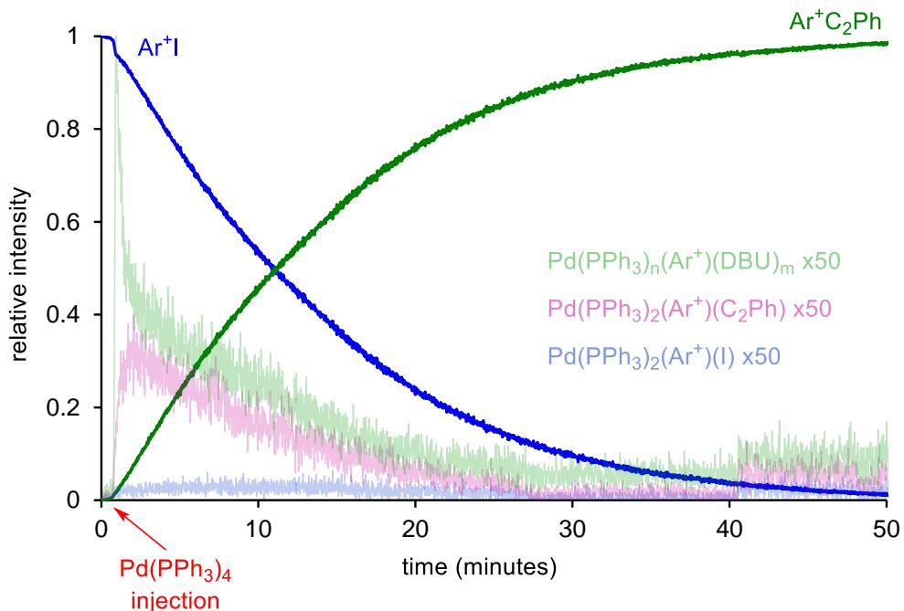
Figure SI10: ESI(+)-MS of reaction with “standard conditions” and three equivalents of biphenylacetylene ( $\text{Ar}^+ = [\text{C}_6\text{H}_4\text{CH}_2\text{PPh}_3]^+$ ). The intensities of the palladium intermediates are multiplied by 50 for illustrative purposes.
