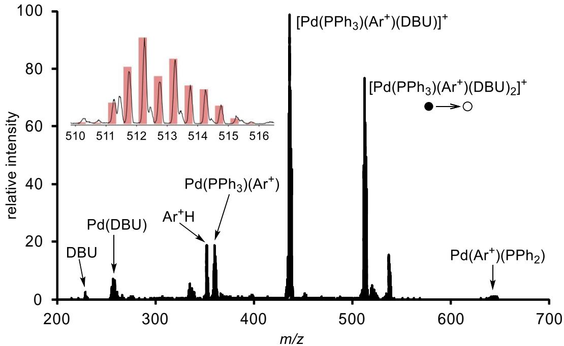
Figure SI4: ESI(+) -MS/MS of  $[\text{Pd}(\text{PPh}_3)(\text{Ar}^+)(\text{DBU})_2]^+$  (doubly charged,  $m/z$  512.3). Inset: actual spectrum (black) and predicted isotope pattern (red bars) for  $[\text{Pd}(\text{PPh}_3)(\text{Ar}^+)(\text{DBU})_2]^+$ . The most abundant fragment is obtained by the loss of one DBU (doubly charged,  $m/z$  436.2). Also the loss of the second DBU (doubly charged,  $m/z$  360.1)
