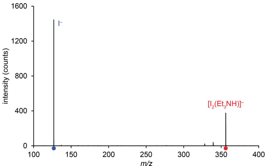
Figure SI11b. ESI(-)-MS intensity data for reaction involving neutral substrates. Release of the iodide and  $[I_2(Et_3NH)]^-$  clearly indicates the reaction is proceeding. The above spectrum is a snapshot from the experiment conducted in SI11a, at the 10 minute mark.
