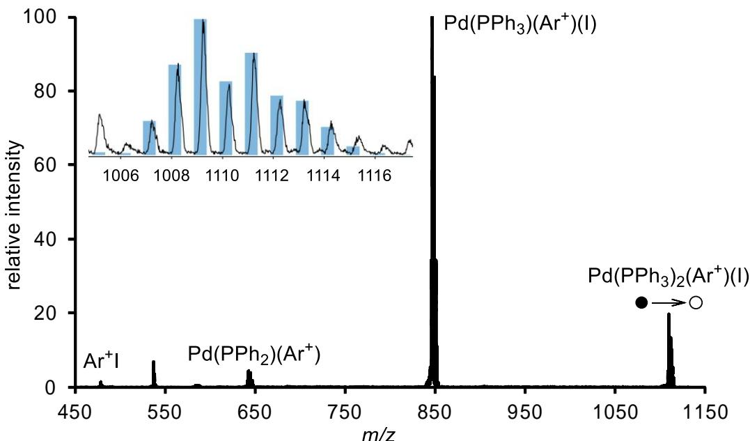
Figure SI1: ESI(+) - MS/MS of  $\text{Pd}(\text{PPh}_3)_2(\text{Ar}^+)(\text{I})$  ( $m/z$  1109.4). Fragmentation occurs via loss of triphenylphosphine not loss of  $\text{Ar}^+\text{I}$  indicating that elimination of  $\text{Ar}^+\text{I}$  is not facile. Inset: actual spectrum (black) and predicted isotope pattern (blue bars) for  $\text{Pd}(\text{PPh}_3)_2(\text{Ar}^+)(\text{I})$ .
