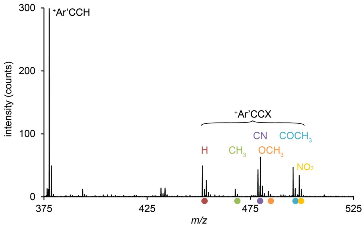
Figure SI13. Snapshot from  $t = 10$  minutes of the multisubstrate screening reaction shown in Figure 4.  $\text{X} = p\text{-C}_6\text{H}_4\text{Y}$  where  $\text{Y} = \text{H}, \text{CH}_3, \text{CN}, \text{OCH}_3, \text{COCH}_3$  and  $\text{NO}_2$
