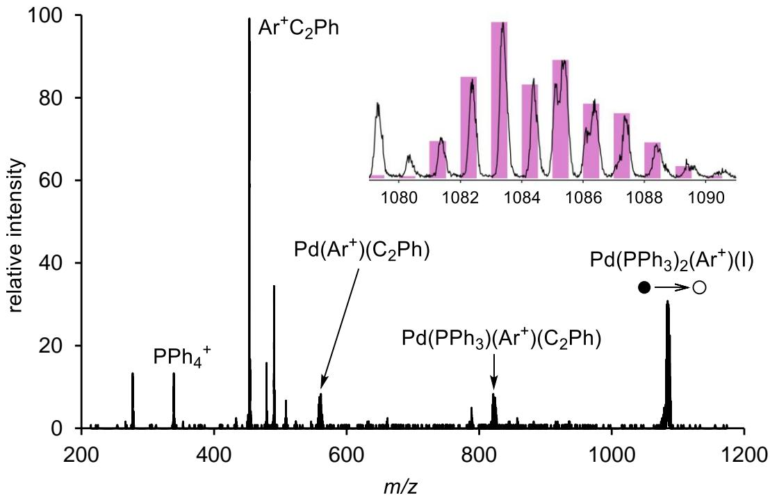
Figure SI2: ESI(+)-MS/MS of  $\text{Pd}(\text{PPh}_3)_2(\text{Ar}^+)(\text{C}_2\text{Ph})$  ( $m/z$  1083.4). Inset: actual spectrum (black) and predicted isotope pattern (pink bars) for  $\text{Pd}(\text{PPh}_3)_2(\text{Ar}^+)(\text{C}_2\text{Ph})$ .  $\text{ArC}_2\text{Ph}$  is the most abundant fragment which denotes that reductive elimination of the product is favourable. Loss of one and two triphenylphosphine is observed. Some peaks were not assigned.
