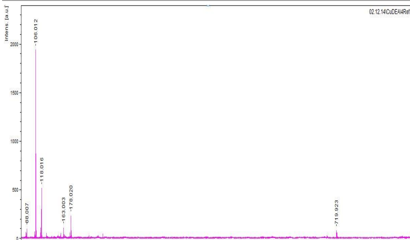
Fig. S3. MALDI (Matrix Assisted Laser Desorption/Ionization) mass spectrum of [\text{Cu}^{2+}\text{DH}_2(\text{DH}^-)][(\text{DH}_2)_4\text{H}^+](\text{OTf}^-)_2 preparation
