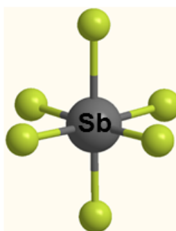
Fig. S7 Optimized structure of \text{SbF}_6^- . Selected bond distance ( \text{\AA} ) and angle (deg): Sb-F = 1.88 (av.), F-Sb-F = 90.0 (av.).
