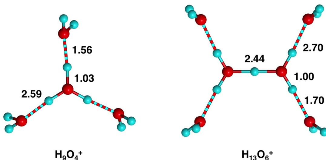
Fig S2. Structures of  $\text{H}_9\text{O}_4^+$  and  $\text{H}_{13}\text{O}_6^+$  with distances ( $\text{\AA}$ ) calculated with DMol/BLYP.
