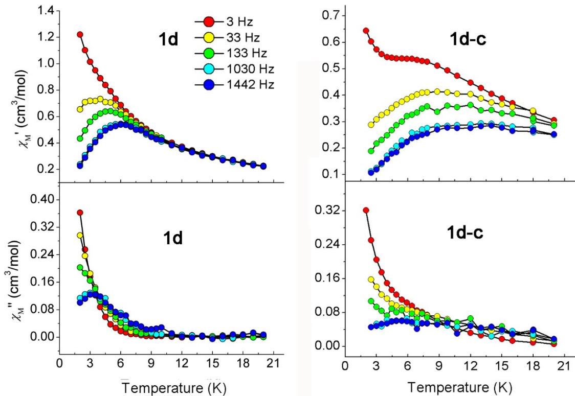
**Fig. S10** Temperature dependent in-phase ( $\chi'_M$ ) (up) and out-of-phase ( $\chi''_M$ ) (down) ac susceptibility components at different frequencies for the diluted sample **1d** (with Dy/Y = 1/440) and the corresponding calcined sample **1d-c** with 500 Oe applied dc field. The solid lines join the data points.
