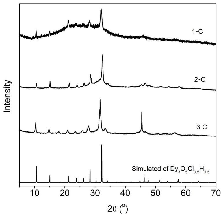
**Fig. S4** Experimental PXRD for **1-c**, **2-c** and **3-c** and simulated PXRD pattern of **1-c**.
