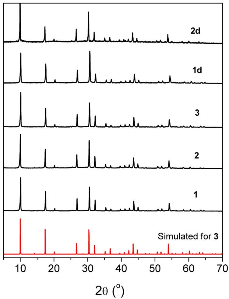
**Fig. S2** Experimental PXRD patterns of **1**, **2**, **3**, **1d** and **2d**, comparing with the simulated one for **3**.
