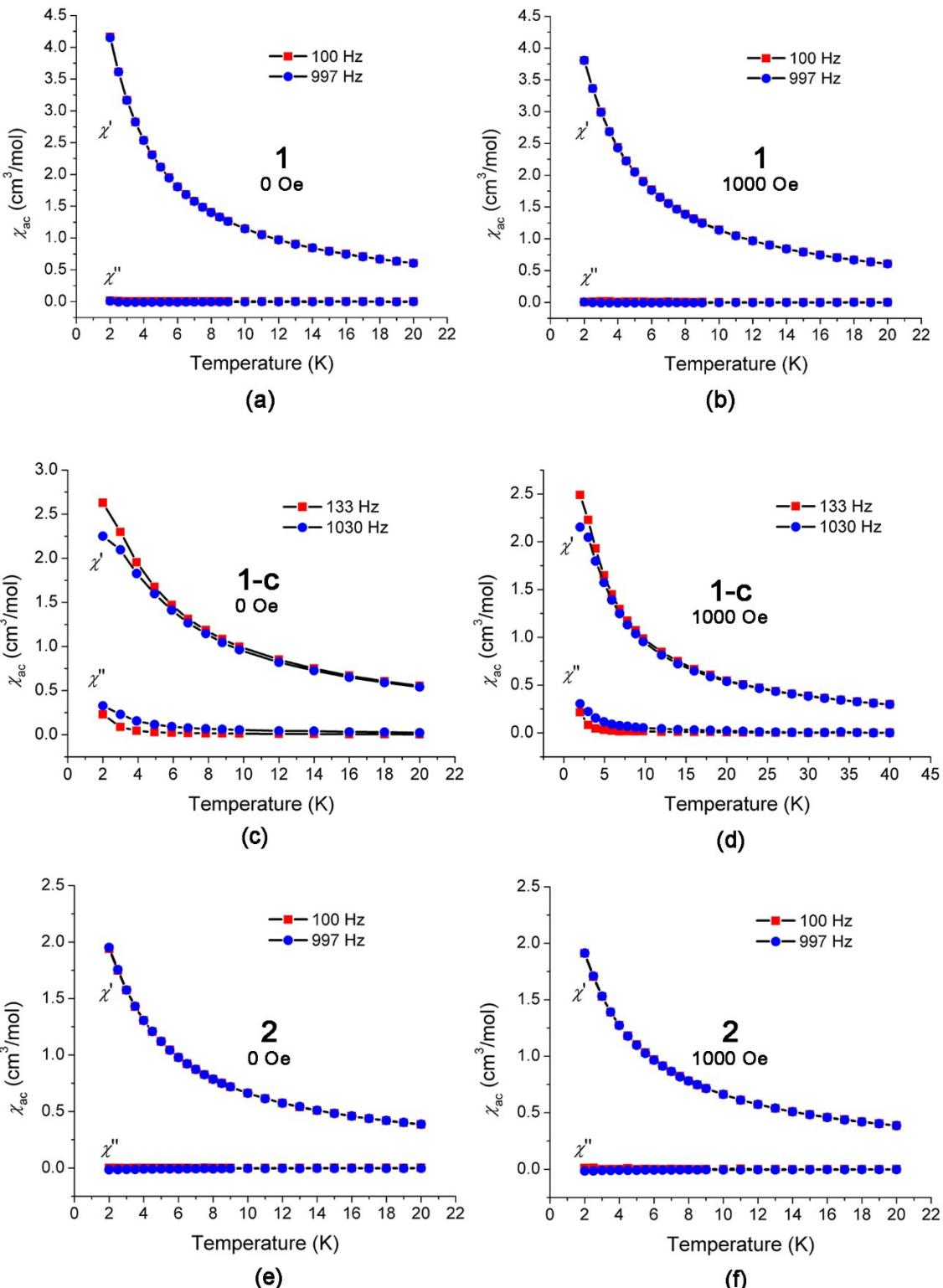
**Fig. S9** Temperature-dependent in-phase ( $\chi'_M$ ) (up) and out-of-phase ( $\chi''_M$ ) (down) ac susceptibility components at different frequencies for complex **1** ((a) and (b)), **1-c** ((c) and (d)) and **2** ((e) and (f)) with applied dc field of 0 Oe (left) and 1000 Oe (right). The solid lines join the data points.
