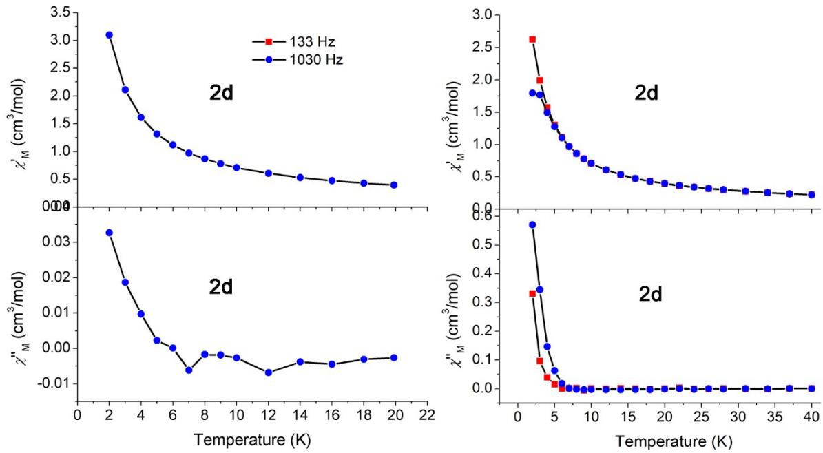
**Fig. S11** Temperature dependent in-phase ( $\chi'_M$ ) (up) and out-of-phase ( $\chi''_M$ ) (down) AC susceptibility components at different frequencies for the diluted sample **2d** (with Er/Y = 1/15) with applied DC field of 0 Oe (left) and 1000 Oe (right). The solid lines join the data points. Ac in the presence of a small external dc field of 1000 Oe show the presence of an out-of-phase signal,  $\chi''$ , for **2d** in contrast with **2**.
