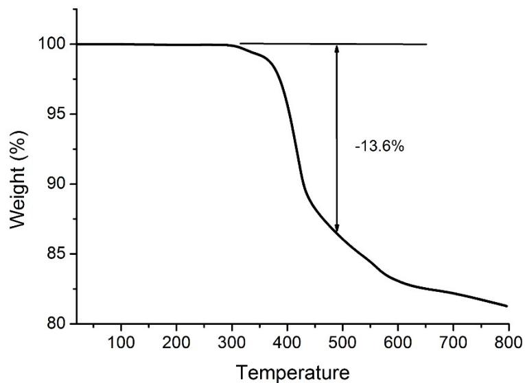
**Fig. S3** TGA curves of as-synthesized **1**.
