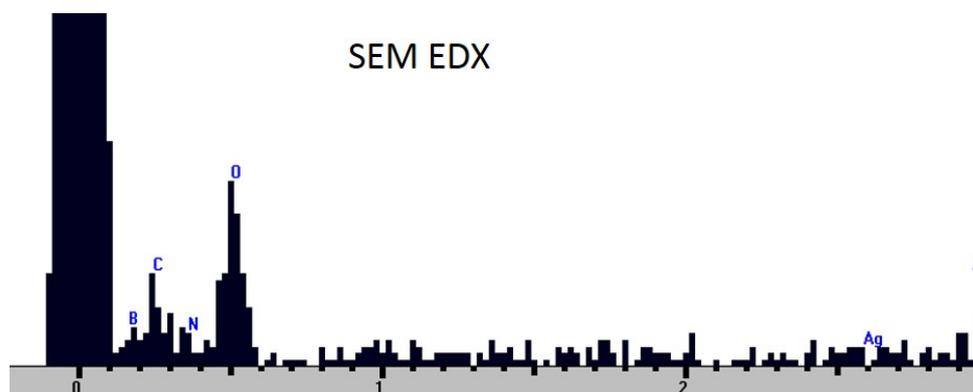
**Figure S4:** SEM-EDX analysis of amorphous BN-containing nanostructures grown from the pyrolysis (2 h, at 1000 °C under flow of N<sub>2</sub>) of **2** on Si-wafer.
