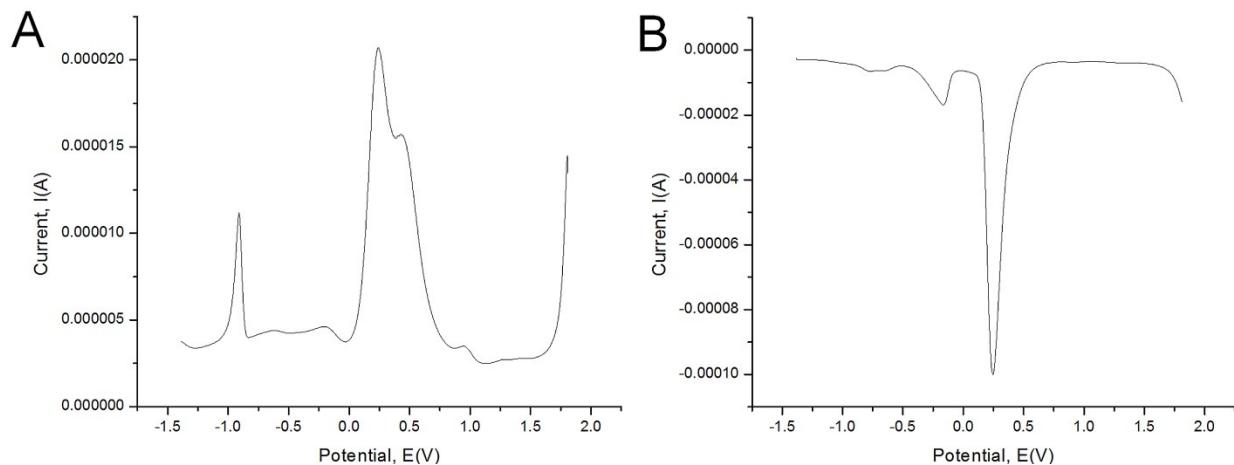
**Fig. S27.** Differential pulse voltammograms of  $[\text{Fe}(\text{dmise})_2(\text{CH}_3\text{CN})_2]\text{[OTf]}_2$  (**4**; 10 mM) in acetonitrile: A) negative mode and B) positive mode; potentials are reported vs. NHE.
