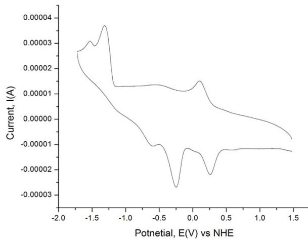
**Fig. S19.** Cyclic voltammogram for  $\text{FeCl}_2 \cdot 4\text{H}_2\text{O}$  (10 mM) in acetonitrile starting at 1.48 V.
