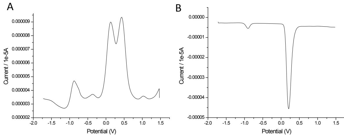
**Fig. S23.** Differential pulse voltammograms of ebis (10 mM) in acetonitrile: A) negative mode and B) positive mode; potentials are reported vs. NHE.
