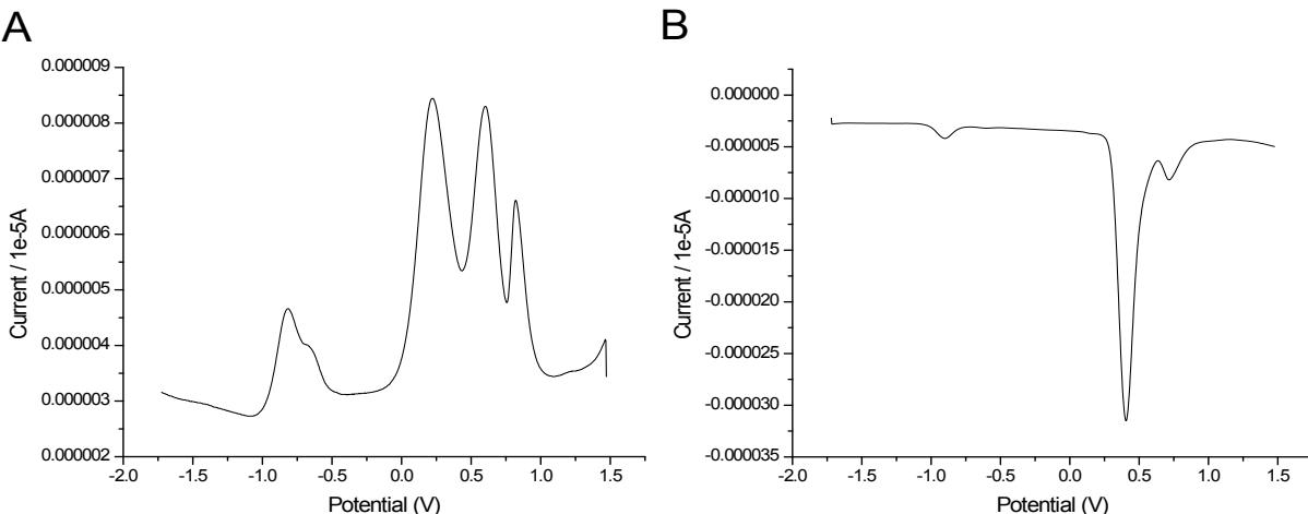
**Fig. S22.** Differential pulse voltammograms of ebit (10 mM) in acetonitrile: A) negative mode and B) positive mode; potentials are reported vs. NHE.
