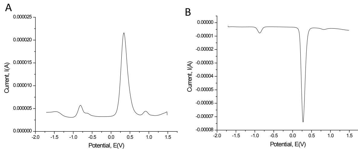
**Fig. S21.** Differential pulse voltammograms of dmise (10 mM) in acetonitrile: A) negative mode and B) positive mode; potentials are reported vs. NHE.
