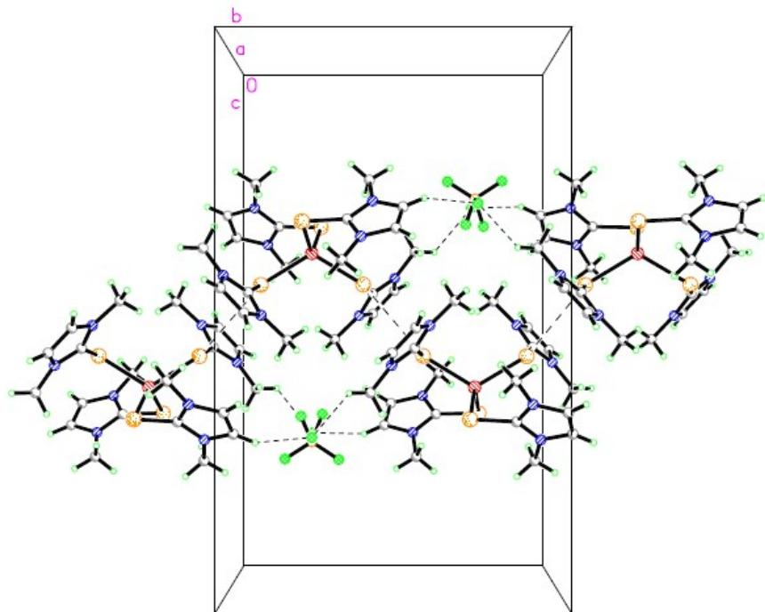
**Fig. S4.** Crystal packing diagram for  $[\text{Fe}(\text{dmise})_4][\text{BF}_4]_2$  (**6b**) showing short F-H interactions as viewed along the *a*-axis with 50% probability density ellipsoids.
