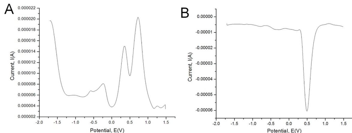
**Fig. S28.** Differential pulse voltammograms of  $[\text{Fe}(\text{dmit})_4]\text{[OTf]}_2$  (**5a**; 10 mM) in acetonitrile: A) negative mode and B) positive mode; potentials are reported vs. NHE.
