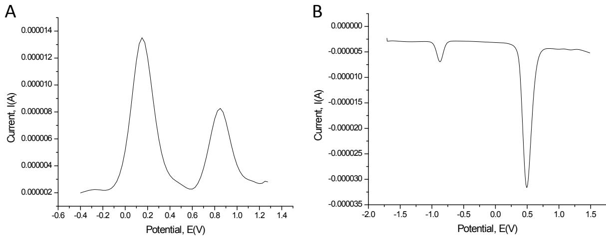
**Fig. S20.** Differential pulse voltammograms of dmit (10 mM) in acetonitrile: A) negative mode and B) positive mode; potentials are reported vs. NHE.
