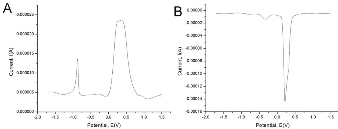
**Fig. S29.** Differential pulse voltammograms of  $[\text{Fe}(\text{dmise})_4]\text{[OTf]}_2$  (**6a**; 10 mM) in acetonitrile: A) negative mode and B) positive mode; potentials are reported vs. NHE.
