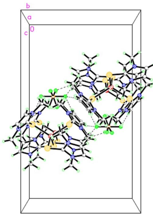
**Fig. S3.** Crystal packing diagram for  $[\text{Fe}(\text{dmit})_4][\text{BF}_4]_2$  (**5b**) showing short F-H interactions as viewed along the *a*-axis with 50% probability density ellipsoids
