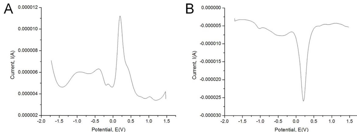
**Fig. S31.** Differential pulse voltammograms of  $\{\text{Fe}(\text{ebis})\text{Cl}_2\}_n$  (**8**; 10 mM) in acetonitrile: A) negative mode and B) positive mode; potentials are reported vs. NHE.
