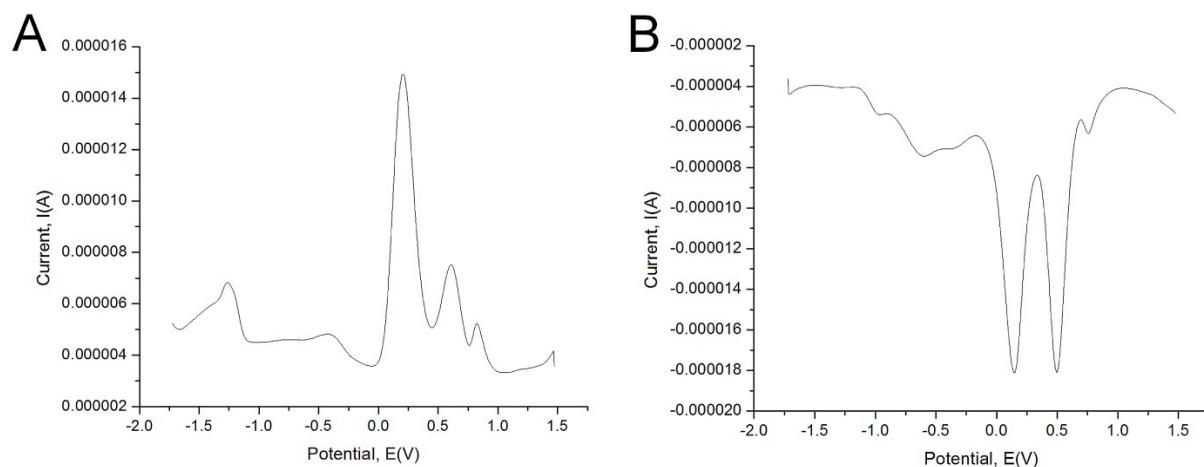
**Fig. S30.** Differential pulse voltammograms of  $\{\text{Fe}(\text{ebit})\text{Cl}_2\}_n$  (**7**; 10 mM) in acetonitrile: A) negative mode and B) positive mode; potentials are reported vs. NHE.
