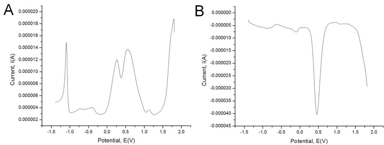
**Fig. S26.** Differential pulse voltammograms of  $[\text{Fe}(\text{dmit})_2(\text{CH}_3\text{CN})_2]\text{[OTf]}_2$  (**3**; 10 mM) in acetonitrile: A) negative mode and B) positive mode; potentials are reported vs. NHE.
