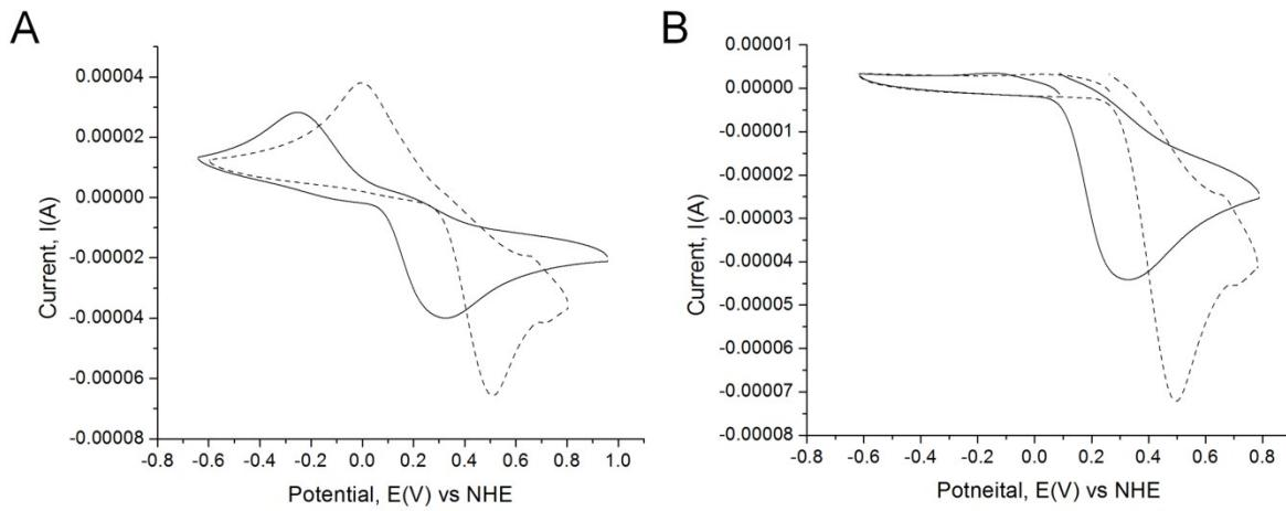
**Fig. S16.** Cyclic voltammetry with initial starting potential at A) 0.94 V for ebis (solid) and 0.80 V for ebit (dashed) and B) 0.09 V for ebis (solid) and 0.26 V for ebit (dashed).
